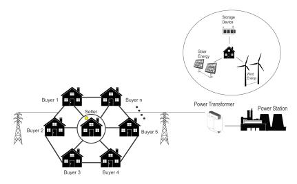
Figure 1.2: Smart grid network with peer-to-peer energy trading
