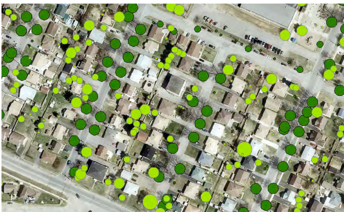
Figure 4.5. A screenshot from ArcGIS displaying the public (dark green) and private (light green) trees after the buffers had been applied, to produce a realistic representation of canopy cover based on each tree's crown width class.
