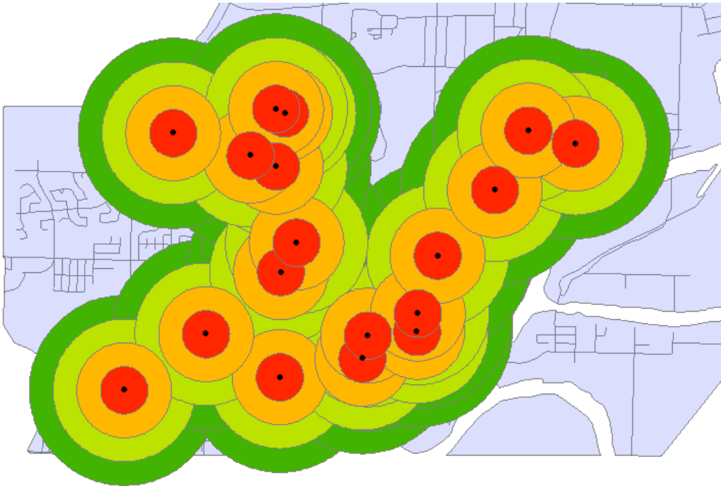
Figure 5.12. A screenshot of the various multiple ring buffers surrounding schools for a portion of Thunder Bay schools. The schools are represented by black dots, the red buffers are the 250m zones (weight of 1), the orange buffers are the 500m zones (weight of .75), the light green buffers are the 750m zones (weight of .50), and the dark green are the 1000m zones (weight of .25).
