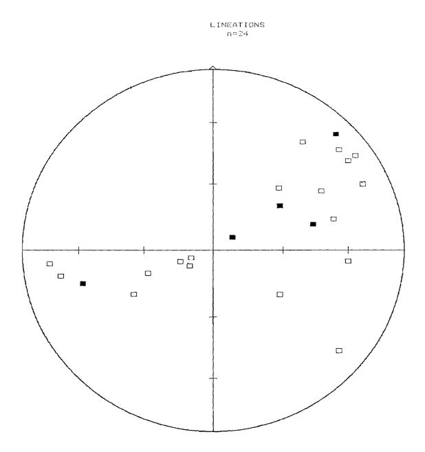
squares. The distribution of hinge lines appears to lie in the general plane of the foliation. The wide variation in plunge of the hinge lines from very steep to very gentle may be due to refolding of earlier folds or sheath folding.
