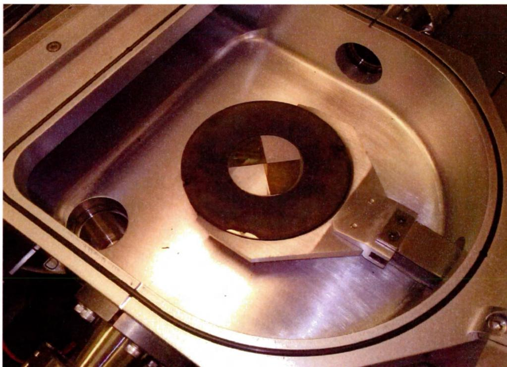
*Figure 4.3: The placement of the sapphire substrates (clear  $\frac{1}{4}$  wafer sections) in proximity to the surrounding aluminum disk and extra sapphire covers (discarded GaN samples, dark  $\frac{1}{4}$  wafer sections). The configuration is expected to act to lower temperature and prevent atomic deposition from the sample holder.*
