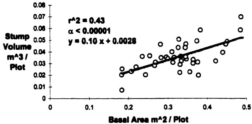
Figure 19. Regression of measured basal area per plot versus measured stump volume per plot for the CTL system.
