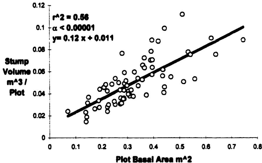
Figure 15. Regression of measured basal area per plot versus measured stump volume per plot for the FT-CH system.
