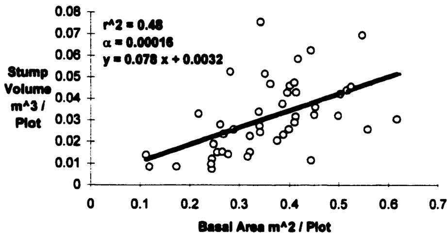
Figure 17. Regression of measured basal area per plot versus measured stump volume per plot for the FT-SW harvesting system.
