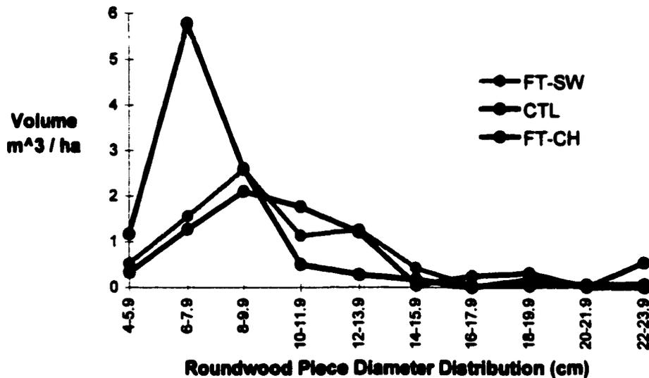
Figure 23. Volume of roundwood pieces distributed by 2 cm diameter class for the FT-SW, CTL and FT-CH systems.
