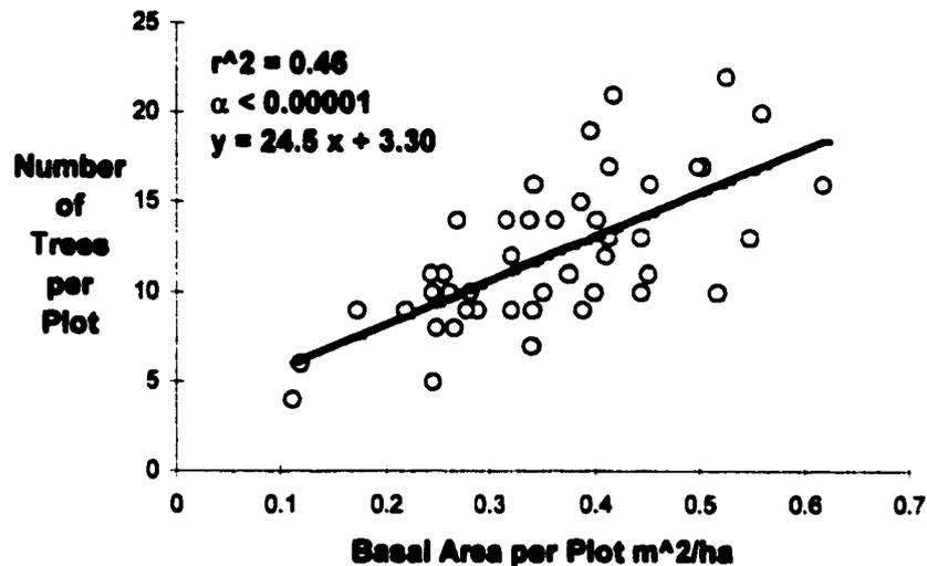
Figure 21. Regression of basal area per plot and number of trees per plot for the tree-length-to-mill system.
