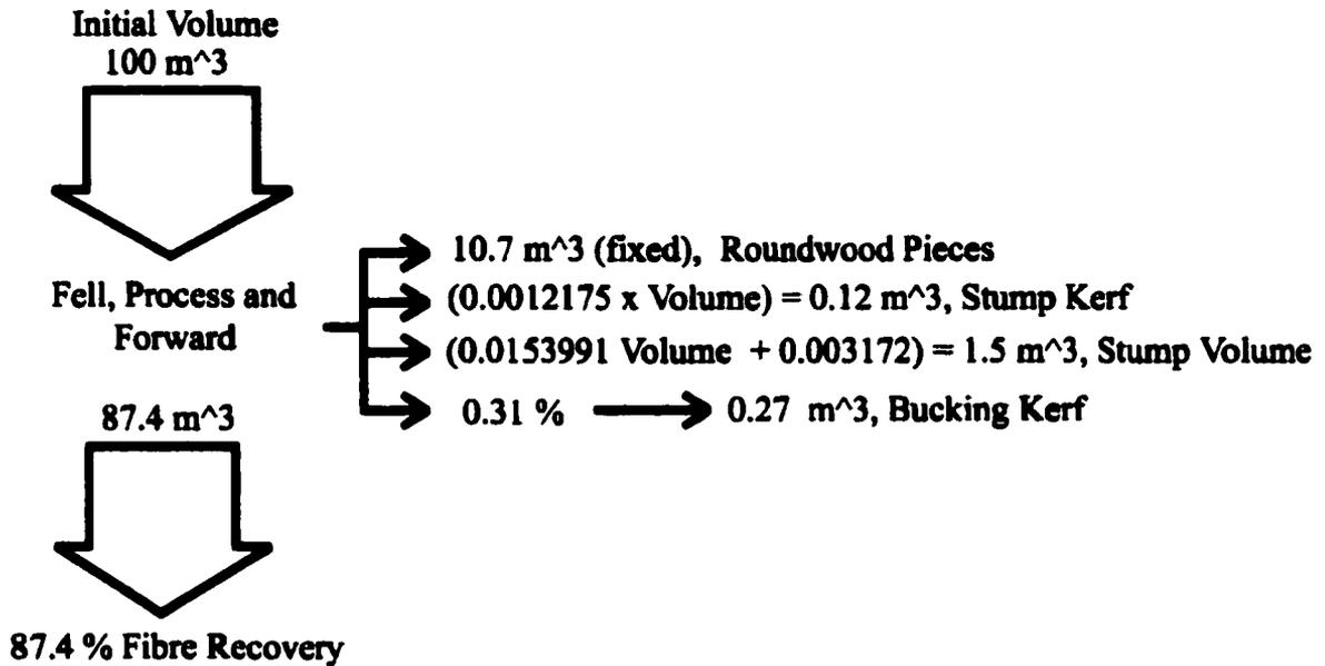
**Figure 18. Wood fibre utilization model for the CTL (single-grip harvester/forwarder) system. Descending arrows are to scale and indicate wood flow towards the mill. Horizontal arrows indicate fibre losses. The initial volume of 100 m<sup>3</sup>/ha is used as an arbitrary seed value.**
