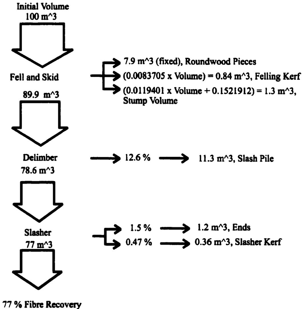
Figure 16. Wood fibre utilization model for the FT-SW (feller-buncher/skidder/delimber/slasher) system. Descending arrows are to scale and indicate wood flow towards the mill. Horizontal arrows indicate fibre losses. The initial volume of 100 m<sup>3</sup>/ha is used as an arbitrary seed value.
