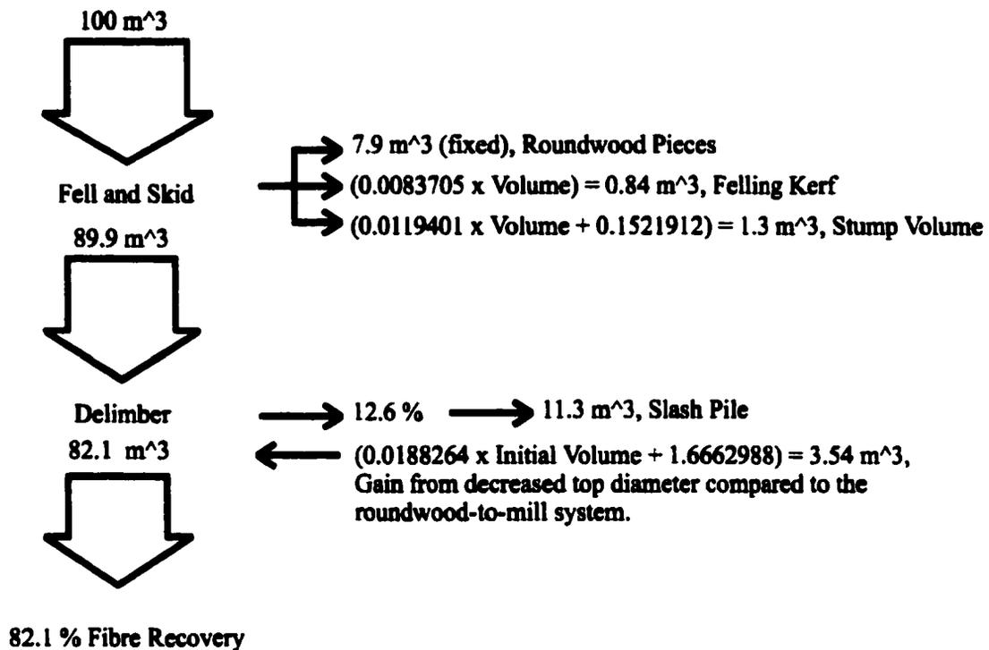
Figure 20. Wood fibre utilization model for the FT-TL (feller-buncher/skidder/delimiter) system. Descending arrows are to scale and indicate wood flow towards the mill. Horizontal arrows indicate fibre losses. The initial volume of 100 m<sup>3</sup>/ha is used as an arbitrary seed value.
