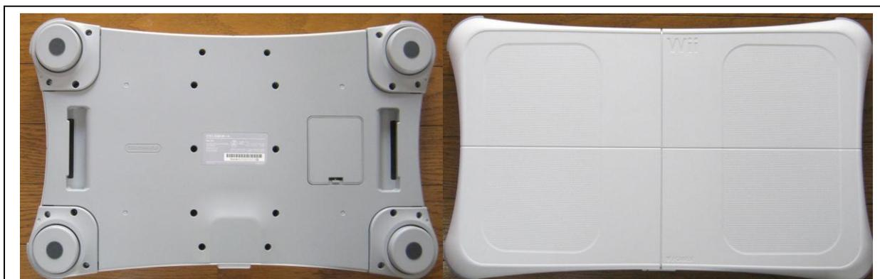
*Figure 21.* Wii board. The board on the left illustrates that the four sensors are in the corners of the board. The board on the right shows the rectangles where the individual should stand while performing simulations. Adapted from “About the Wii console” by Nintendo, 2010. Copyright 2010 by author, Canada.
