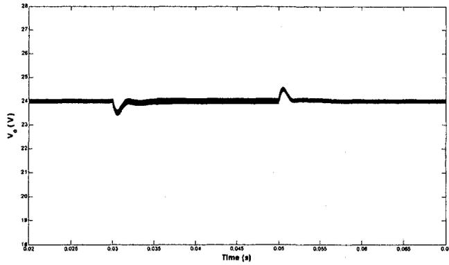
Figure 3-2: Output voltage performance for load disturbance,  $\pm 17\Omega$
