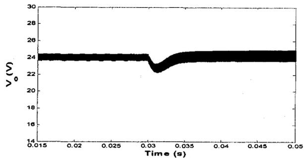
Figure 3-11: Output voltage response to input voltage disturbance of  $-1.85V$ ,  $D < D_{max}$
