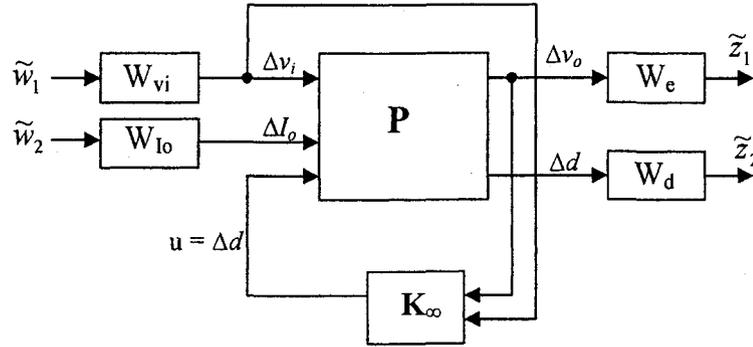
Figure 2-2: Block diagram used to design  $H_\infty$  controller
