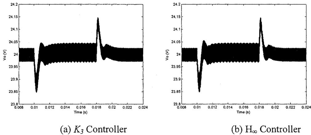
Figure 2-13: Simulated output behavior for line voltage disturbance
