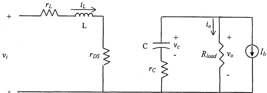
(a) Switch ON; Diode OFF
