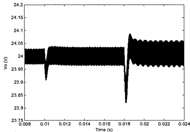
Figure 2-22:  $v_o$  performance of the worst case stability for system controlled by  $K_I$ ,
