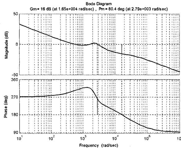
Figure 3-14: Frequency of the designed controlled system loop gain
