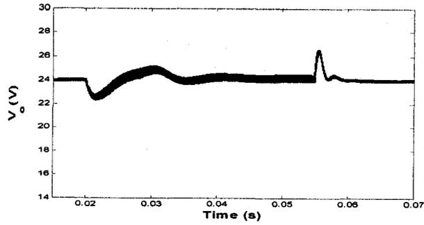
Figure 3-10: Output voltage response (avoiding dynamic collapse of Figure 3-4,  $D_{sat}=0.8736$ )
