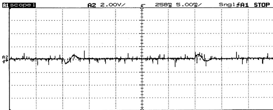
Figure 4-18: Amplified negative error voltage measured at the input of the controller
