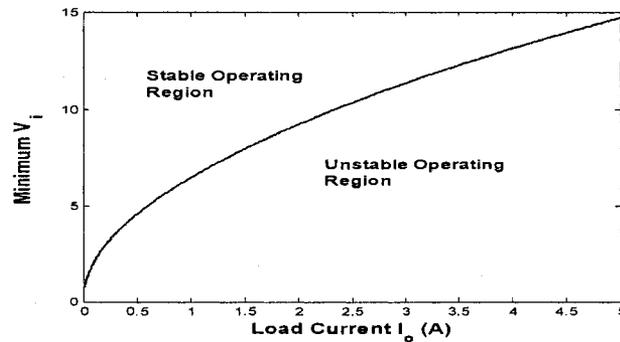
Figure 3-7: Minimum line input voltage required to avoid static output voltage collapse
