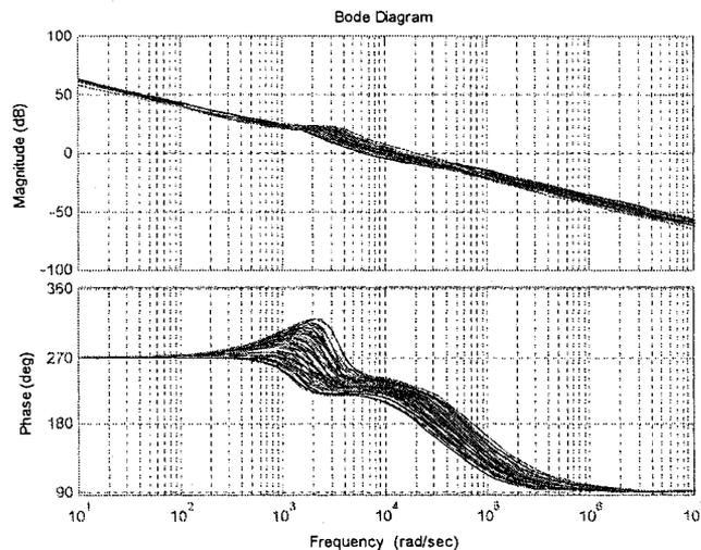
Figure 2-18: Frequency responses of the uncertain systems (controlled by  $K_I$ ) subsequent to the parameters variations and disturbances (nominal and limit values)
