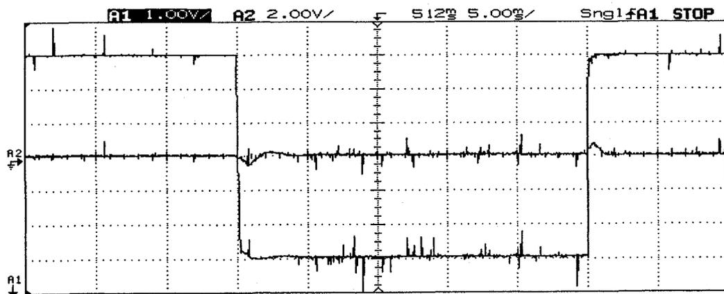
Figure 4-13: Amplified negative error voltage measured at the input of the controller
