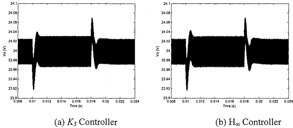
Figure 2-12: Simulated output behavior for load disturbance
