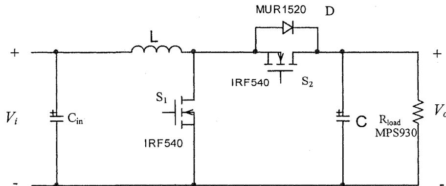
Figure 4-1: Synchronous Boost Converter used in the experimental setup
