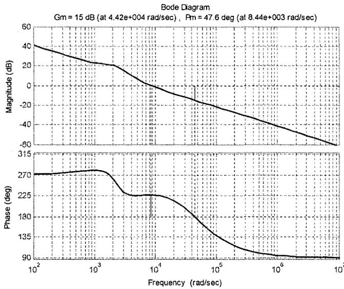
Figure 2-4: Loop gain frequency response using  $H_\infty$  controller
