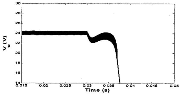
Figure 3-12: Output voltage response to input voltage disturbance of  $-2V$ ,  $D > D_{max}$
