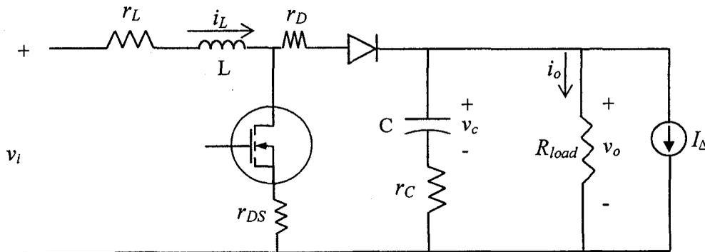
Figure 1-1: Boost converter circuit
