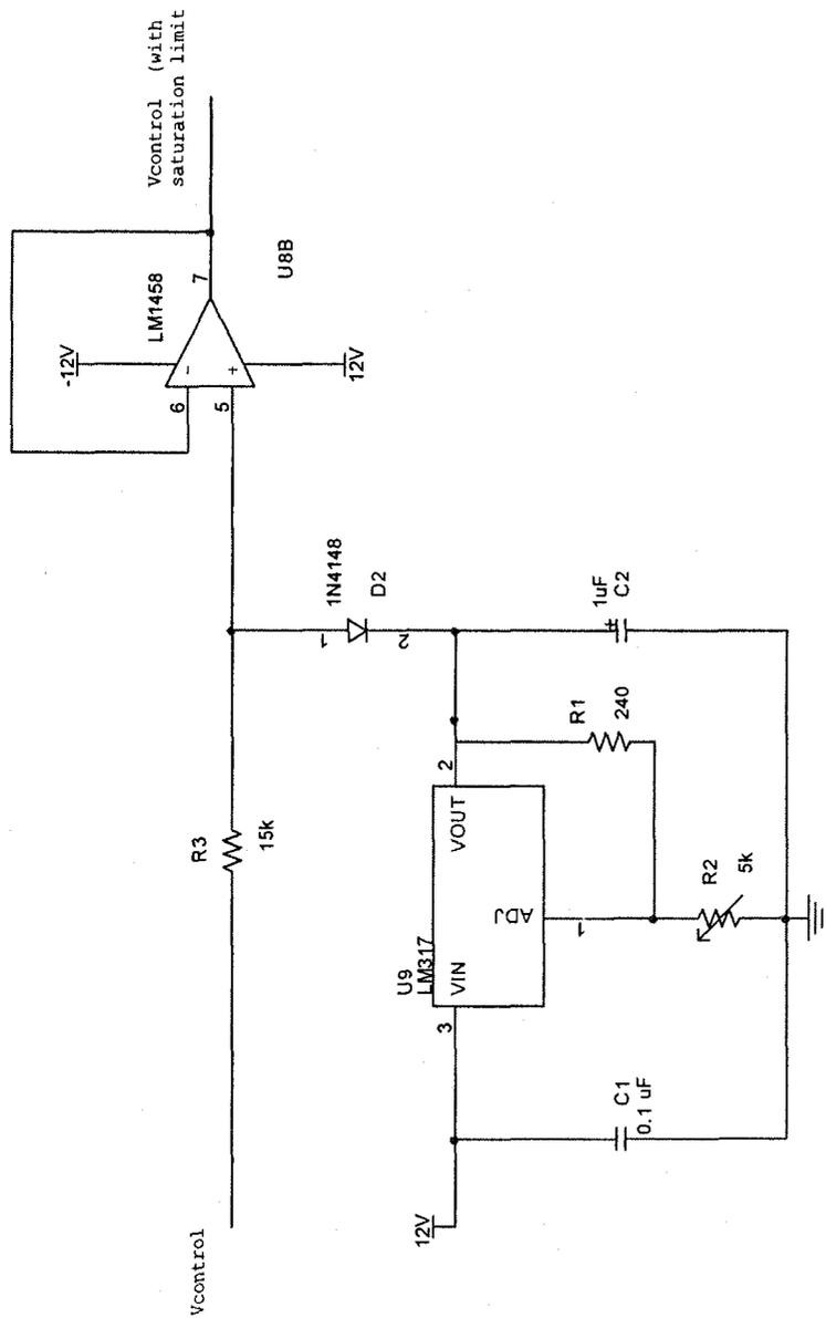
Figure A-3: Duty cycle saturating circuit
