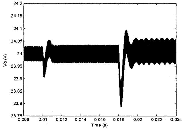
Figure 2-23:  $v_o$  performance of the worst case stability for system controlled by  $K_3$ ,
