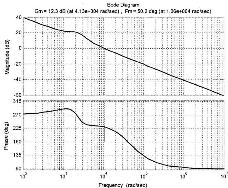
Figure 2-9: Loop gain frequency response of the  $G_{c1}$  controlled system
