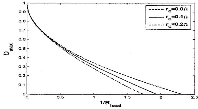
Figure 3-5: Stable duty cycle limit  $D_{max}$  versus  $1/R_{load}$
