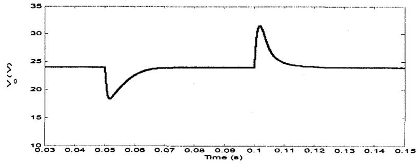
(a) Passivity Based Controller
