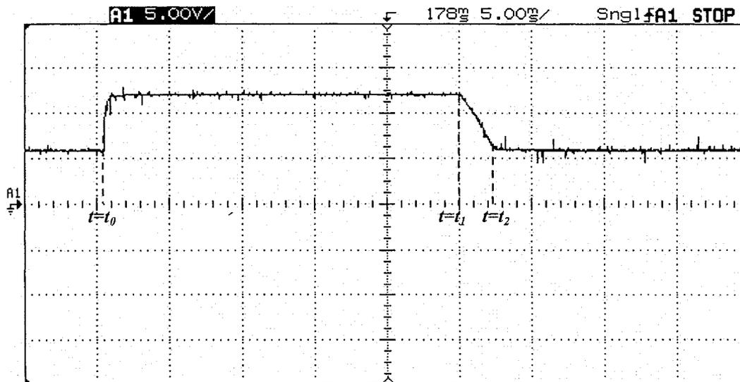
Figure 4-11:  $V_s$  performance with  $C_{in}=470\mu\text{F}$
