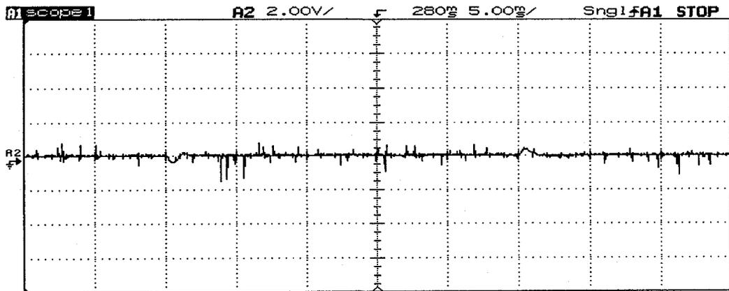
Figure 4-7: Amplified negative error voltage measured at the input of the controller
