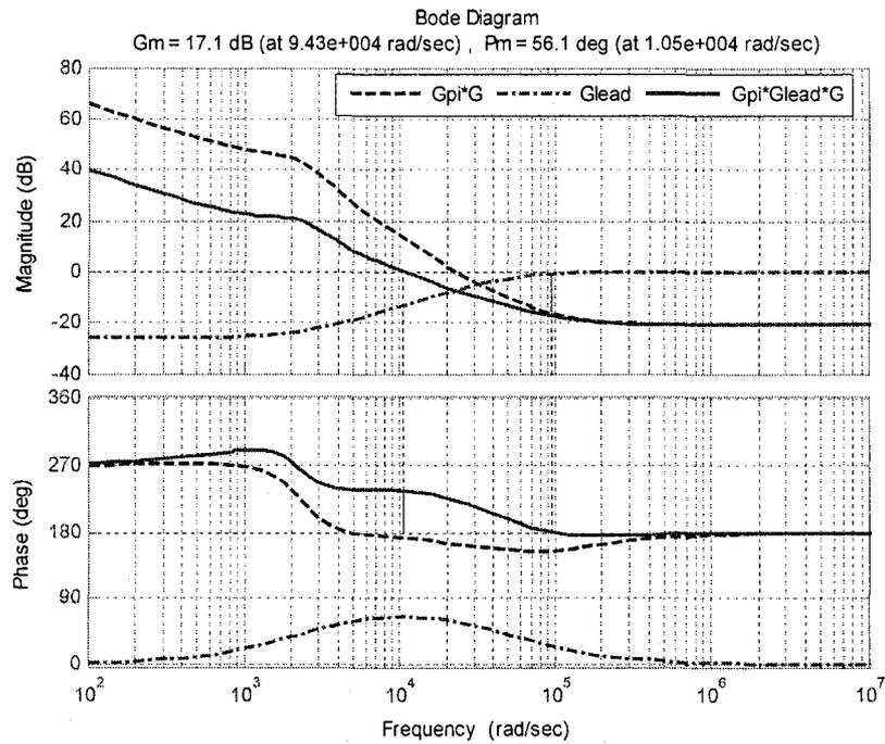
Figure 2-8: Frequency response of  $G_{pi}G$ ,  $G_{lead}$ ,  $G_{pi}G_{lead}G$
