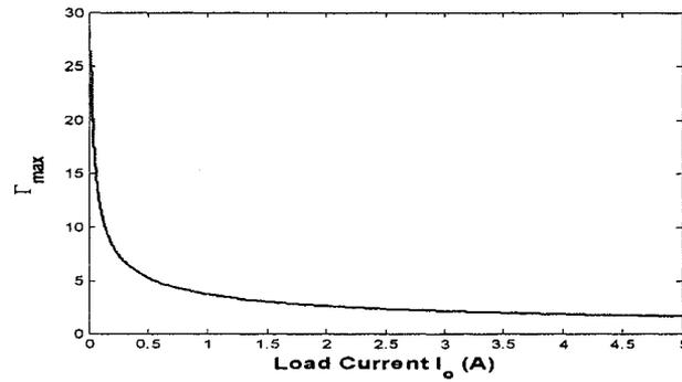
Figure 3-6: Maximum boosting gain as a function of load current
