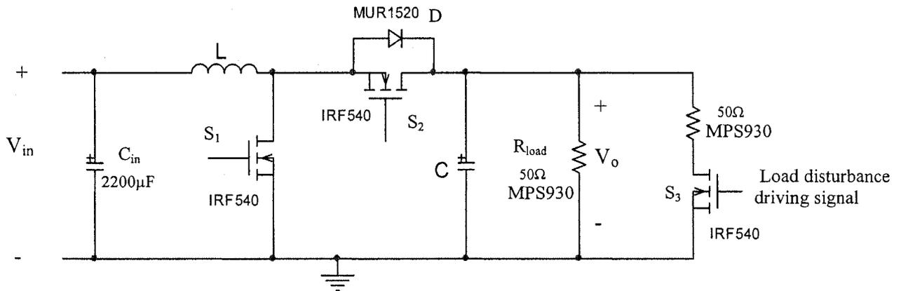
Figure 4-5: Load disturbance experimental setup
