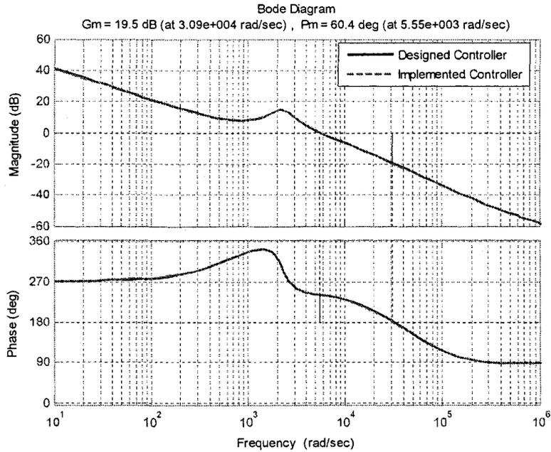
Figure 4-4: Loop gain frequency response using the theoretically designed controller and the experimentally implemented controller
