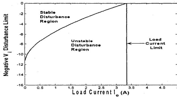
Figure 3-8: Negative  $V_i$  disturbance limit and load current limit
