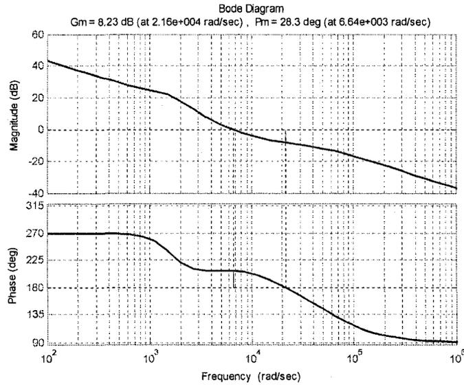
Figure 2-21: Worst case stability margins for  $H_\infty$  controlled system
