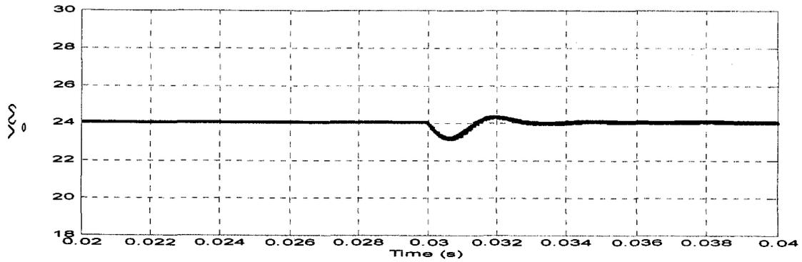
(a) Simulated output performance for positive 100% load disturbance ( $V_i=6V$ )
