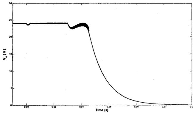
Figure 3-3: Output voltage performance for load disturbance and input voltage disturbance leading to voltage collapse
