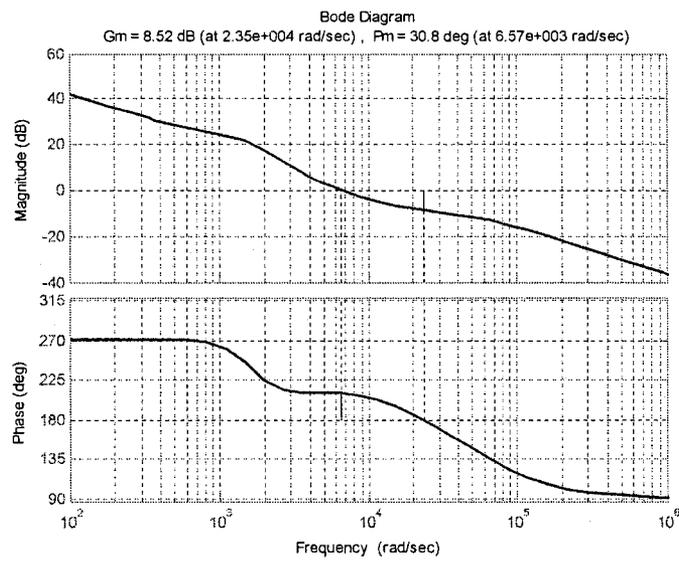
Figure 2-20: Worst case stability margins for  $K_3$  controlled system
