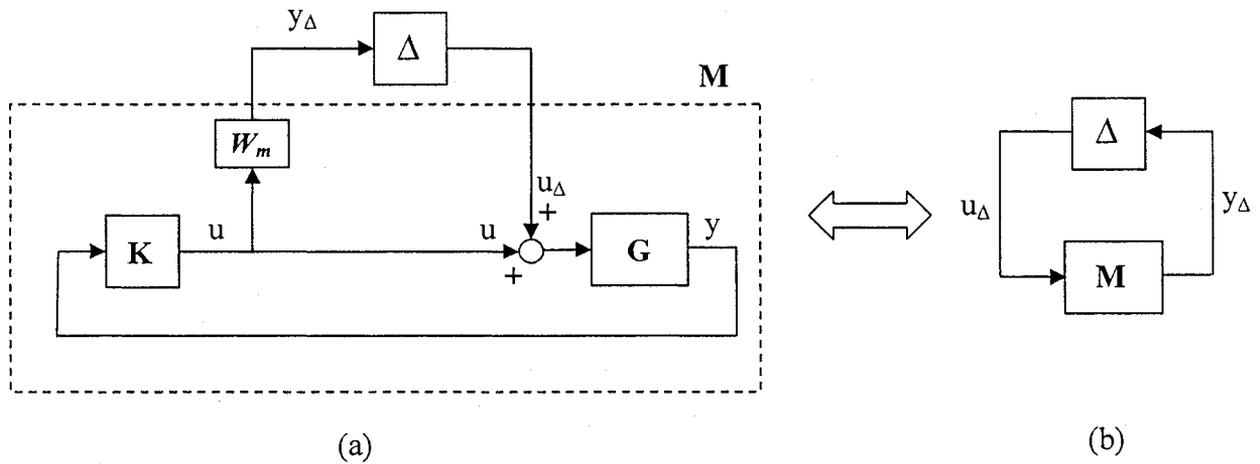
Figure 2-25: Block diagram of the boost converter system in the presence of multiplicative input uncertainty
