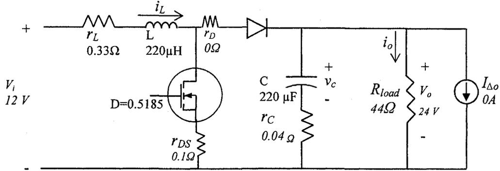
Figure 2-1: Boost converter circuit operating at 100 KHz
