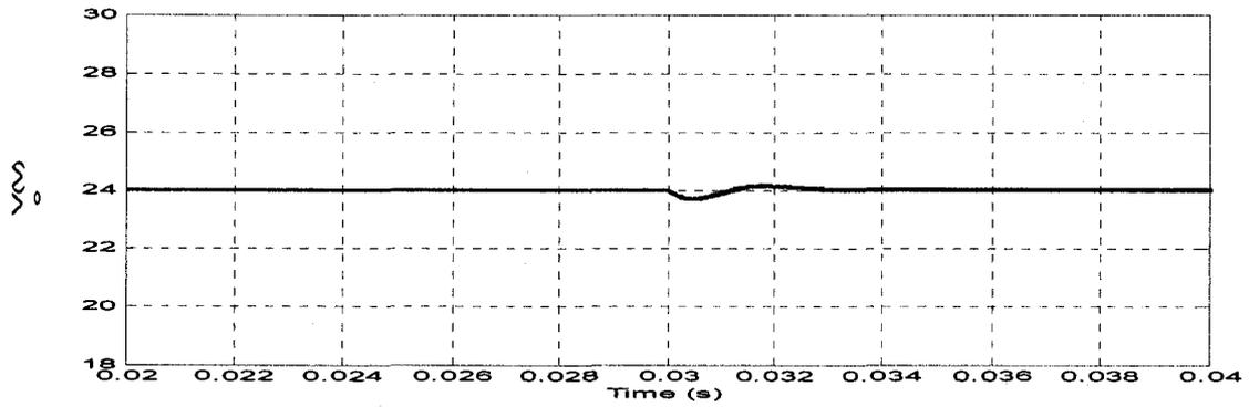
(a) Simulated output performance for negative line voltage disturbance
