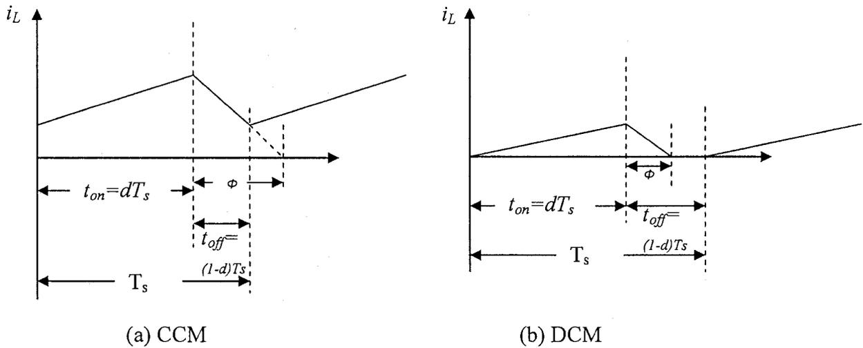
Figure 1-3: Inductor Current and  $i_L$  and  $\phi$  in continuous (a) and discontinuous (b) conduction mode
