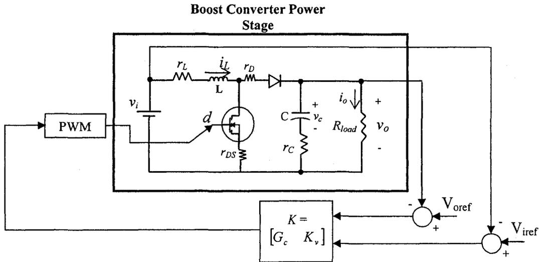
Figure 2-6: Controller diagram of the boost converter
