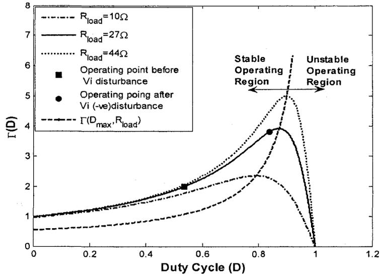
Figure 3-4: Static characteristic of the boost converter (Illustrative Example)
