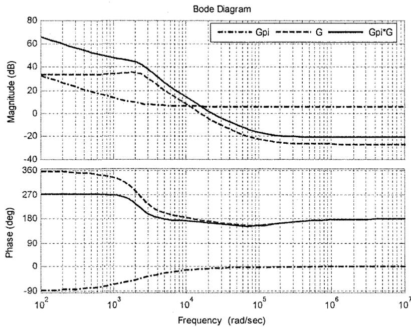
Figure 2-7: Frequency response of  $G$ ,  $G_{pi}$  and  $G_{pi}G$
