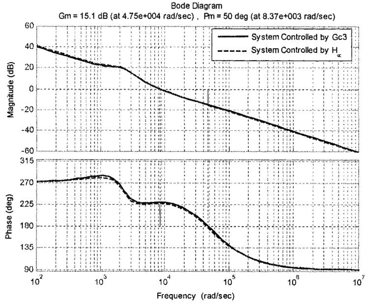
Figure 2-11: Loop gain frequency response of  $H_\infty$  controlled system and  $G_{c3}$  controlled system
