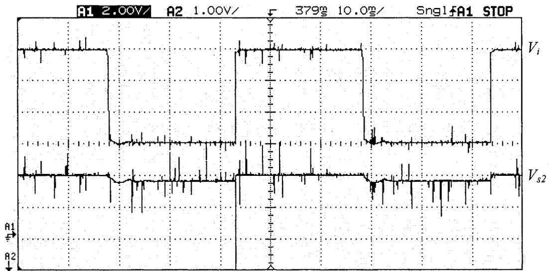
Figure 4-15:  $V_{s2}$  dynamic response and  $V_i$  waveform
