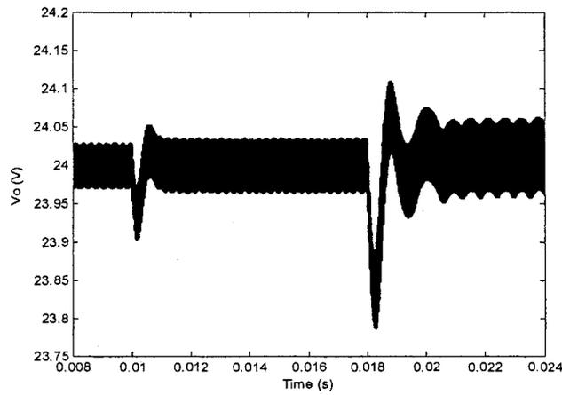
Figure 2-24:  $v_o$  performance of the worst case stability for system controlled by  $H_\infty$ ,
