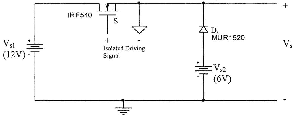
Figure 4-9: Circuit setup used to apply voltage disturbances
