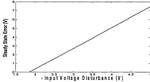
Figure 3-9: Steady state error with  $D_{sat}=D_{max}=0.7916$  ( $R_{load}=10\Omega$ )
