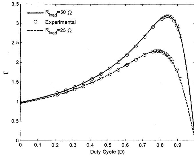
Figure 4-2: Experimentally measured static characteristics vs. the calculated characteristics (with an additional input series resistance of  $1 \Omega$ )
