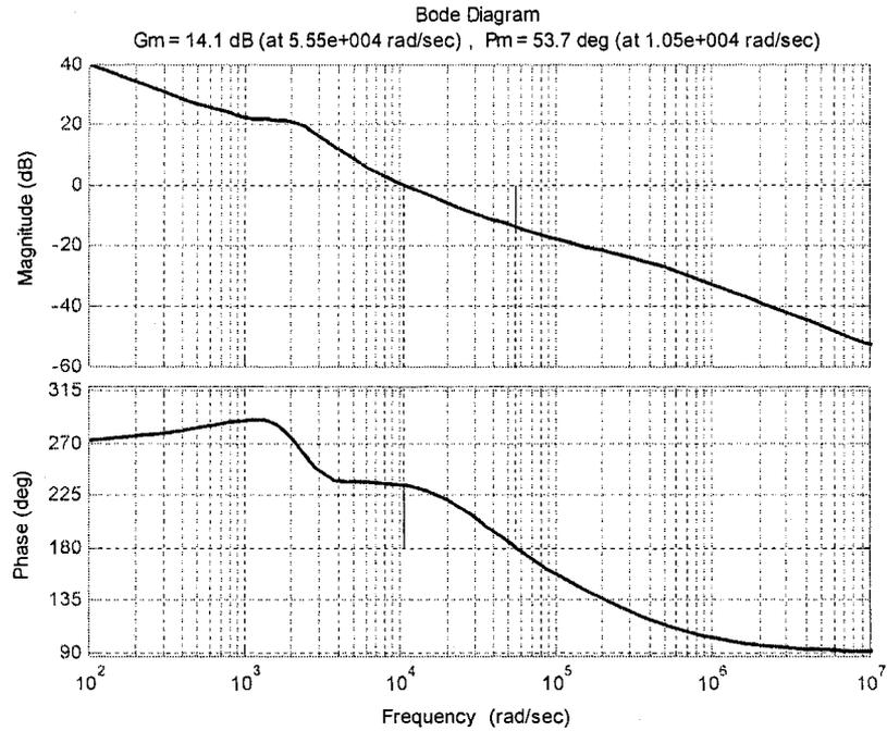
Figure 2-10: Loop gain frequency response in the  $G_{c2}$  controlled system
