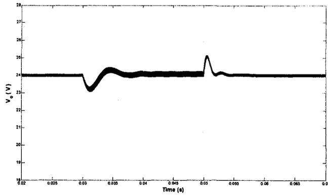
Figure 3-1: Output voltage performance for line disturbance,  $\pm 6V$
