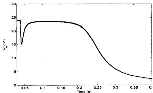
Figure 3-17:  $V_o$  performance for -5 line voltage disturbance (Static voltage collapse)
