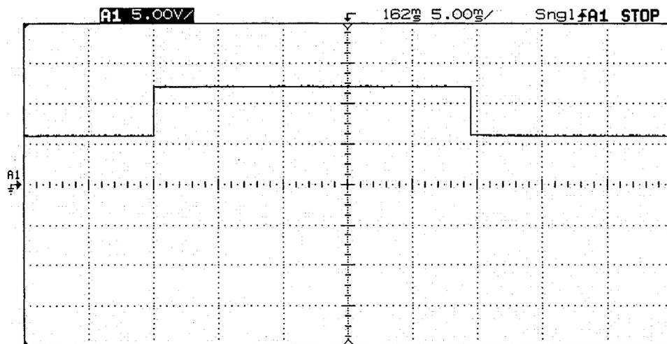
Figure 4-10: Output voltage ( $V_s$ ) with a low resistive load
