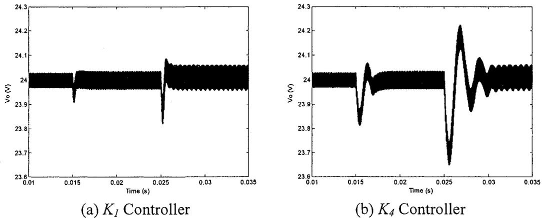
Figure 2-28: Output voltage performance of the worst case stability
