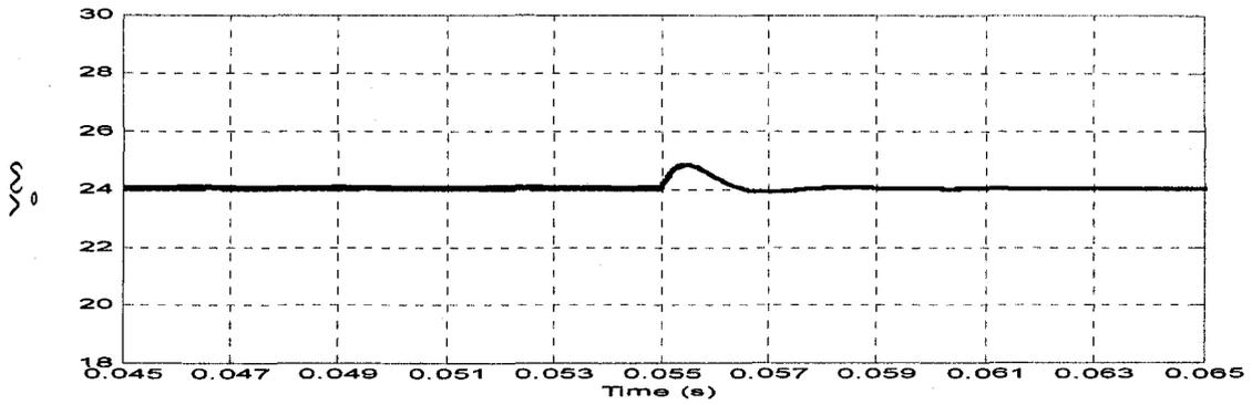
(c) Simulated output performance for 100% negative load disturbance ( $V_i=6V$ )
