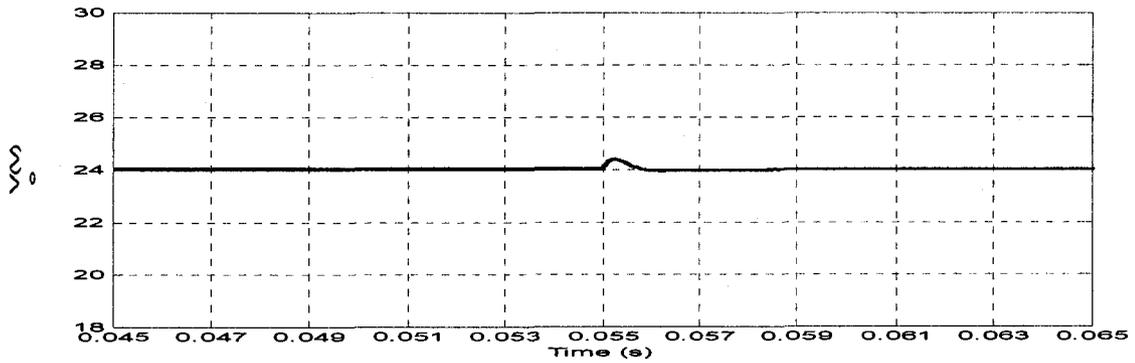
(c) Simulated output performance for positive line voltage disturbance
