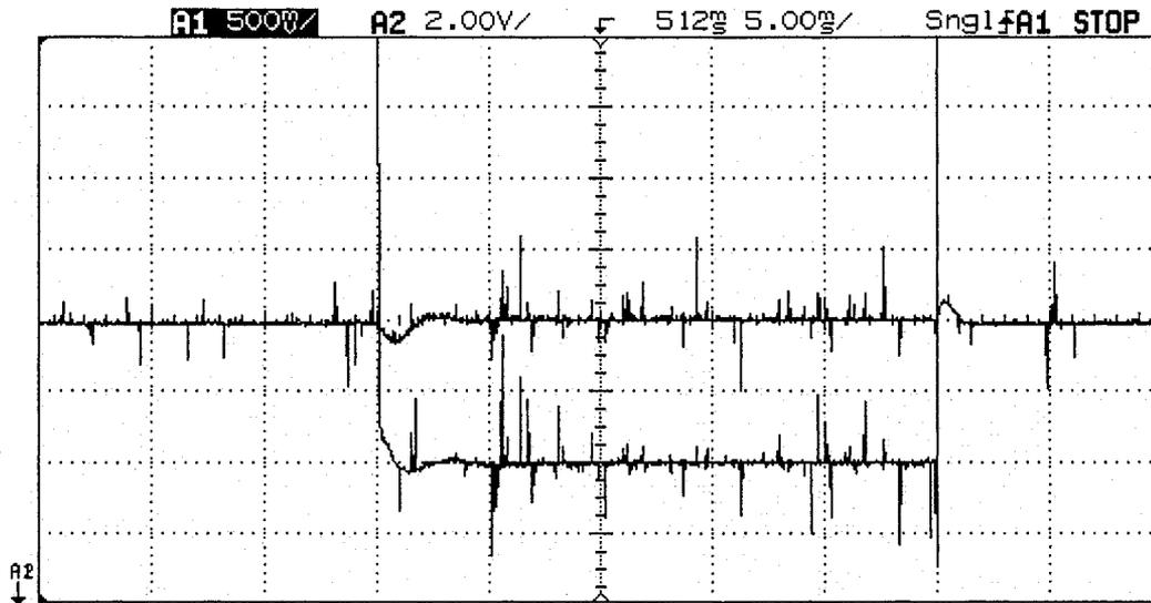
Figure 4-14:  $V_i$  Falling edge along with the output voltage performance
