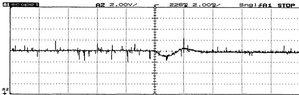
(b) Experimental output performance for positive 100% load disturbance ( $V_i=6V$ )
