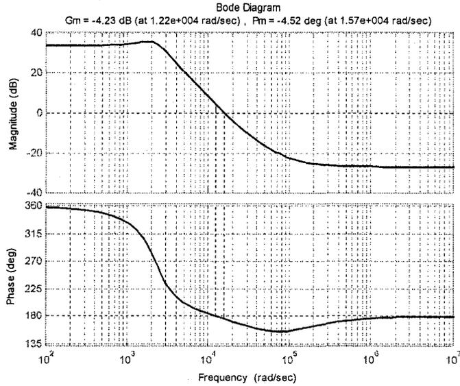
Figure 2-3: Frequency response of control-to-output transfer function
