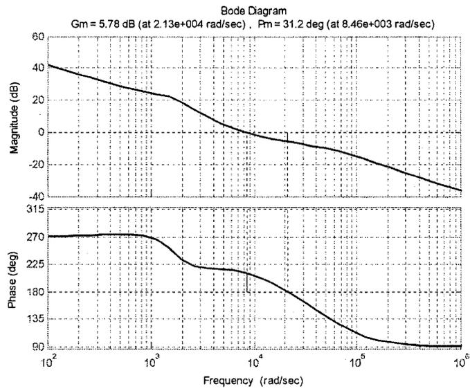
Figure 2-19: Worst case stability margins for  $K_1$  controlled system
