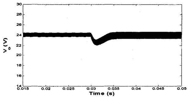
Figure 3-13: Output voltage response to input voltage disturbance of  $-2V$ , ( $D > D_{max}$  with  $D_{sat} = D_{max}$ )
