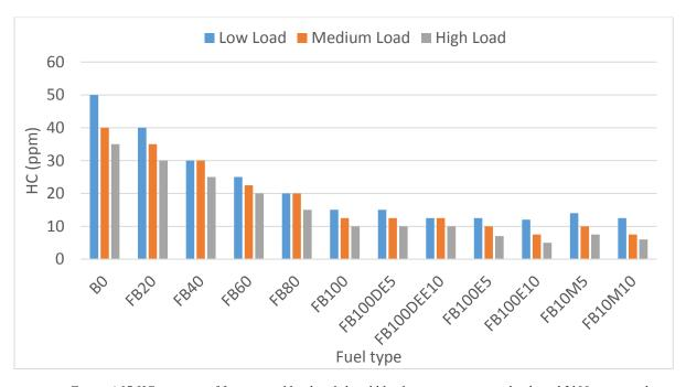
Figure 4.17 HC emission of fractionated biodiesel-diesel blends at various engine loads and 2100 rpm speed
