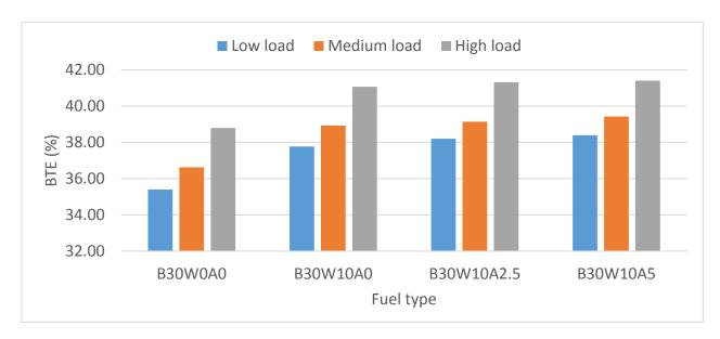
Figure 4.14 BTE of B30 with three different ammonium hydroxide levels in emulsion with water content of 10% at various engine loads and 2100 rpm speed.
