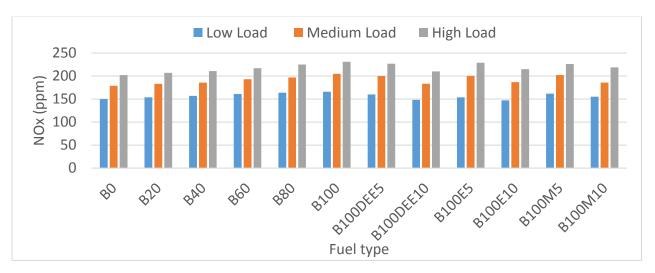
Figure 4.10 NOx emission of biodiesel-diesel blends at various engine loads and 2100 rpm speed
