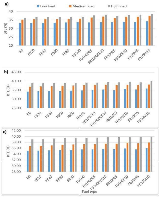
Figure 4.9 BTE of different fractionated biodiesel blends at various engine loads at a) 1000 rpm, b) 2100 rpm and c) 3000 rpm
