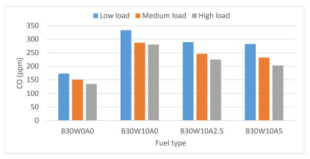
Figure 4.26 CO emission of B30 with three different ammonium hydroxide levels in emulsion with water content of 10% at various engine loads and 2100 rpm speed
