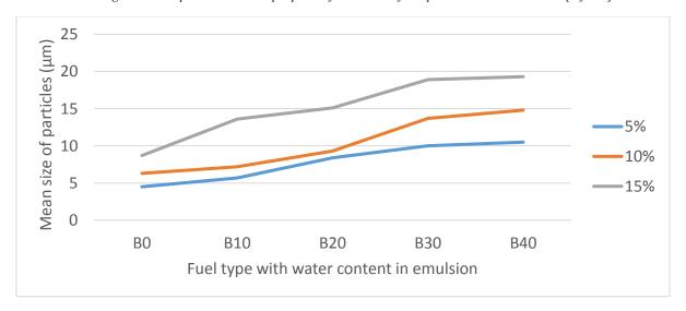
Figure 4.3 Mean particle size of emulsion diesel-blends with three water levels [ref.102]
