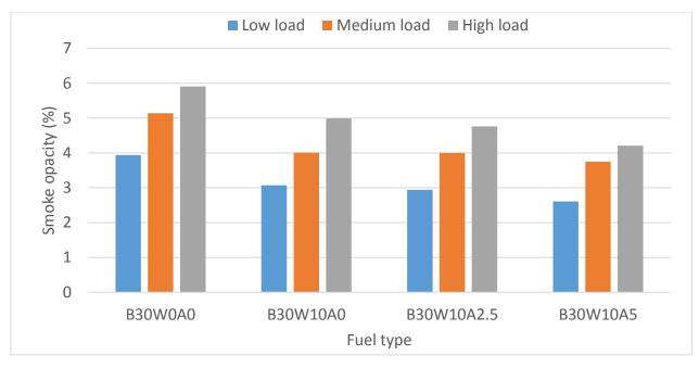
Figure 4.23 Smoke opacity of B30 with three different ammonium hydroxide levels in emulsion with water content of 10% at various engine loads and 2100 rpm speed
