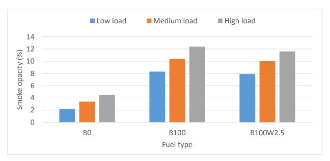
Figure 4.22 Smoke opacity of biodiesel and biodiesel emulsion at various engine loads and 2100 rpm speed
