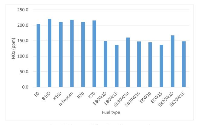
Figure 4.30 NOx emission of different fuel at 1500 rpm engine speed
