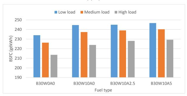
Figure 4.7 BSFC of B30 with three different ammonium hydroxide levels in emulsion with water content of 10% at various engine loads at 2100 rpm speed
