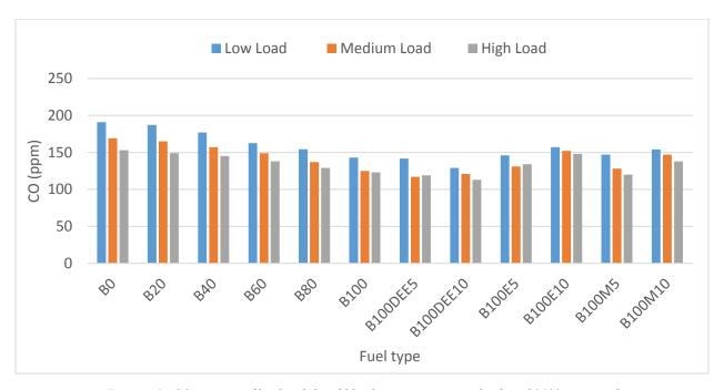
Figure 4.14 CO emission of biodiesel-diesel blends at various engine loads and 2100 rpm speed
