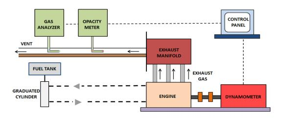
Figure 3.7 Schematic diagram of the light-duty diesel engine setup
