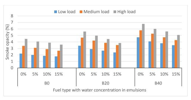
Figure 4.21 Smoke opacity of diesel and diesel-biodiesel blends with their emulsions at various engine loads and 2100 rpm speed [ref. 102]
