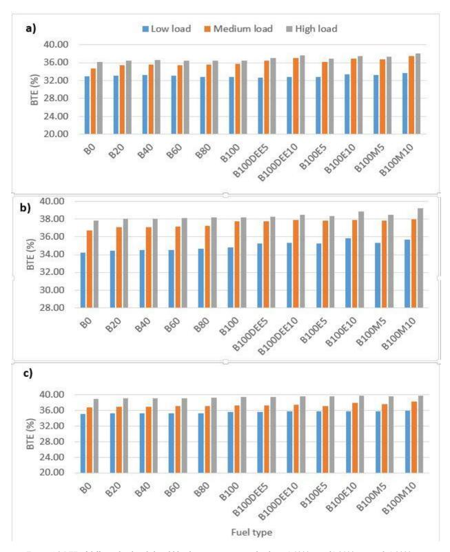
Figure 4.8 BTE of different biodiesel-diesel blends at various engine loads at a) 1000 rpm, b) 2100 rpm and c) 3000 rpm
