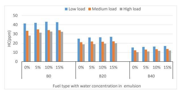
Figure 4.27 HC emission of diesel and diesel-biodiesel blends with their emulsions at various engine loads and 2100 rpm speed [ref.102]
