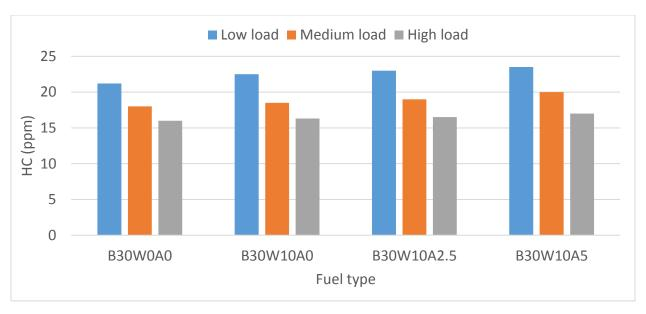
Figure 4.29 HC emission of B30 with three different ammonium hydroxide levels in emulsion with water content of 10% at various engine loads and 2100 rpm speed.
