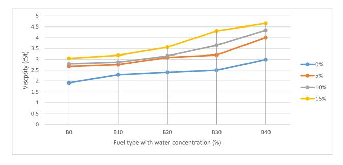
Figure 4.4 Viscosity of different fuels vs water concentration [ref.102]
