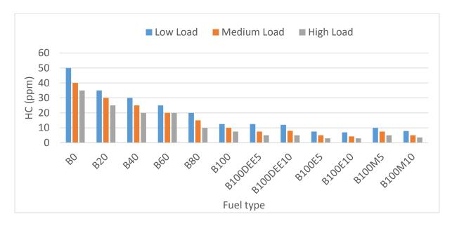
Figure 4.16 HC emission of biodiesel-diesel blends at various engine loads and 2100 rpm speed
