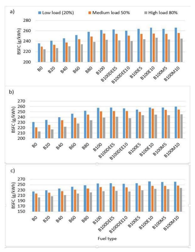
Figure 4.6 BSFC of different biodiesel-diesel blends at various engine loads at a) 1000 rpm, b) 2100 rpm and c) 3000 rpm
