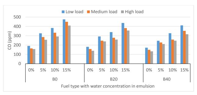
Figure 4.24 CO emission of diesel and diesel-biodiesel blends with their emulsions at various engine loads and 2100 rpm speed [ref.102]
