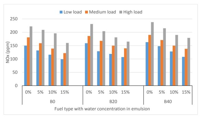
Figure 4.18 NOx emission of biodiesel-diesel blends and their emulsions at various engine loads and 2100 rpm speed [ref.102]
