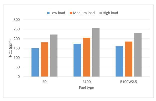
Figure 4.20 NOx emission of B0, B100 and B100W2.5 at various engine loads and 2100 rpm speed
