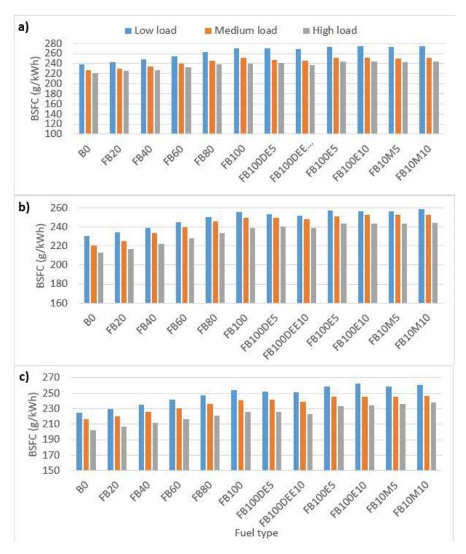
Figure 4.7 BSFC of different fractionated biodiesel blends at various engine loads at a) 1000 rpm, b) 2100 rpm and c) 3000 rpm
