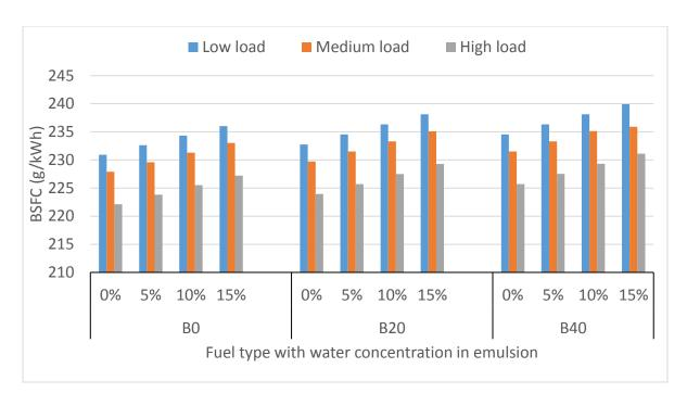
Figure 4.10 BSFC of different fuel blends with three different water levels in emulsion at various engine loads at 2100 rpm speed [ref.102]
