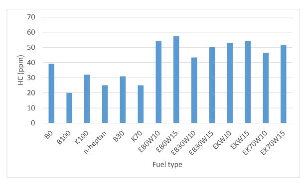
Figure 4.32 HC emission of various fuel at 1500 engine speed
