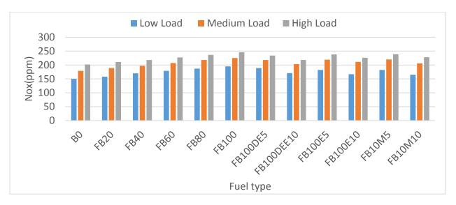
Figure 4.11 NOx emission of fractionated biodiesel-diesel blends at various engine loads and 2100 rpm speed
