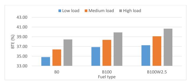
Figure 4.15 BTE of B0, B100 and B100W2.5 at various engine loads and 2100 rpm speed
