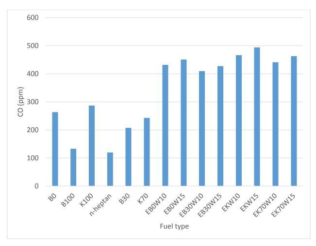
Figure 4.31 CO emission of various fuels at 1500rpm engine speed
