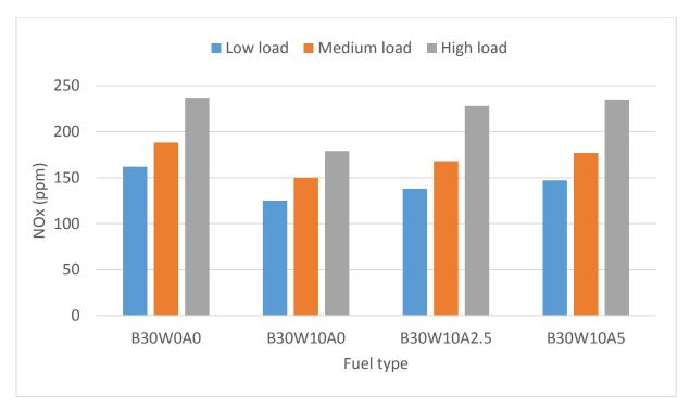
Figure 4.19 NOx emission of B30 with three different ammonium hydroxide levels in emulsion with water content of 10% at various engine loads and 2100 rpm speed.
