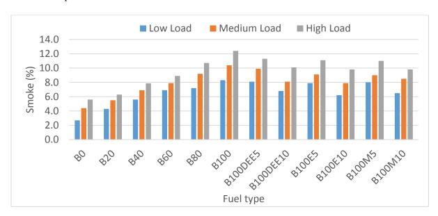
Figure 4.12 Smoke opacity of biodiesel blends at various engine loads and 2100 rpm speed.
