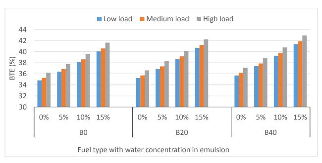
Figure 4.9 BTE of different fuels and their emulsions at various engine loads and 2100 rpm speed [ref.102]
