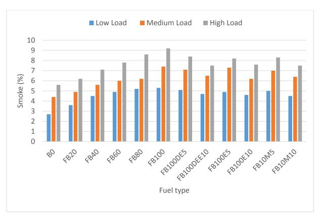
Figure 4.13 Smoke opacity of fractionated biodiesel blends at various engine loads and 2100 rpm speed
