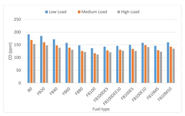
Figure 4.15 Fractionated biodiesel blends at various engine loads and 2100 rpm speed.
