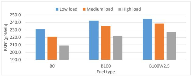
Figure 4.8 BSFC of B0, B100 and B100W2.5 at various engine loads and 2100 rpm speed.
