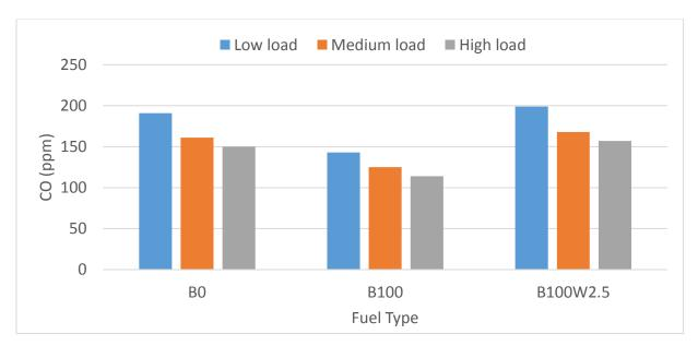
Figure 4.25 CO emission of biodiesel and biodiesel emulsion at various engine loads and 2100 rpm speed
