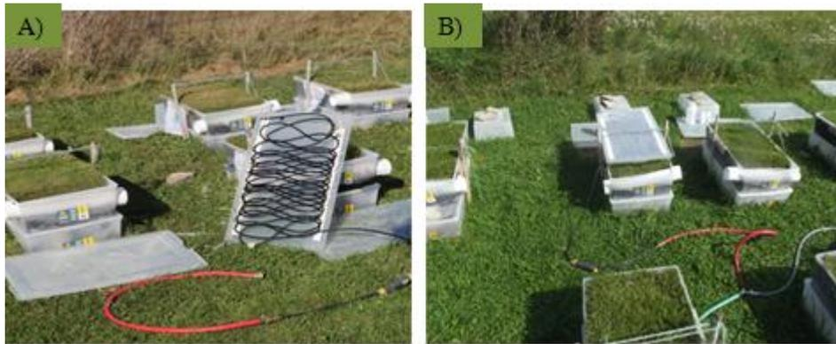
**Figure 5.** The rain simulator used for the experiment (A) and in use (B).
