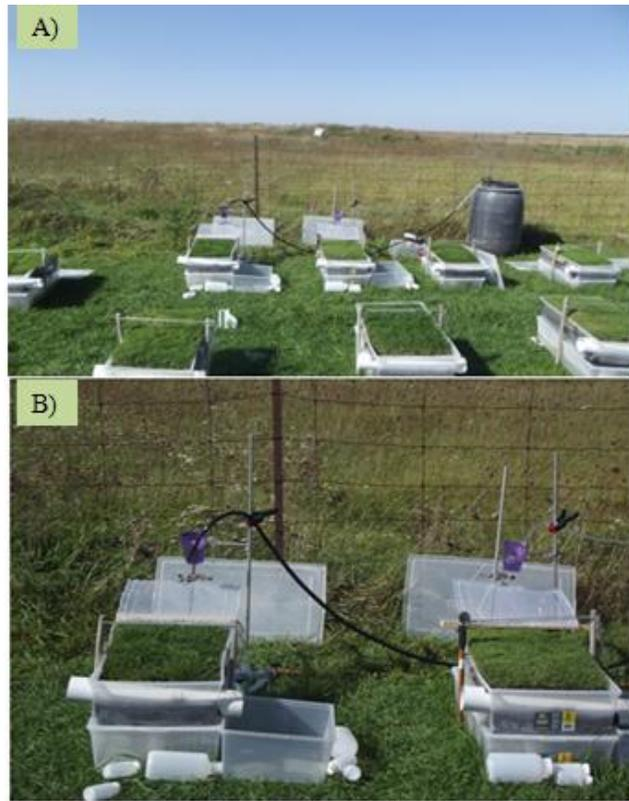
**Figure 8.** Image of storm simulations A) showing the whole set up with rain barrel, B) with a close up view of cups used for measuring flow rates.
