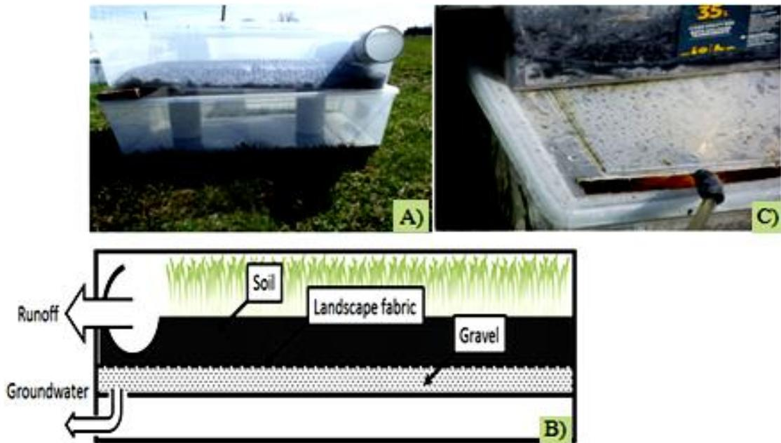
**Figure 2.** Display of the layering described in the bottom of the mesocosms A) and B) with dimensions 70.2 cm x 40.0 cm x 16.5 cm. Shown in C) is the type of cut that has been made to allow infiltrate to be collected.
