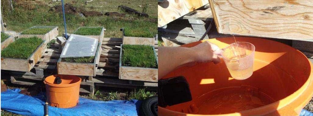
**Figure 6.** A 2016 rain simulation with raised mesocosms in progress (left) and collection of infiltrate with measuring cup (right).
