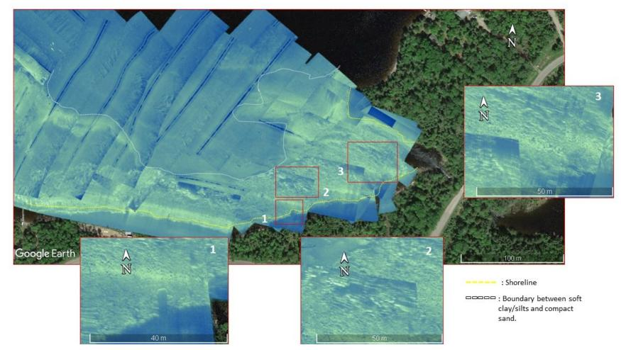
Figure 5.3.2.6. Highlights from the side scan mosaic east of the Portage Island Site (DeJj-8). 1) Large boulder resting amongst a layer of cobble; 2) Patch of rocks and cobble armour; 3) Patch of rocks and cobble armour. Yellow dash-marks represent the outline of the shoreline. White dash-marks represent a boundary between the hard surfaces of the near-shore zone and the soft sediments found in the away from shore.
