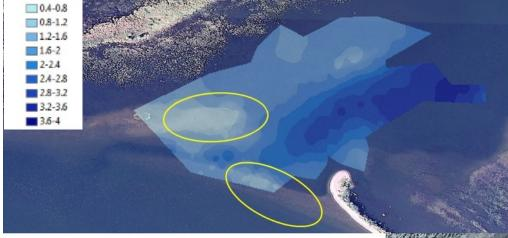
Top: **Vector** (IDW) bathymetric output from a preliminary survey on Arrow Lake, near the mouth of Frog Portage. ESRI's ArcMap was used to interpolate the data points originally collected using a Garmin 525 Chart Plotter sonar system.
