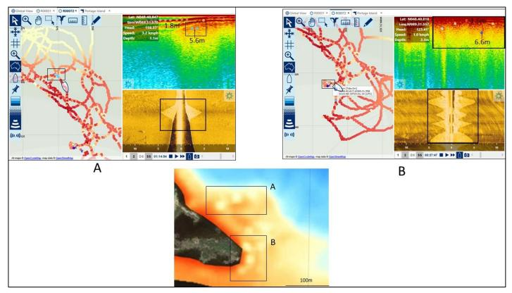
Figure 6.1.1.6. Anomalies in the bathymetric output (areas A and B) are compared to the sonograms taken from the same area. Evidence suggests human error caused the anomalies.
