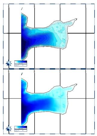
Figure 4.3.1. Top) Vector bathymetric map of the southeast bay located on Cloud Lake. Bottom) Raster map representing the same southeast bay on Cloud Lake.
