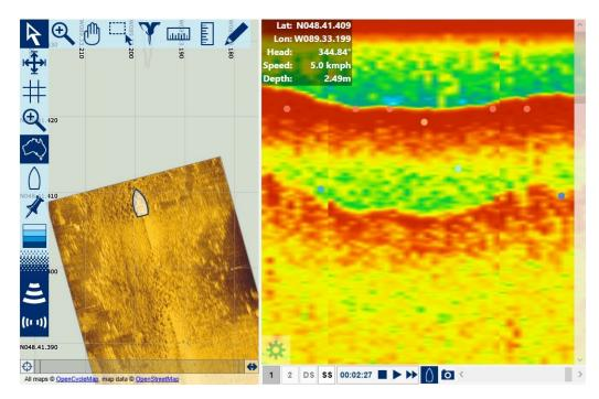
Figure 6.1.1.5. Right) Echogram of track R0091 shows that some of the depth returns are at odds with the bottom profile. Left) Side scan image (sonogram) of the R0091 track detecting the field of rocks and cobble below the transducer.
