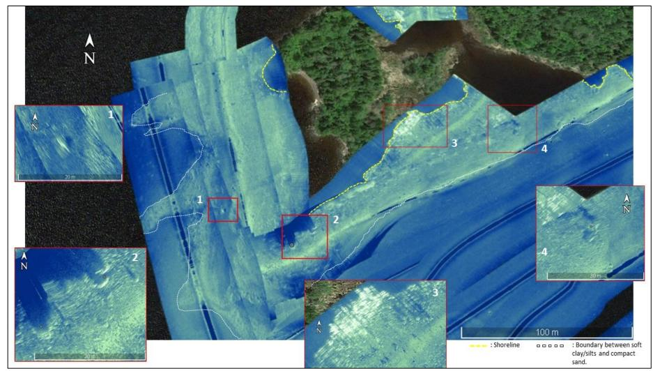
Figure 5.1.2.6: Highlights from the side scan mosaic at the Hawk Bay Site (DeJj-2). 1) Small-Medium Boulder; 2) Large Boulder/Erratic resting against shoreline; 3) Potential bedrock feature or cluster of rocks/cobble. Yellow dash-marks represent the outline of the shoreline. White dash-marks represent a boundary between the hard surfaces of the near-shore zone and the soft sediments found in the away from shore.
