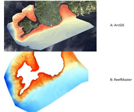
Figure 6.2.1. Comparison of the ArcGIS and ReefMaster bathymetric rendering of the Hawk Bay site.
