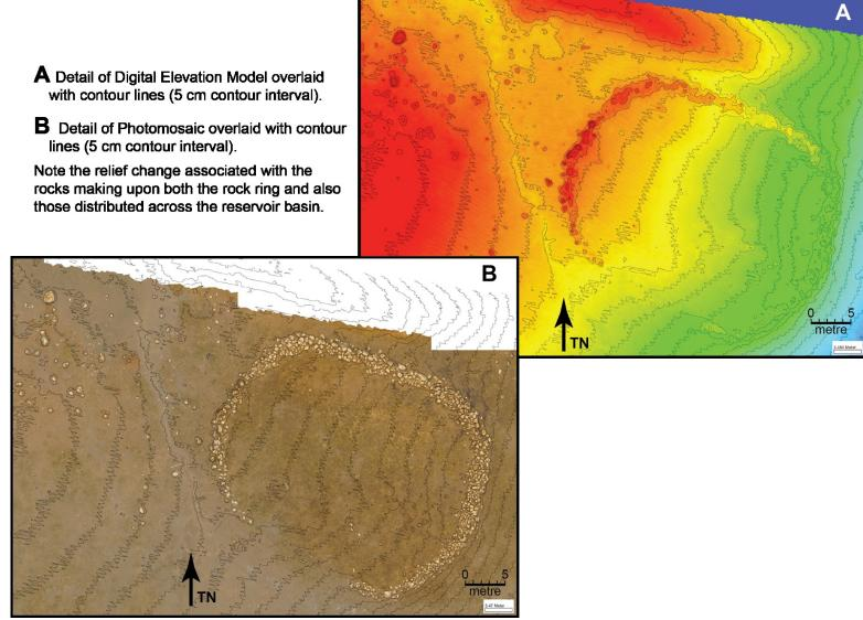
Figure 5.2.4.3. Elevation models of the rock circle and surrounding terrain with 5cm contour resolution (from Hamilton, 2017). Elevation data is relative and not tied to ASL.
