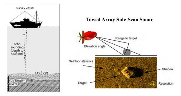
Figure 4.1.1. Left: Schematic depicting how acoustic pulses reflect off the bottom to determine depth (after Powers et al., 2010). Right: Representation of how the range and angle of the sonar beam reflect off the target, and create a shadow (from Hansen, 2012).
