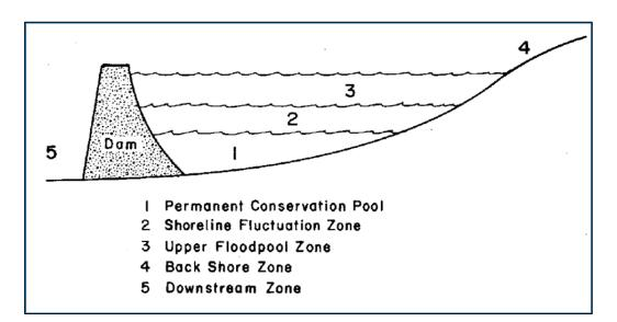
Figure 3.2.1. A schematic labeling the different pools and zones that are impacted by a hydroelectric dam (borrowed from Lenihan et al., 1982).
