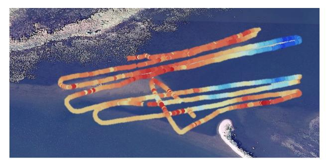
Figure 5.1.1.3. Tracks of data points (depth measurements) collected near the mouth of Frog Portage, on Dog Lake. Colour coding of the data points reflect depth changes (Red reflects a shallower water column, while Blue represent a deeper area).
