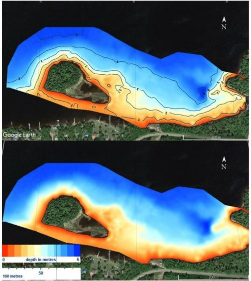
Figure 5.2.3.1: Bathymetric TIN raster of the Portage Island Site and the southeastern near-shore zone of Hawk Bay. Top)Map 1; Bottom) Map 2.
