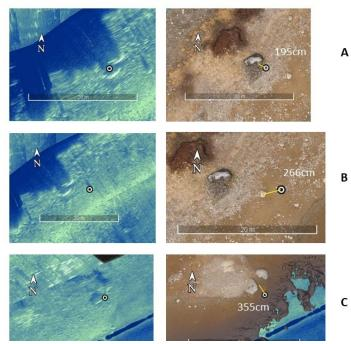
Figure 5.1.2.8. Comparison of spatial accuracy between the side scan sonar, and imagery captured with the UAV at the Hawk Bay Site.
