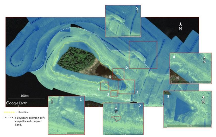
Figure 5.2.3.5. Highlights from the side scan mosaic at the Portage Island Site (DeJj-8). 1) Log, approximately 10m in length ; 2) Patch of rocks and cobble; 3) Large boulder and vegetation; 4) A cluster of rocks, cobble and vegetation; 5) A mix or rocks and hard-packed sediment (sand).. Yellow dash-marks represent the outline of the shoreline. White dash-marks represent a boundary between the hard surfaces of the near-shore zone and the soft sediments found in the away from shore.
