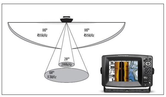
Figure 4.1.2. Left: frequency of and coverage area of the side scan and down imaging beam. Right: Counsel of the acquisition of bathymetric and side-scan data. Humminbird 899ci SH HD fish finder.
