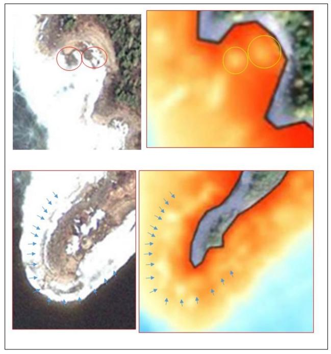
*Figure 5.1.2.2. Features represented in the bathymetric data (Right) are evaluated and compared to satellite imageryobtained from Google Earth.*
