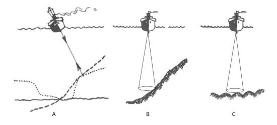
Figure 6.1.1.4. Common variables that can affect the vertical accuracy of a Single Beam Echo Sounder include: A) Vessel motion such as yaw, pitch and roll; B) Size of the acoustic footprint on a severe slope; C) The composition of the bottom (i.e. hardness, size, and shape) (after Honeywell Elac Brochure).
