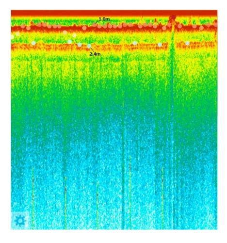
*Figure 6.1.1.3. Echogram reflecting the errors in depth, as some of the data points are falling below the first echo return (E1).*
