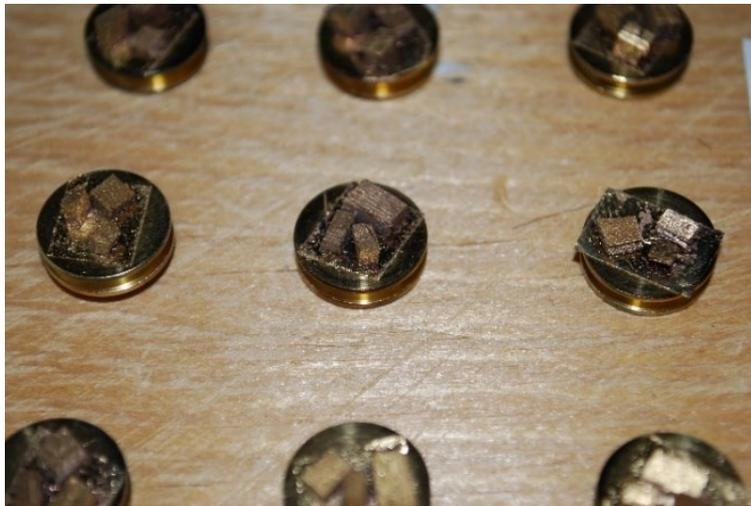
Figure 2.20 Gold-covered samples mounted on pegs (Courtesy of Dr. Leitch, 2016).
