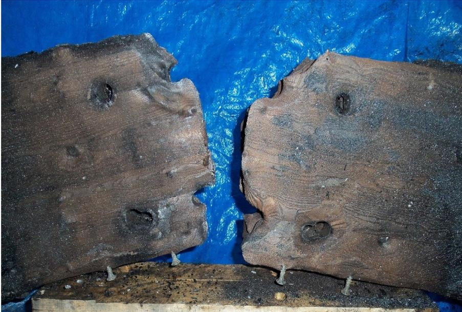
(a) Charred layer removed from Test 1FS assembly (four-bolt strengthened connections with four-times bolt diameter end distance).
