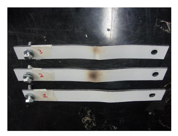
Figure 4.16: Closer view of damaged bracing
