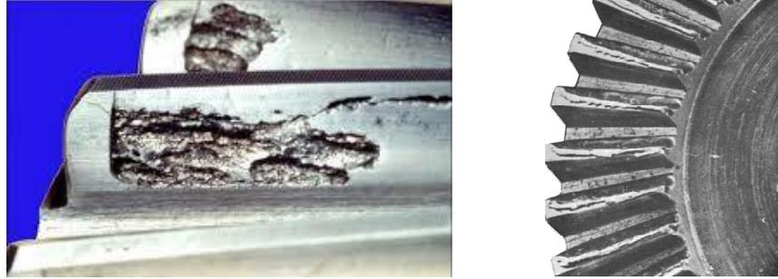
**Figure 1.3.** Sever scoring defect in gears [16].
