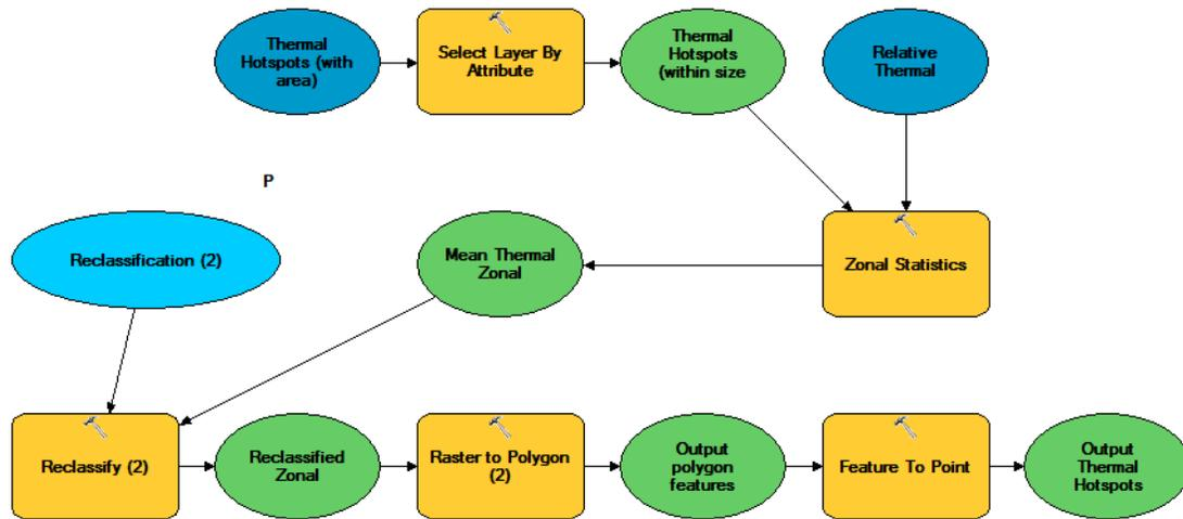
**Figure 4.2.4.** The final part of the model takes the relative thermal raster and the thermal hotspot polygons to create zones where thermal hotspot polygons within the size constraint of  $0.5 \text{ m}^2$  to  $4.0 \text{ m}^2$  are located. The mean relative thermal value is calculated within each zone. Zones with hotspots greater than  $0.5$  Celsius degrees are identified as moose and exported as point shapefiles for analysis and examination. Diagram symbology is as in Figure 4.2.2.
