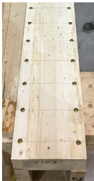
Figure 3.13. Bottom side of a finished screwed beam assembly
