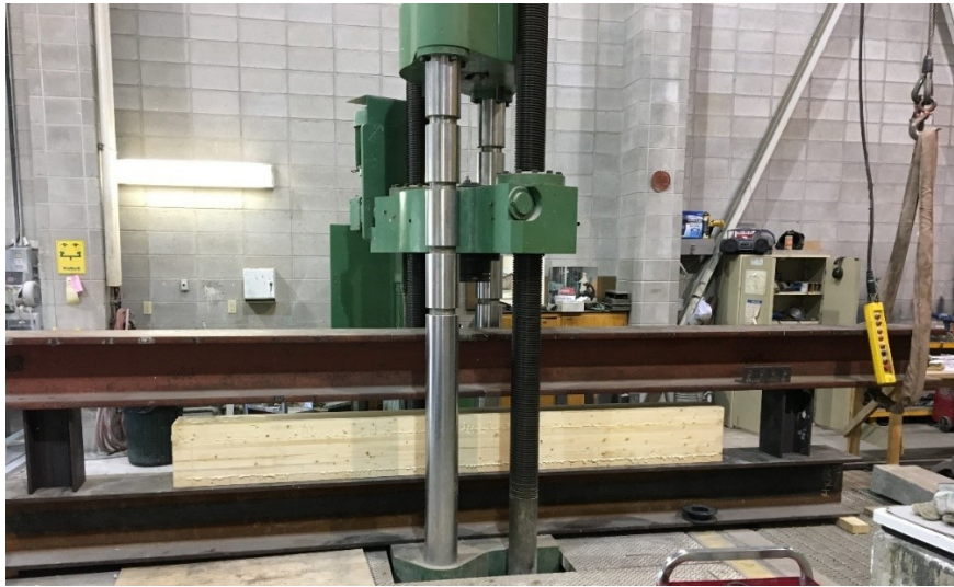
Figure 3.15. Built-up beam assembly right before applying pressure
