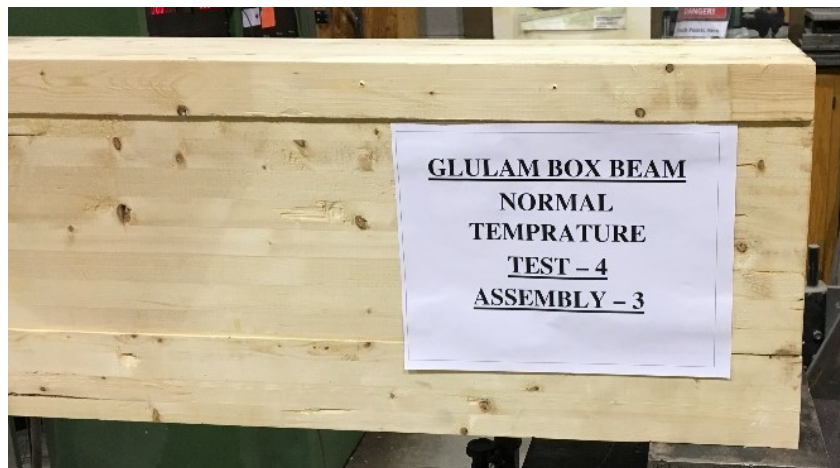
Figure 3.17. Finished glued built-up glulam box-section beam assembly
