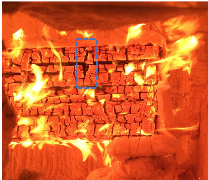
Figure 5.11. Wood charring and exposed screw in a screwed built-up beam assembly during fire resistance testing
