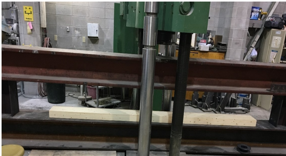
Figure 3.14. A glulam bottom flange panel temporary placed in hydraulic compression press system
