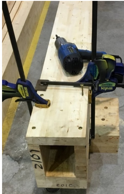
Figure 3.12. Screws thrusting at top side of the beam assembly
