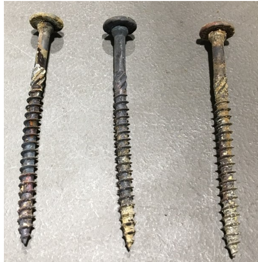
(a) Yielding in top screws due to shear stresses and fire exposure
