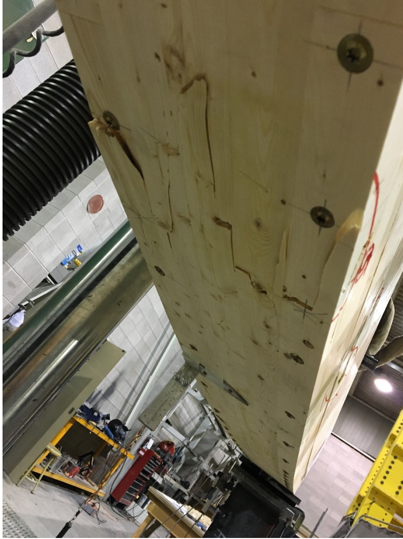
Figure 4.10. Brittle failure in the bottom flange of a general screwed beam assembly
