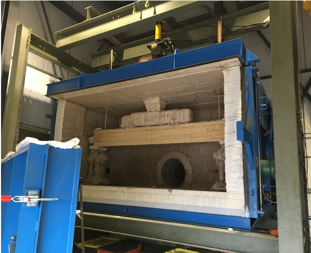
Figure 5.5. A general test setup inside the fire testing furnace
