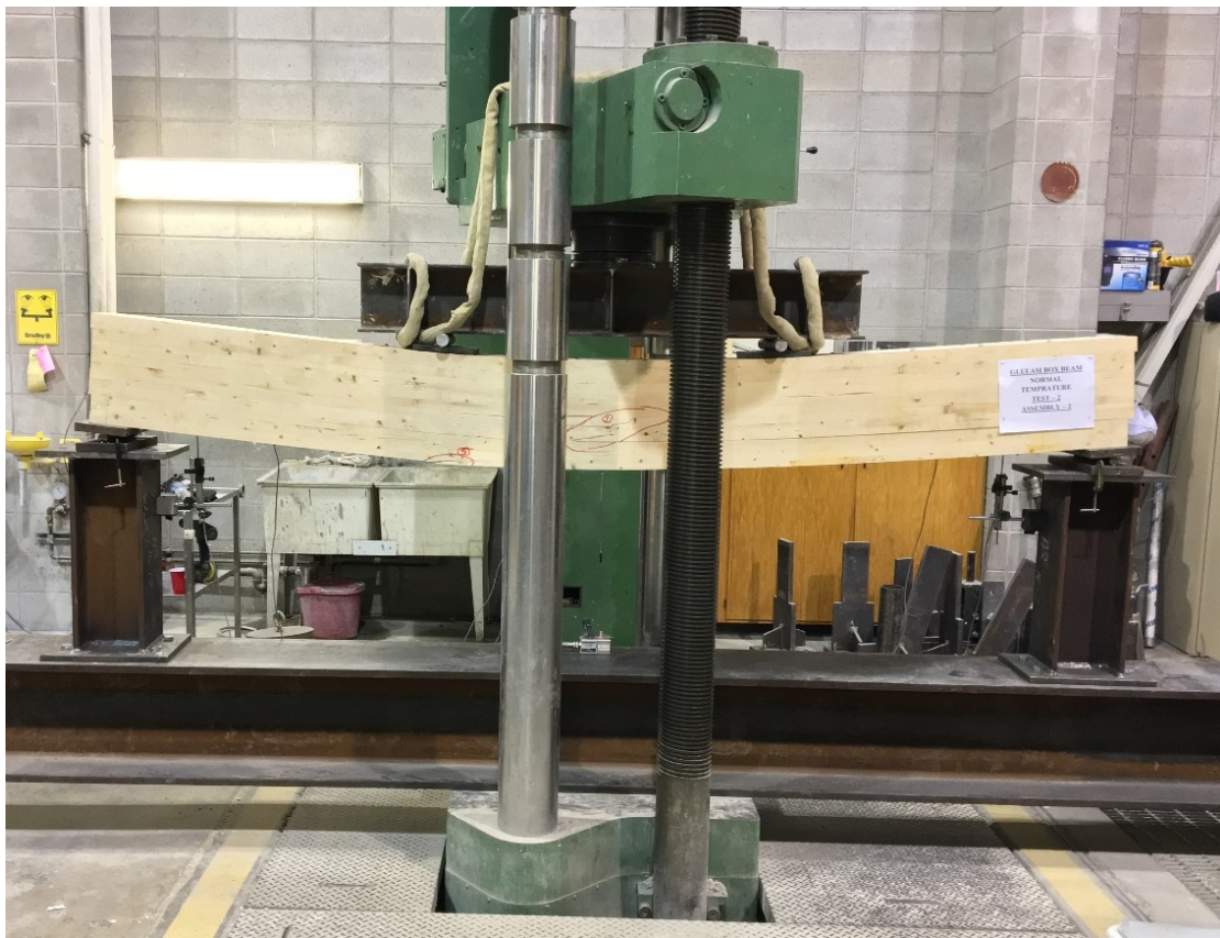
Figure 4.1. A general built-up glulam box-section beam assembly undergoing testing
