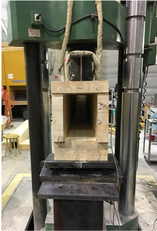
(a) Front view of the relative slips between the flanges and the web panels
