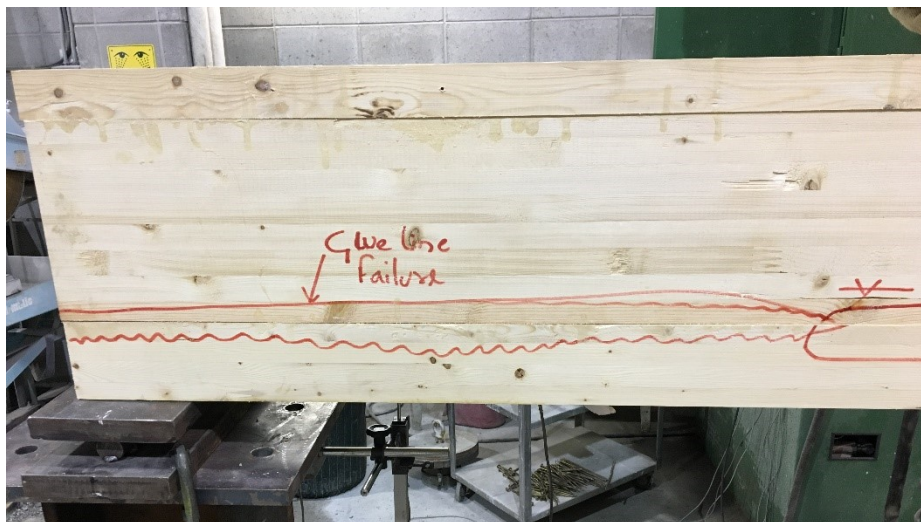
Figure 4.15. Ultimate shear failure in glue line
