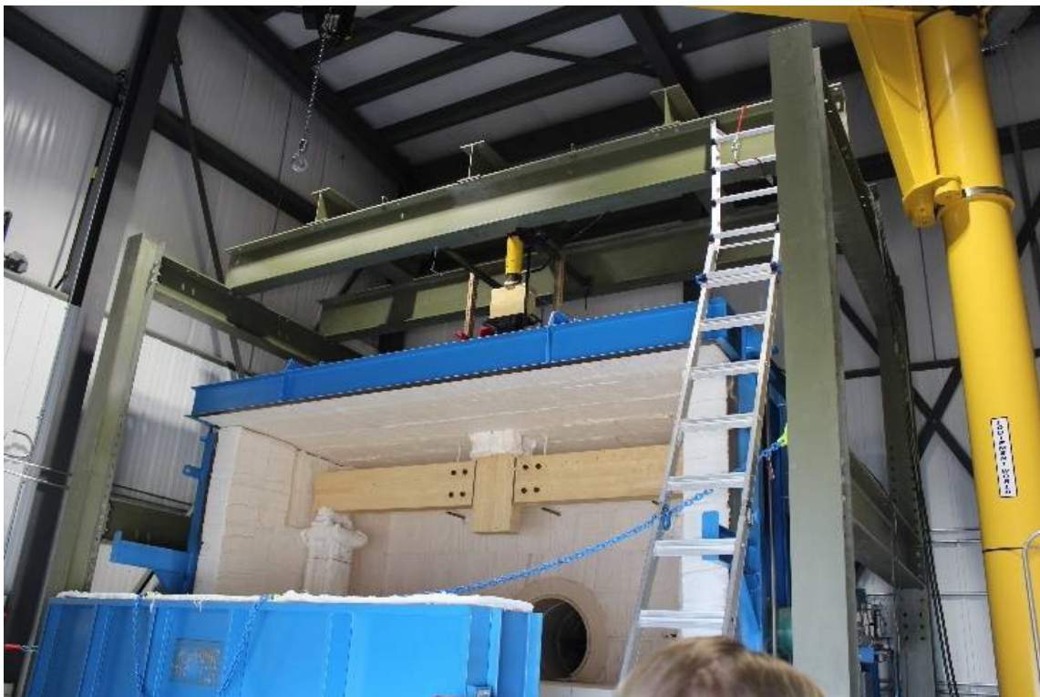
Figure 5.2. Large custom-designed fire testing furnace accommodated at LUFTRL
