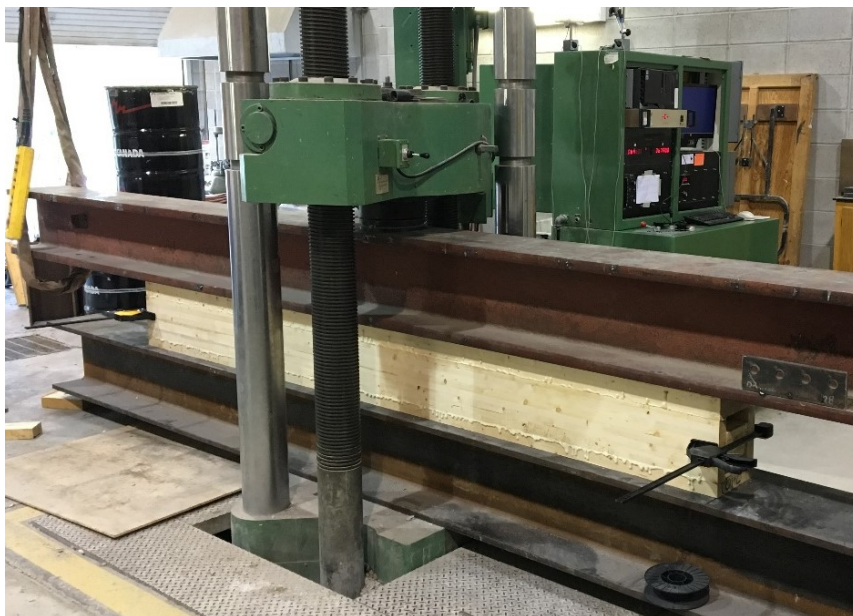
Figure 3.16. Applying compressive pressure on the built-up beam assembly
