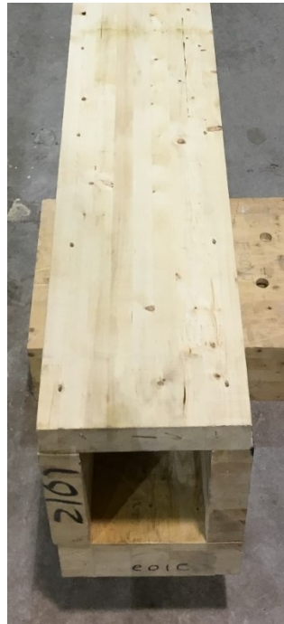
Figure 3.11. Pilot holes drilled through the top side of the beam assembly
