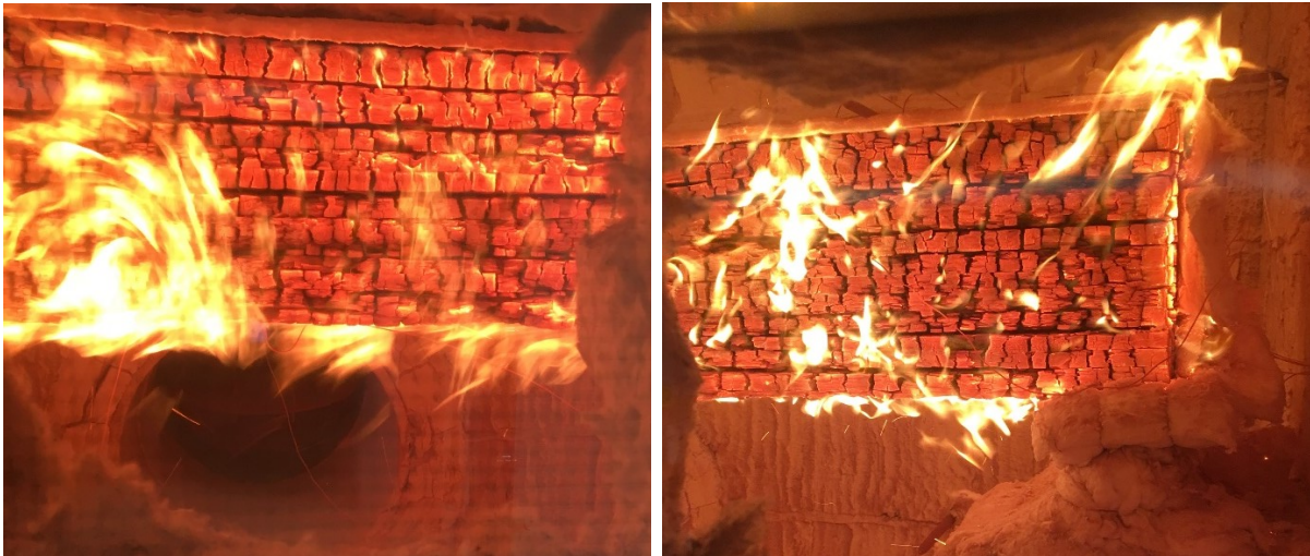
Figure 5.6. A general beam test assembly undergoing fire resistance testing
