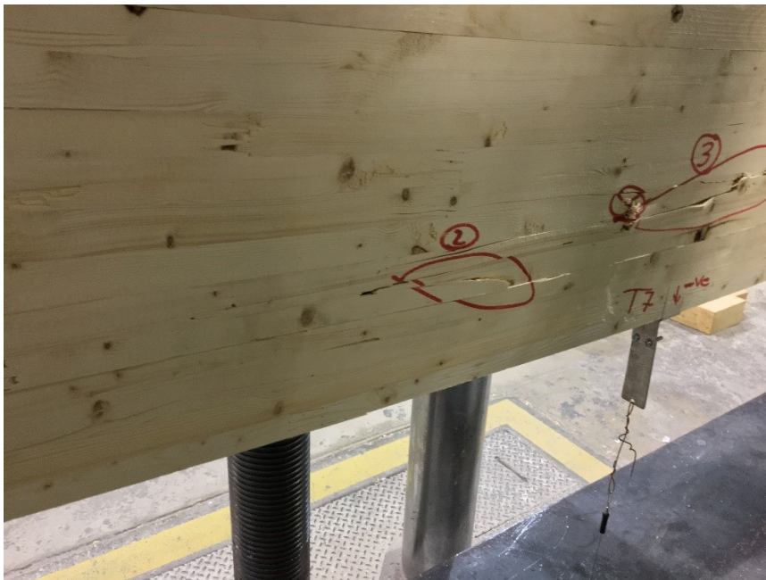
Figure 4.9. Rolling shear failure in the web panel of a general test assembly
