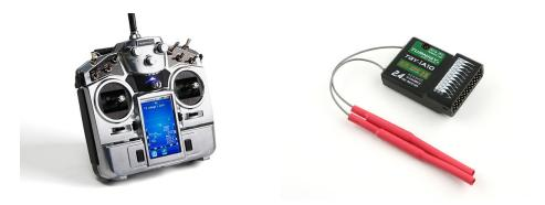
Figure 4.8: (a) RC Transmitter; (b) RC Reciever
