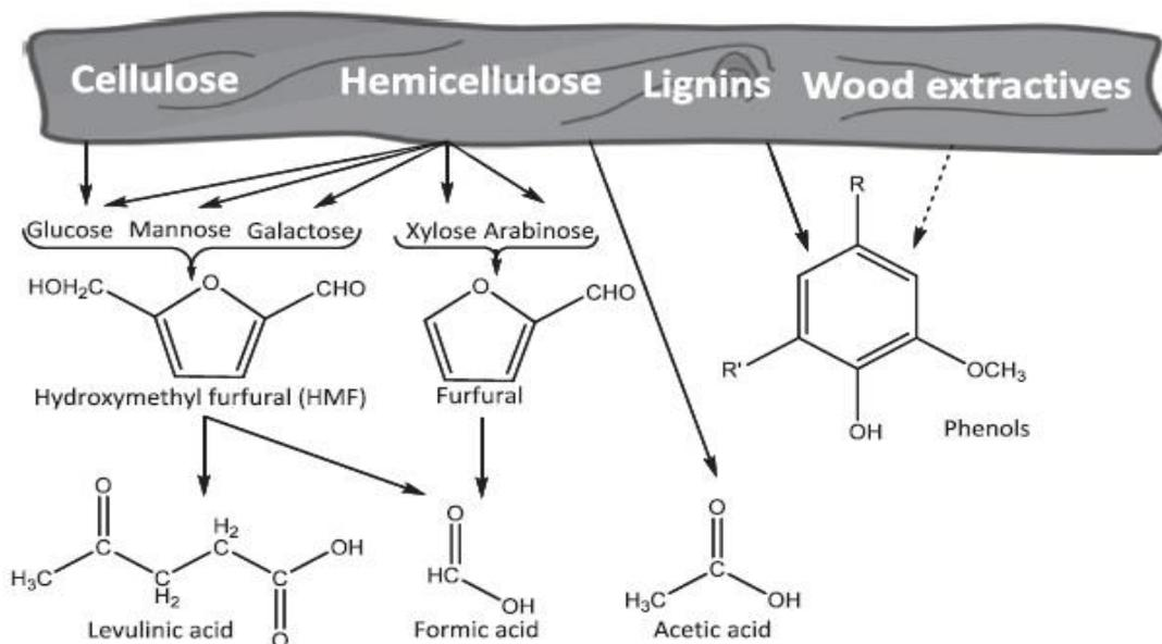
**Figure 2.8 : Formation of inhibitors (Jonsson et al., 2013)**
