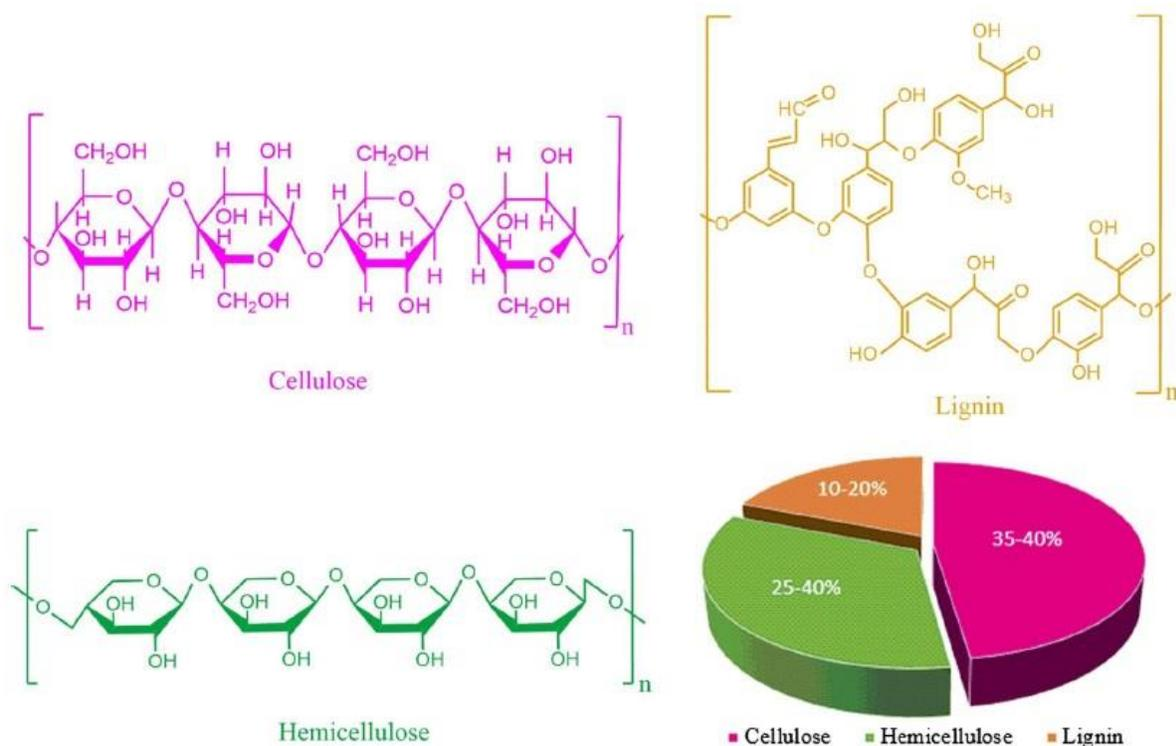
**Figure 2.1:Composition of lignocellulosic Biomass (Amin et al., 2017)**
