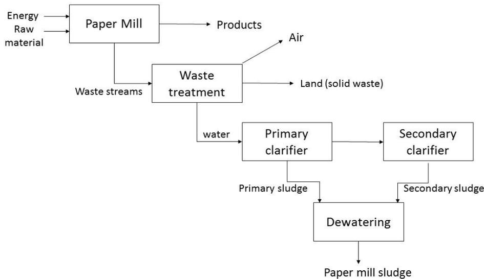
**Figure 2.3: Schematic diagram of paper mill sludge**
