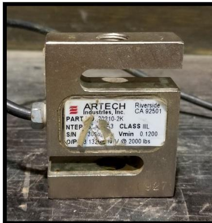
**FIGURE 2.33: ARTECH 20210-2K LOAD CELL**
