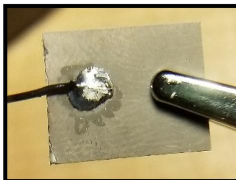
**FIGURE 2.11: A STRONG SOLDER BOND IS MADE WITH THE LEADS AND THE ELEMENT**
