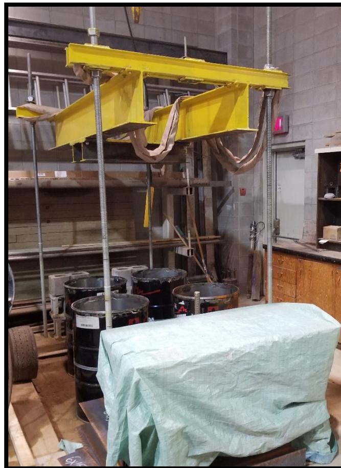
**FIGURE 2.35: BARRELS WITH LOADING FRAME ABOVE AND CONTROL CENTRE IN FRONT**
