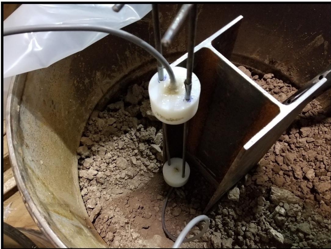
**FIGURE 2.17: ORIENTATION OF BENDERS NEXT TO PILE WITH ALIGNMENT RODS INSERTED**
