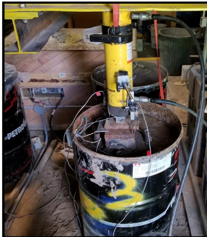
**FIGURE 2.31: BARREL 3 WITH LOADING RIG ABOVE PILE WITH WIRING AND CONDUIT STILL IN PLACE**
