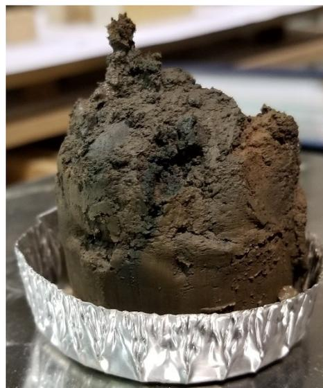
**FIGURE 3.21: SAMPLE TAKEN ADJACENT TO TREATED PILE**
