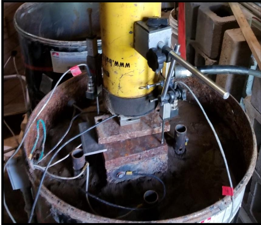
**FIGURE 2.32: PILE READY FOR LOADING WITH DISPLACEMENT AND STRAIN GAGES IN PLACE**
