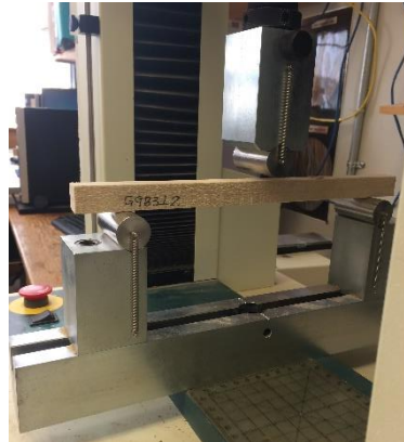
Figure 3. A sample stick ready to be tested for MOE and MOR values.
