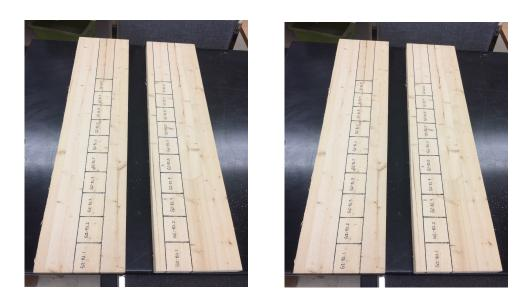
Figure 10. Labeling of the replicate blocks on the sawn boards.
