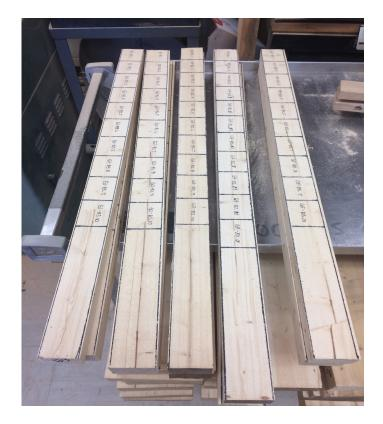
Figure 11. 2" sticks sawn using the table saw and ready to be sawn into replicates.
