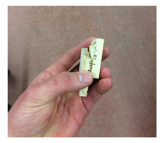
Figure 17. A replicate shorn on the glue line after the test was completed.
