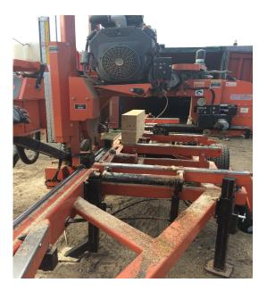
Figure 7. A glulam bolt being halved at  $6\frac{1}{4}$ ".
