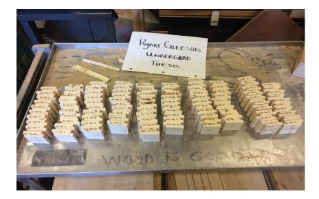
Figure 13. Replicates at the final dimensions, with saddles cut from each end, ready for testing.
