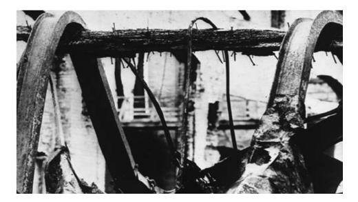
Figure 1. A wood beam that survived the fire in the casein plant in Frankfort, New York. Source: Rowell (2005)
