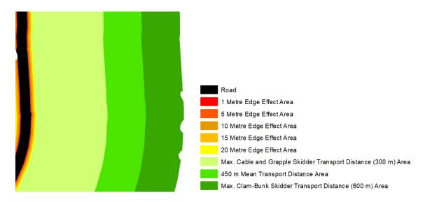
Figure 10. Example of road edge effect areas and maximum harvestable areas using buffers from road edge.
