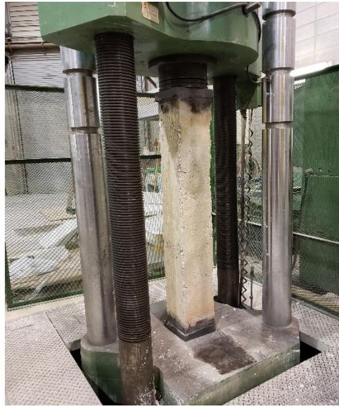
**Figure 3.15** Axial compression test setup
