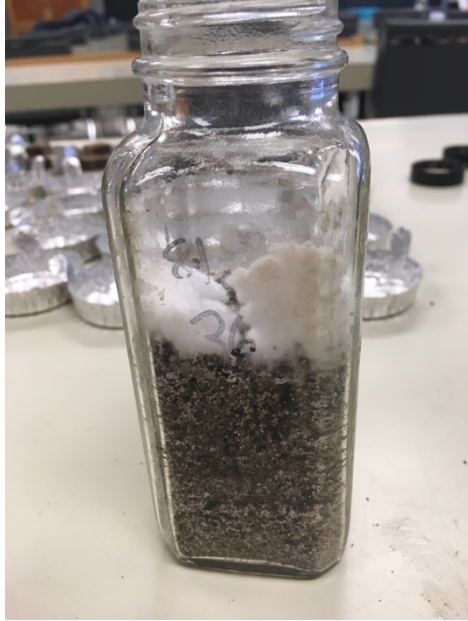
Figure 3 Visible mycelium in with a decaying sample.
