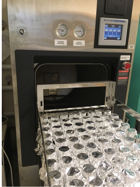
Figure 2 Prepared Quorpak bottles being put into the autoclave.
