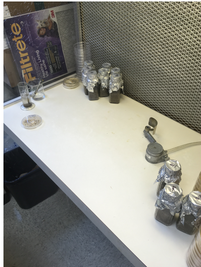
Figure 1 Set up for inoculation process with Bunsen burner, 70% alcohol for sterilization, fungi, and Quorpak bottles.
