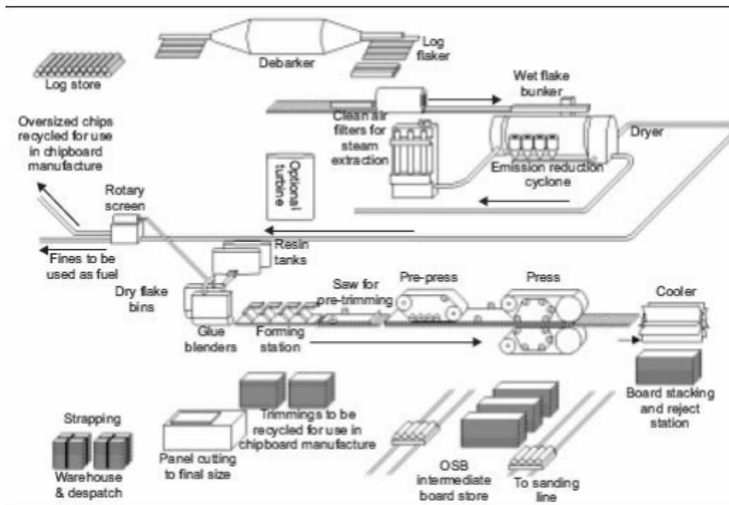
Figure 1. Figure of OSB Manufacture Process (Source: Board, 2006)
