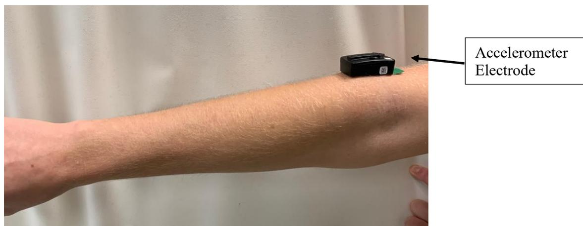
*Figure 11.* Wireless EMG electrode placed on the elbow to measure acceleration.
