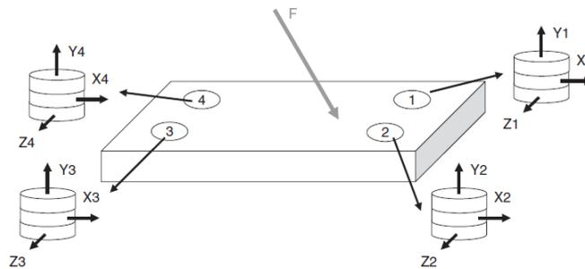
Figure 3. Diagram of a force platform. Adapted from “*Biomechanical Evaluation of Movement in Sport and Exercise*,” by Payton & Bartlett, 2007, Routledge, Milton Park: AB
