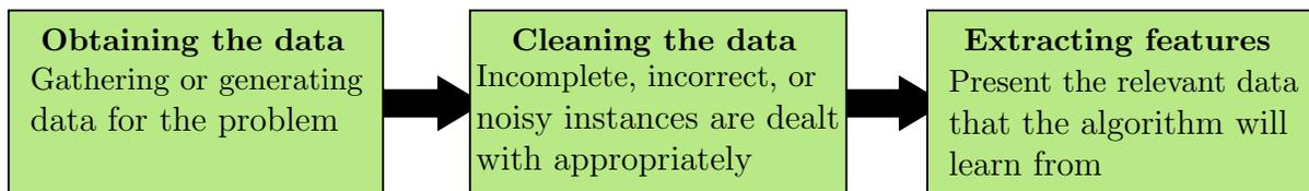
Figure 2.4: Simplified steps for data processing in machine learning to ensure that the algorithm has a clean dataset to work with.
