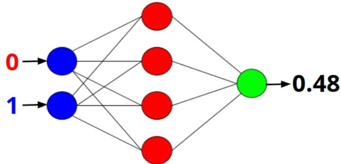
Figure 3.10: An example MDQ network that takes the previous and current state of an individual as an input and outputs an optimal transition probability.
