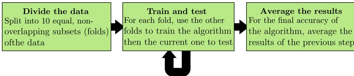
Figure 2.5: An overview of the process for 10-fold cross-validation which is an accurate and fair way to evaluate machine learning models on a given dataset.
