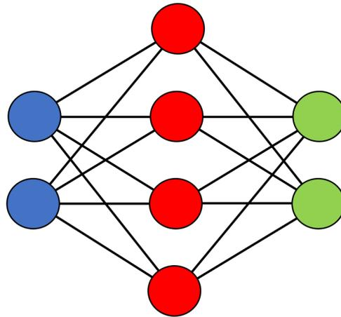
Figure 2.7: A basic example neural network where the *blue* neurons are the inputs, *red* are part of the hidden layer, and *green* are the outputs.
