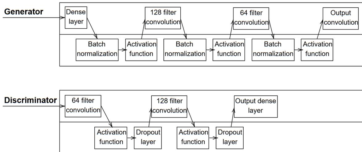
Figure 5.2: An overview of the layout that the DCGAN in this chapter uses.
