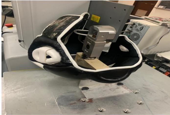
Figure 16: Front static compression test of the Adidas® headguard.
