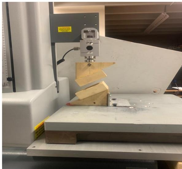
*Figure 14:* Chatillon® TCD1100 Force Tester with modified block formation.
