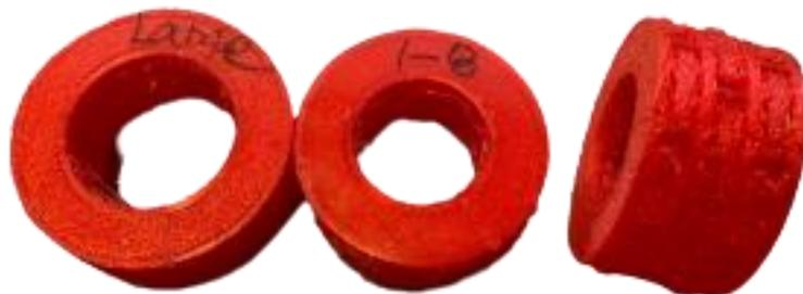
*Figure 11:* TPU inserts. The three large (left) and small (middle, right) 3D-printed TPU inserts used in this study.
