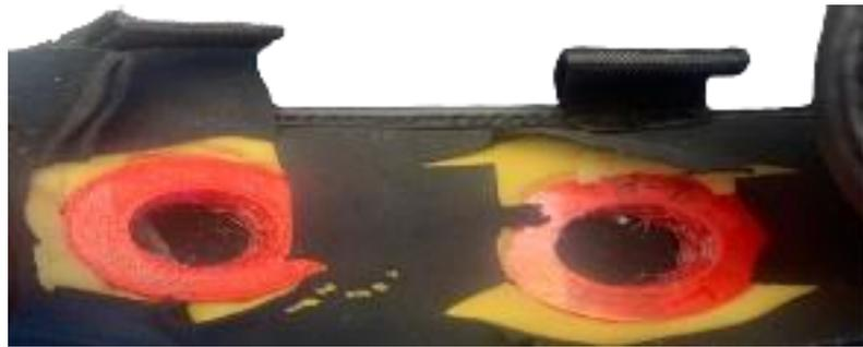
*Figure 12:* TPU inserts placed into Century® Drive headguard. Cut Century® Drive headguard with a large TPU insert at the front (right) and a small TPU insert at the front boss (left) impact locations.
