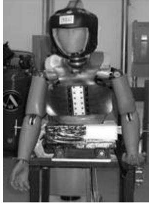
*Figure 2:* The Hybrid III head, neck and torso model with boxing headguard. Adapted from “Biomechanics of the head for Olympic boxer punches to the face”, T. Walilko, D. Viano, and C. Bir, 2005, *British Journal of Sports Medicine*, 39 (10), p. 710-719. Copyright 2005 by British Journal of Sports Medicine.
