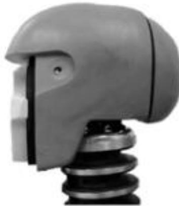
*Figure 3:* The frangible faceform model with the boxing headguard removed. Adapted from “Biomechanics of the head for Olympic boxer punches to the face”, T. Walilko, D. Viano, and C. Bir, 2005, *British Journal of Sports Medicine*, 39 (10), p. 710-719. Copyright 2005 by British Journal of Sports Medicine.
