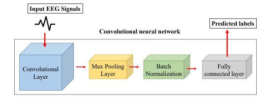
Fig. 3.3 The architecture of a typical convolutional neural network.
