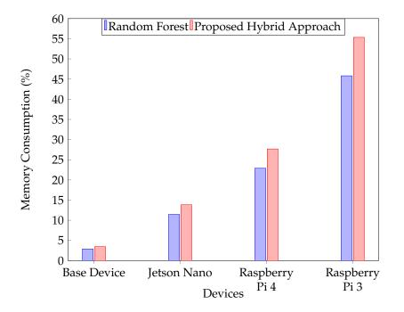
Fig. 5.9 Numeric analysis of memory consumption of two best performing algorithms on various ultra-edge devices.
