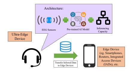
Fig. 1.2 Proposed logic-in-headbands-based edge analytics framework to facilitate localized EEG computing.
