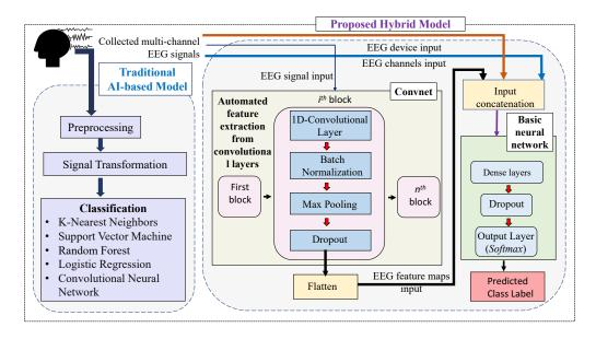
Fig. 5.1 The architecture of our proposed hybrid model vs. traditional AI-based algorithms.
