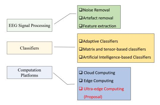
Fig. 2.1 The processing techniques of the EEG signals in the literature.
