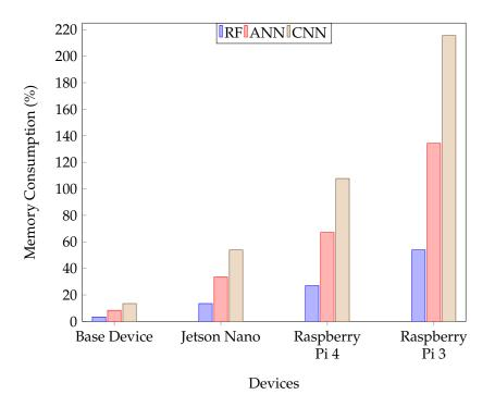
Fig. 4.6 Percentage of memory consumption of selected algorithms with respect to various devices.
