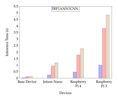
Fig. 4.7 Inference time of different algorithms in various devices.
