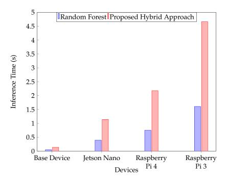
Fig. 5.10 Numeric analysis of inference time of two best performing algorithms on various ultra-edge devices.
