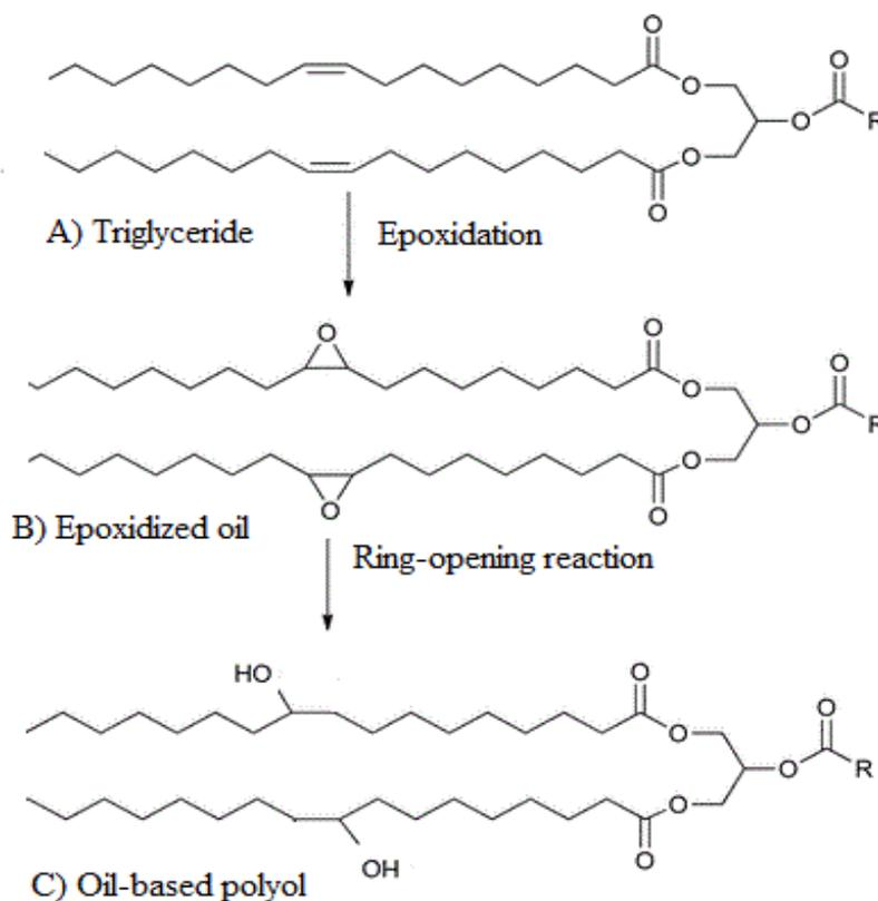
Fig. 2.2. Schematic illustration of microbial lipid-based polyol through epoxidation and ring-opening reaction.
