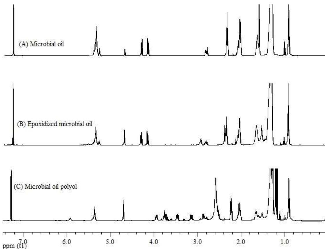
Fig. 4.5. <sup>1</sup>H NMR spectra of (A) microbial oil (B) epoxidized microbial oil (C) microbial oil polyol produced in this study.
