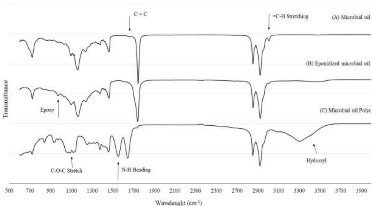
Fig. 4.4. IR spectra of (A) microbial oil (B) epoxidized microbial oil (C) microbial oil polyol produced in this study.
