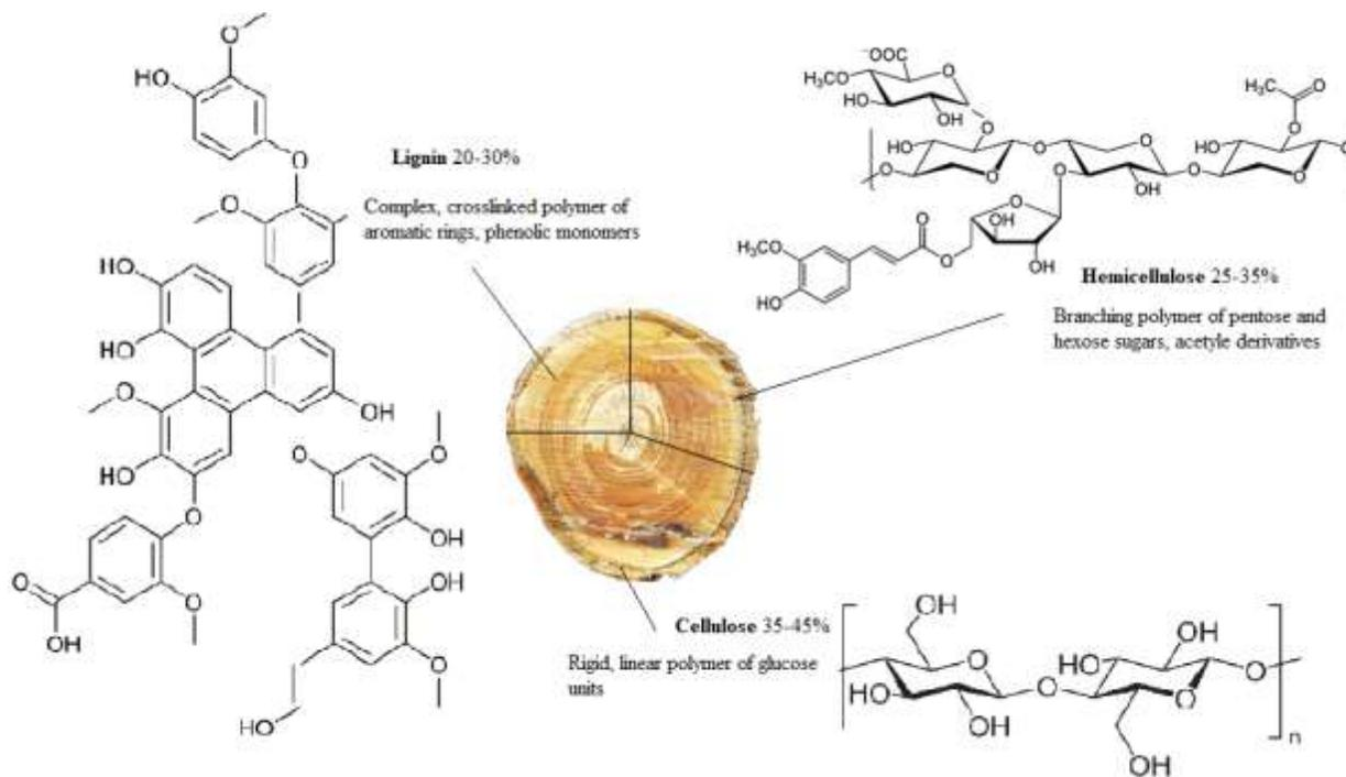
Fig. 2.1. Structure of components of lignocellulosic biomass.
