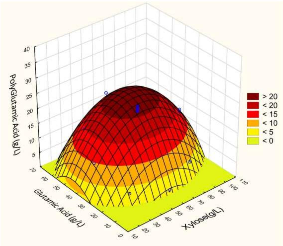
Fig. 5.1. Surface plot of  $\gamma$ -PGA production using central composition design illustrating the effect of glutamic acid and xylose concentration.
