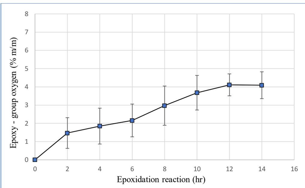
Fig. 4.3. Oxirane content of epoxidized microbial oil as a function of time during epoxidation reaction using Novozym 435 as catalyst.
