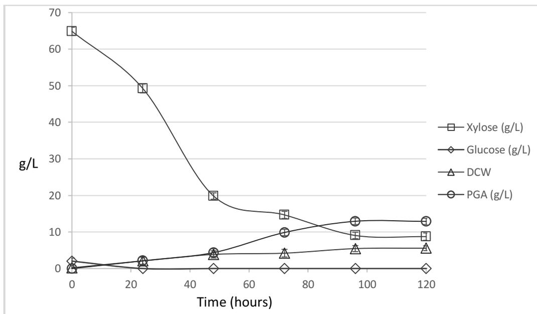
Fig. 5.2. Total cell biomass,  $\gamma$ -PGA and sugar concentration in flask shake fermentation of *B. subtilis* (ATCC 23857) grown on steam treated Poplar wood hemicellulose pre-hydrolysate (HPHL) used in this study under optimized condition.
