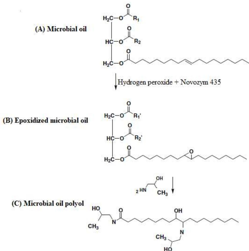
Fig. 4.2. Overall reaction scheme for the synthesis of microbial oil polyol from microbial oil using *C. curvatus* grown on steam treated Poplar wood hemicellulose pre-hydrolysate (HPHL) via enzymatic epoxidation and ring opening reaction.  $R_1$  and  $R_2$  are the fatty acid chain.
