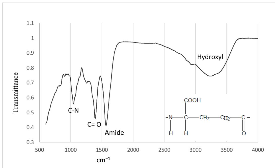
Fig. 5.3. FTIR spectra of purified  $\gamma$ -PGA produced by *Bacillus subtilis* (ATCC 23857) grown on steam treated Poplar wood hemicellulose pre-hydrolysate (HPHL) used in this study under optimized condition.
