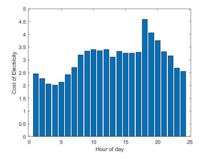
Figure 4.1: Cost of Electricity by hour of day
