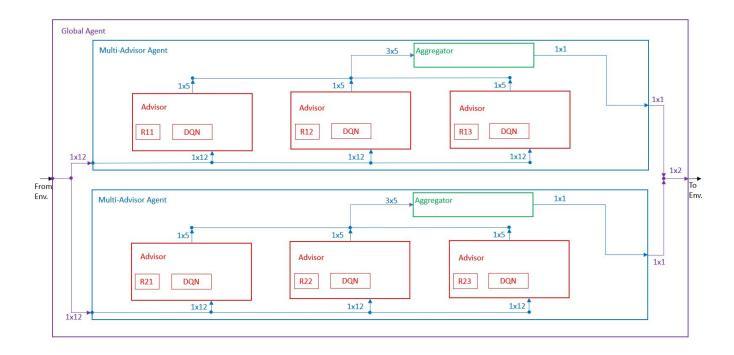
Figure 6.1: Multi-Agent Multi-Advisor Architecture. State is input on the left from the environment, is processed through the agent and it's components, resulting in an action to send to the environment on the right.
