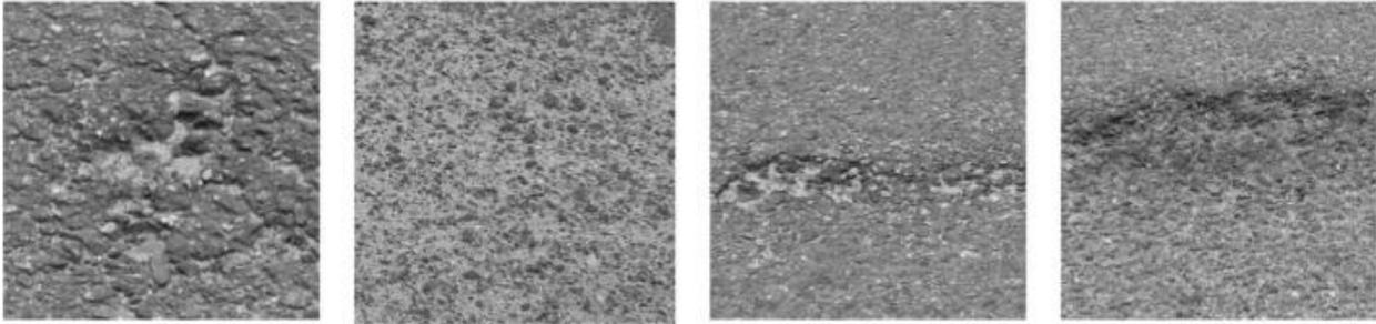
**Figure 4. Examples of raveling on an asphalt road (Hoang 2019b)**
