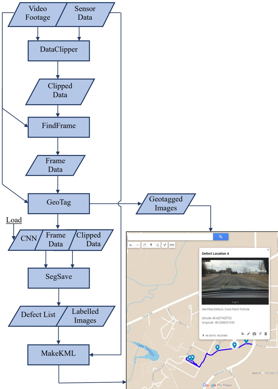
Figure 40. Steps to integrate the motion and video data
