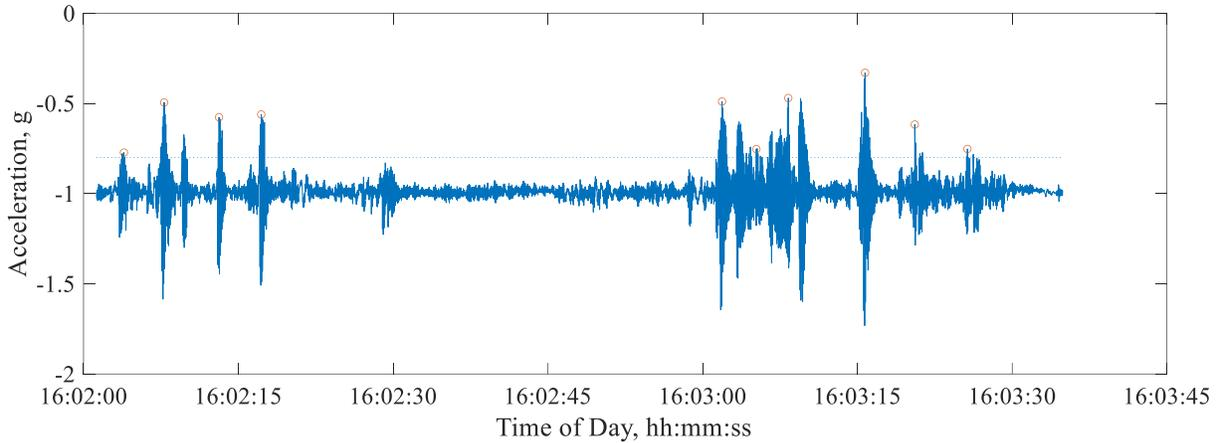
**Figure 29. Acceleration time series plus detected anomalies circled in red.**
