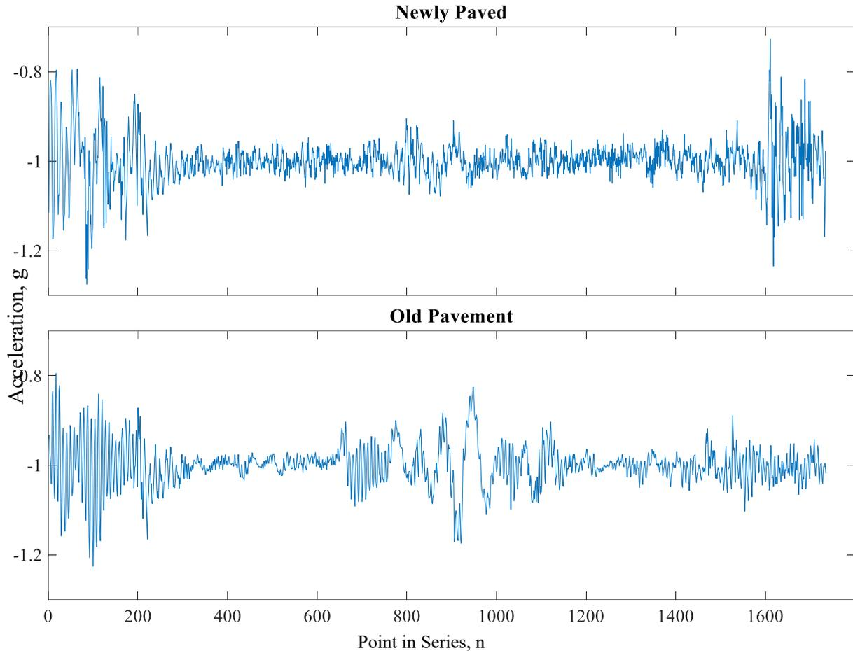
**Figure 49. Plots comparing the same 20-meter stretch of a road before and after paving**
