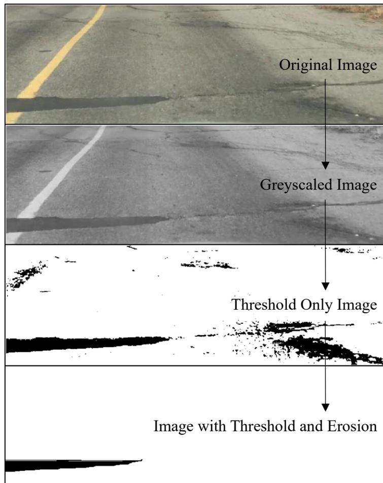
**Figure 36. Image segmented first with a threshold followed by erosion.**
