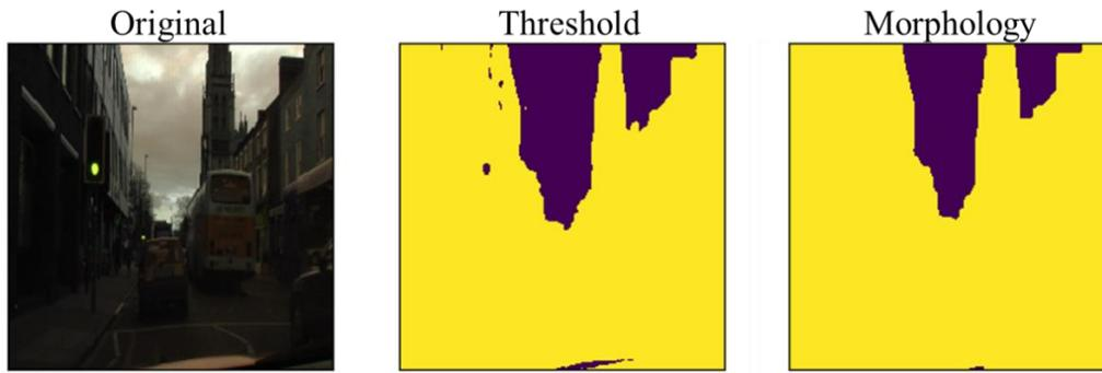
**Figure 15. Identifying the sky in an image using two image processing operations (Canuma 2018)**
