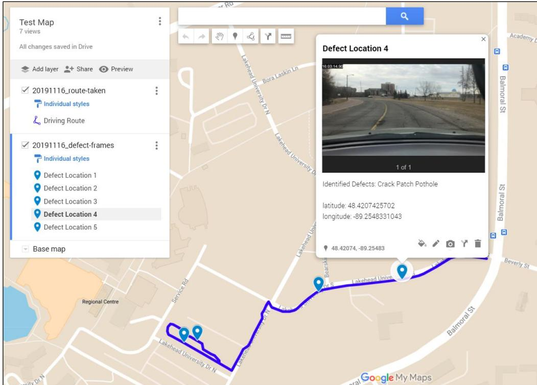
**Figure 42. Example data display of KML files loaded into Google MyMaps**
