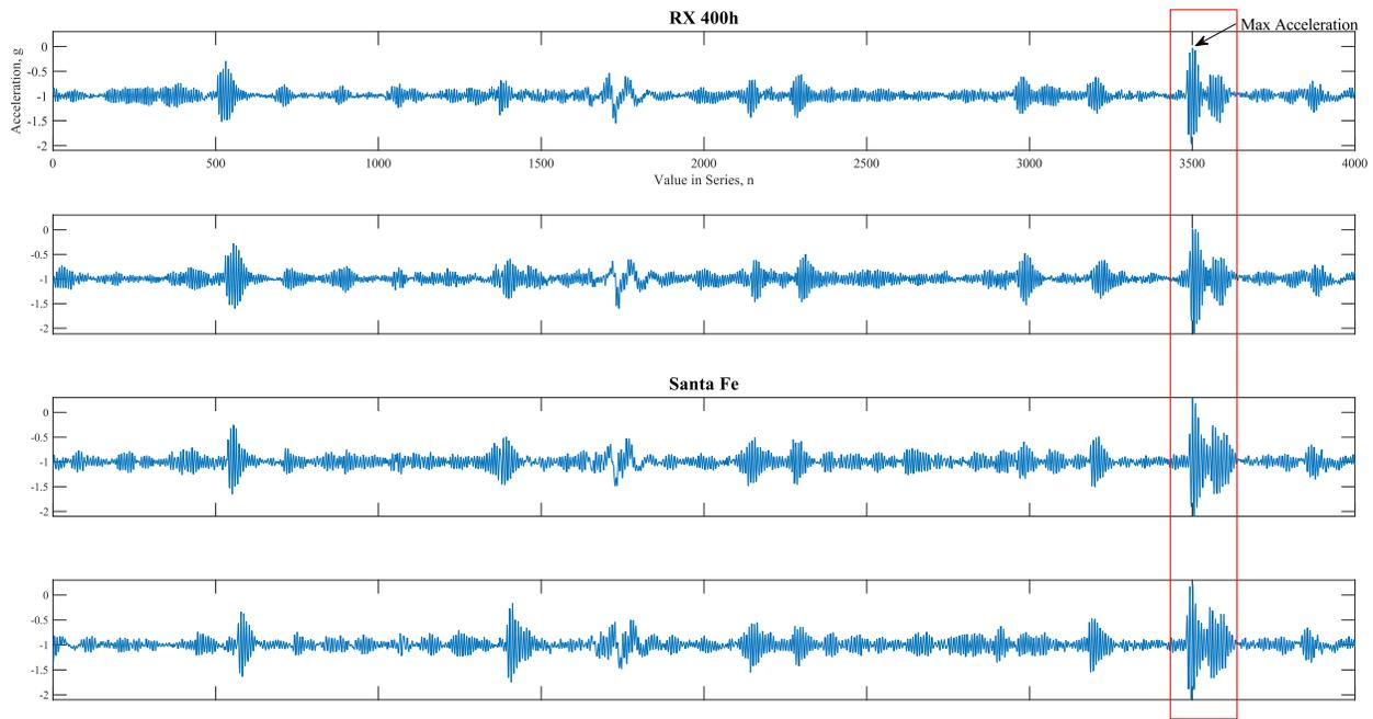
**Figure 43. Comparison of acceleration signals for two different vehicles driving over the same stretch of a road twice**
