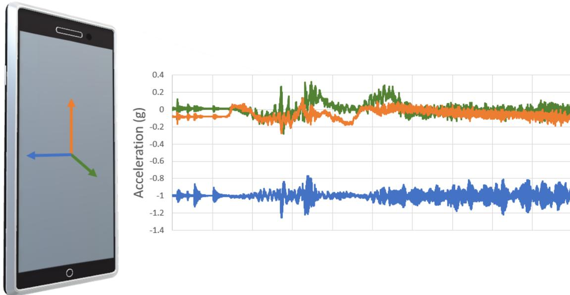
**Figure 10. Triaxial acceleration measurements from a smartphone**
