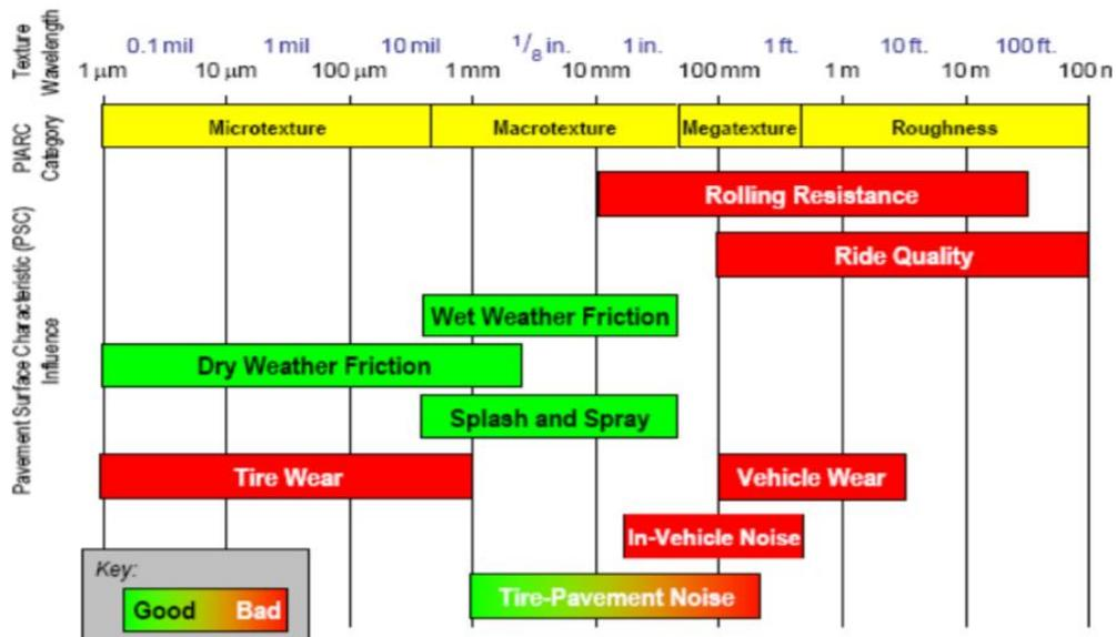
Figure 7. Basic elements of road texture and their impact on driving (Cackler et al. 2006)
