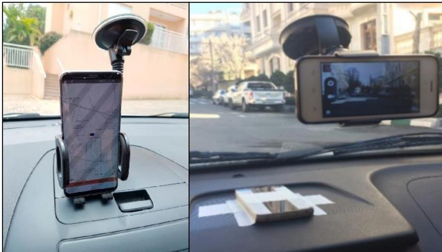
**Figure 12. Left: windshield-mounted smartphone (Souza et al. 2018); Right: dashboard- and windshield-mounted phones (Yeganeh et al. 2019)**
