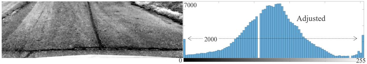
**Figure 34. Contrast enhanced image using gamma correction, plus its histogram**
