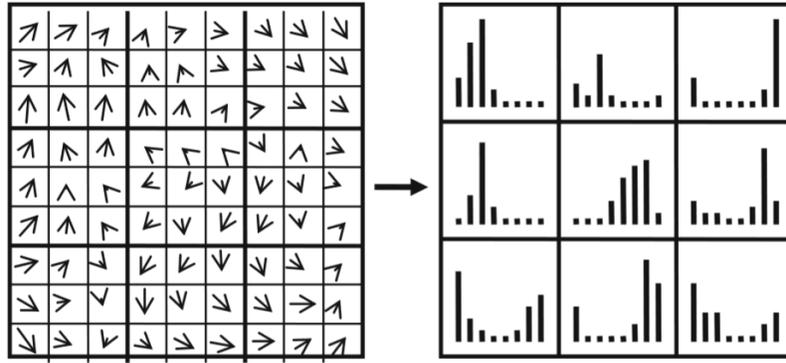
**Figure 16: Gradient orientations (left) and their distributions (right) for the SIFT feature descriptor (Treiber 2010)**
