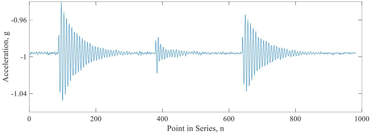
**Figure 50. Damped free vibration behaviour noticed in the data collector**
