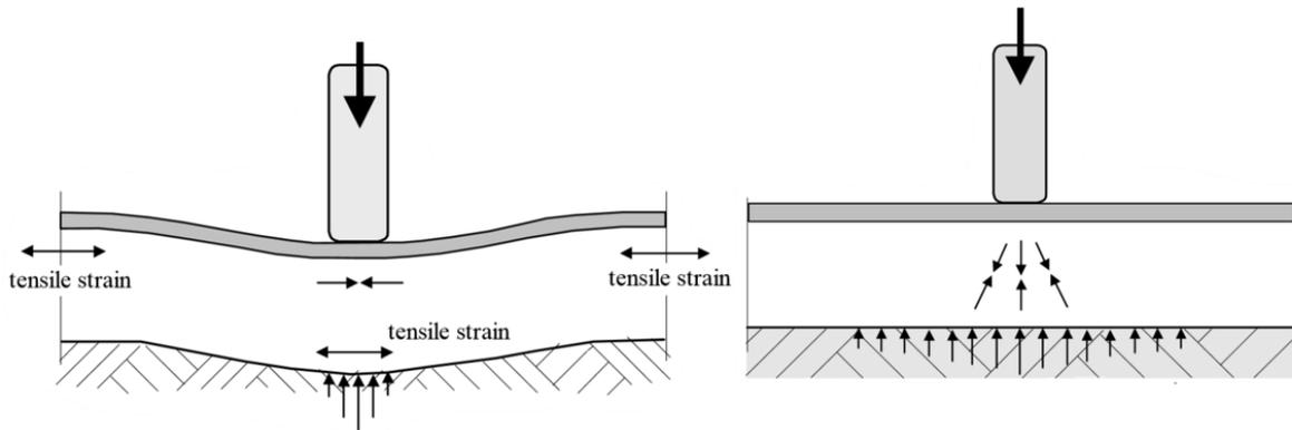
**Figure 3. The idealization of flexible (left) and rigid (right) pavement structures (Lay 2009)**
