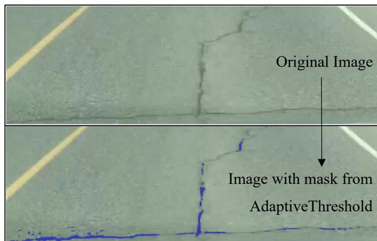
**Figure 35. Mask derived from a contrast-enhance image using `AdaptiveThreshold` function**
