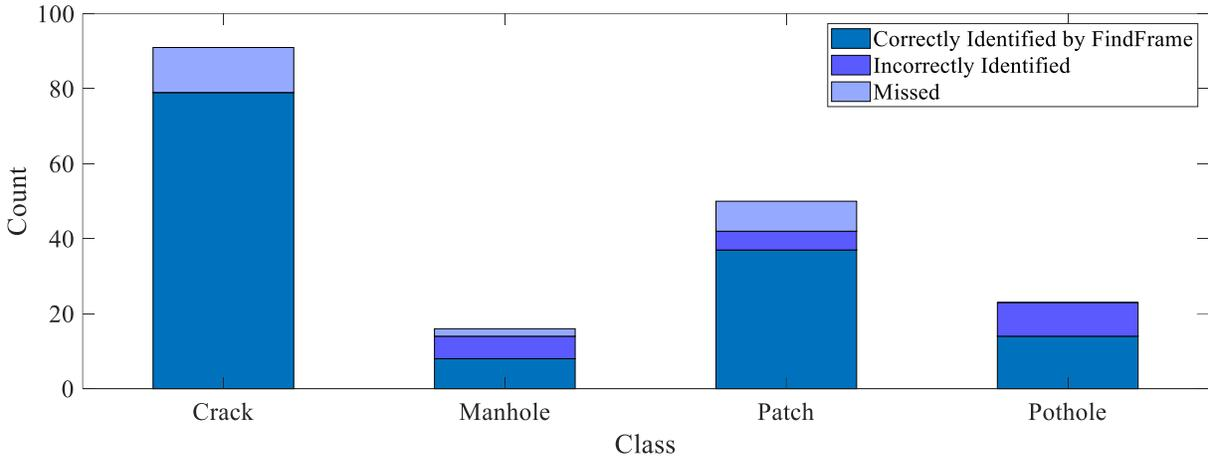
**Figure 64. Defect identification in extracted frames compared to the manual review of the video**
