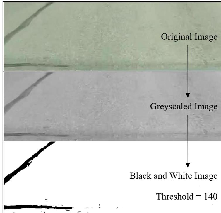
**Figure 30. An example of image segmentation with thresholding.**
