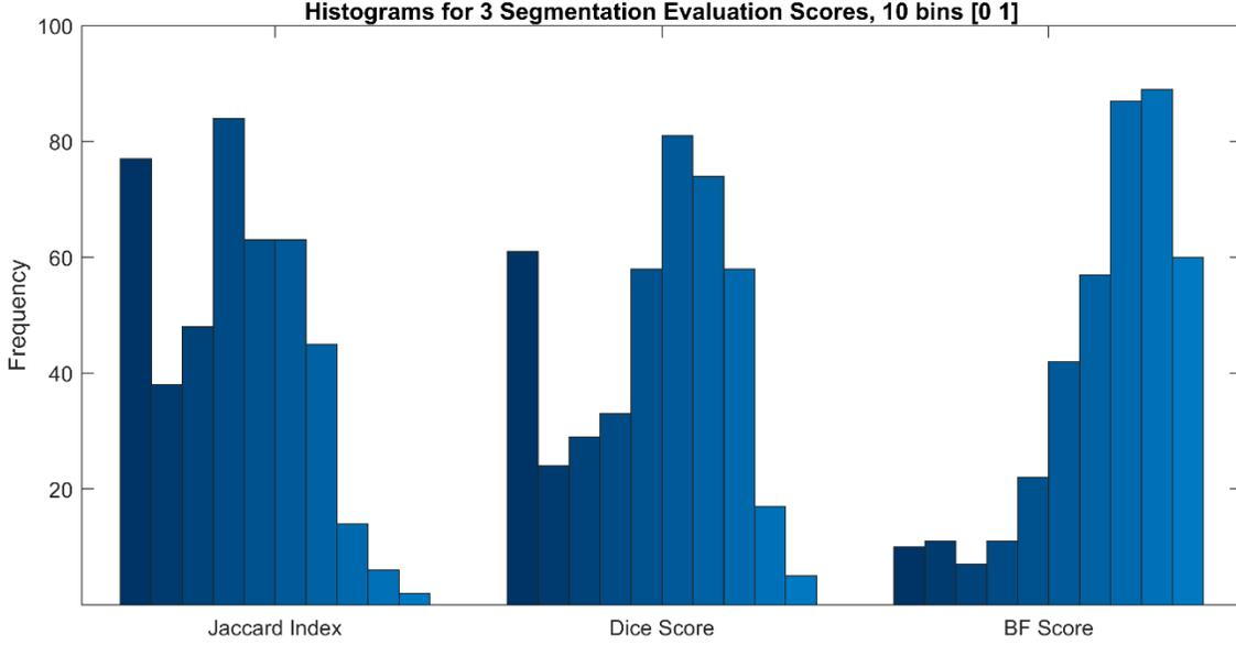
**Figure 55: Comparing scores for the Crack class in the image training set**
