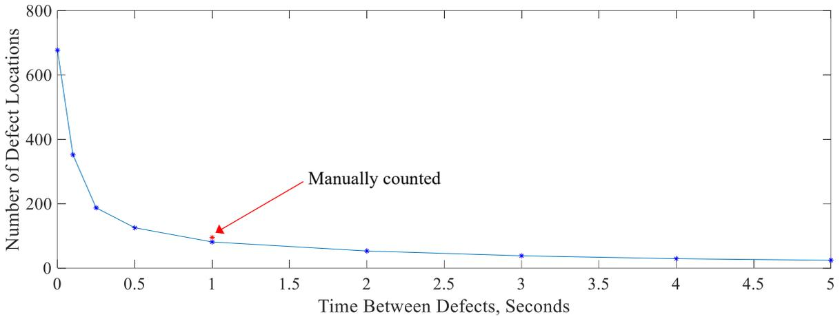
**Figure 63. Defect locations automatically detected based on time between acceleration peaks**
