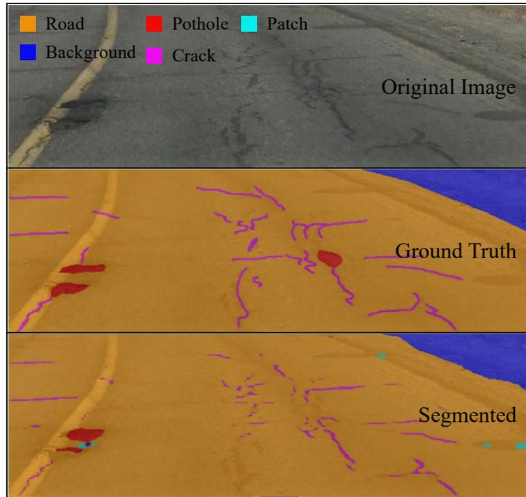
**Figure 58. Example of a segmented image with low BF score**
