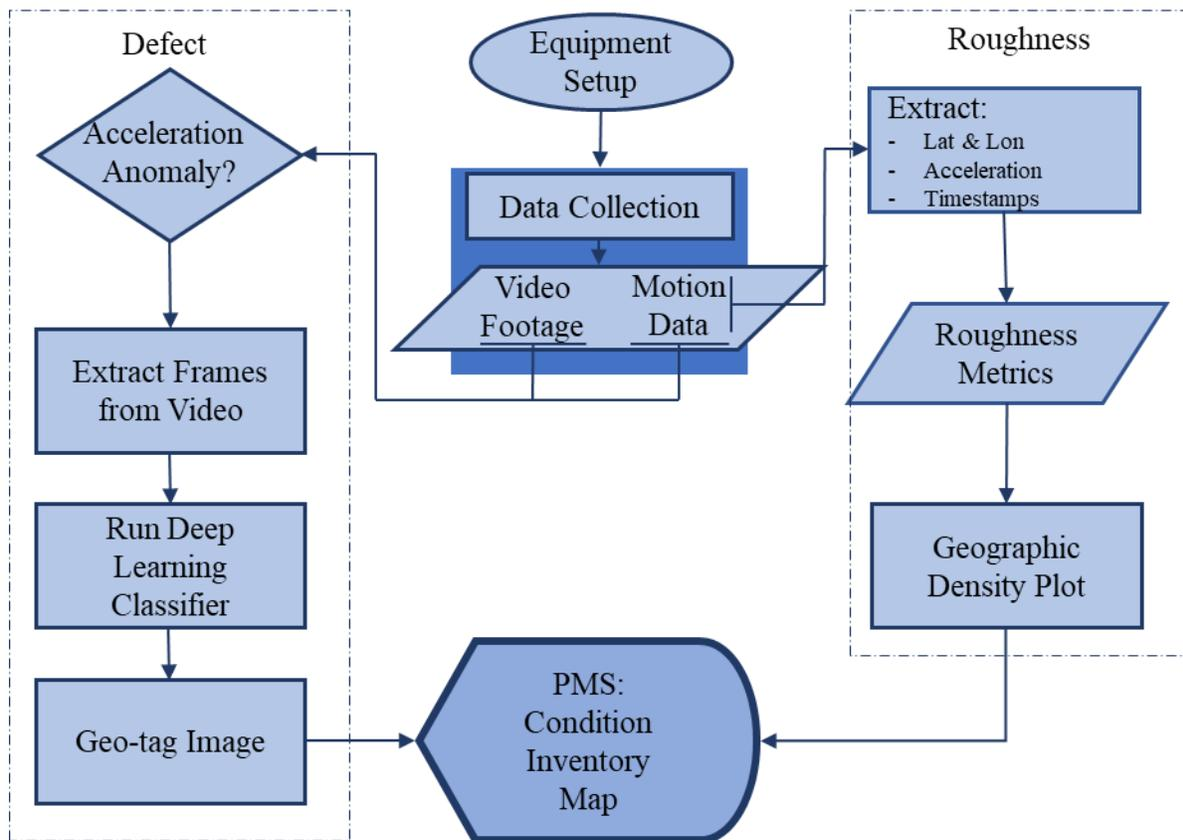
Figure 19. Overview of the pavement condition assessment system, from data collection to display
