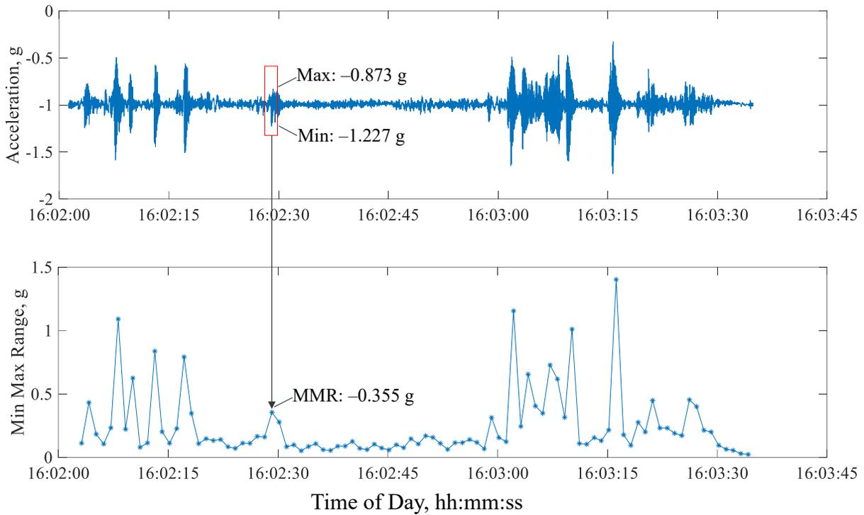
**Figure 25. Original acceleration data (top) condensed to a series of MMR values (bottom).**
