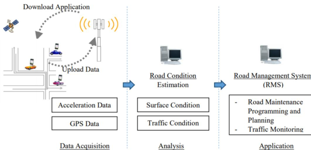
**Figure 11. Acquire, Analyze, Apply—the approach to using smartphone data for a PMS (Douangphachanh and Oneyama 2013b)**
