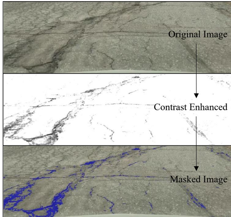
**Figure 53. An example of image segmentation with thresholding**
