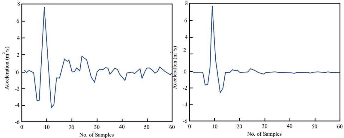
**Figure 13. Acceleration before (left) and after (right) the signal has passed through a maximum absolute value filter (Harikrishnan and Gopi 2017)**
