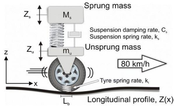
**Figure 8. The quarter car model used in the International Roughness Index (Loizos and Plati 2008)**
