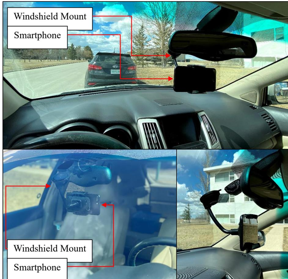
**Figure 20. Equipment setup used for data collection**
