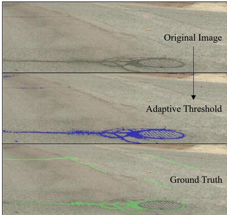
**Figure 51. Comparing an image ground truth and adaptive threshold**
