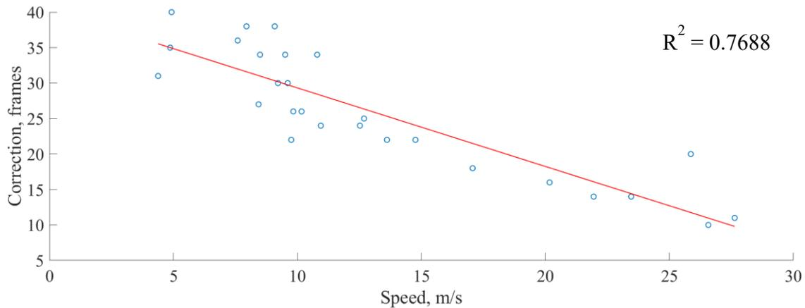
**Figure 41. Values manually collected to determine speed-based correction factor.**
