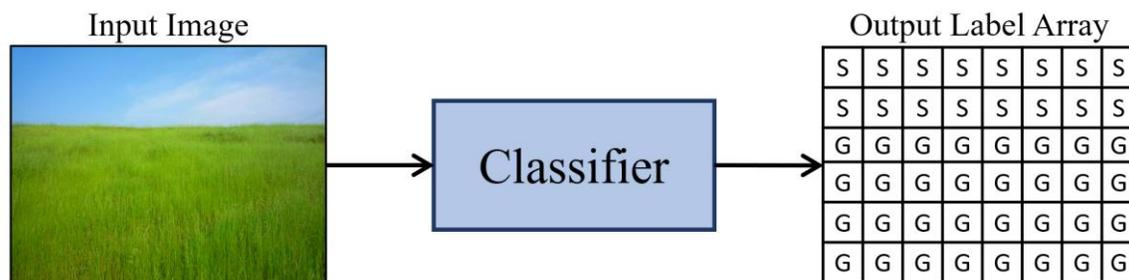
**Figure 37. Basic process of semantic segmentation using a CNN as a classifier**
