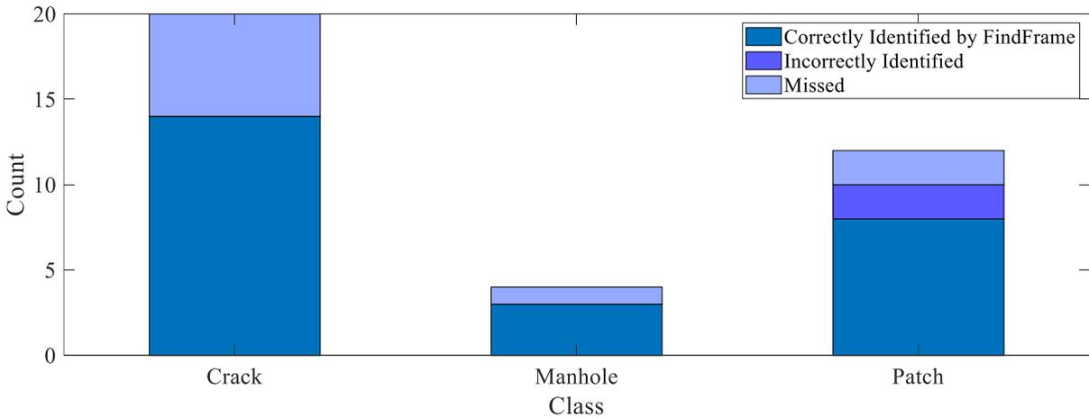
**Figure 61. Combination of defects identified automatically and manually**
