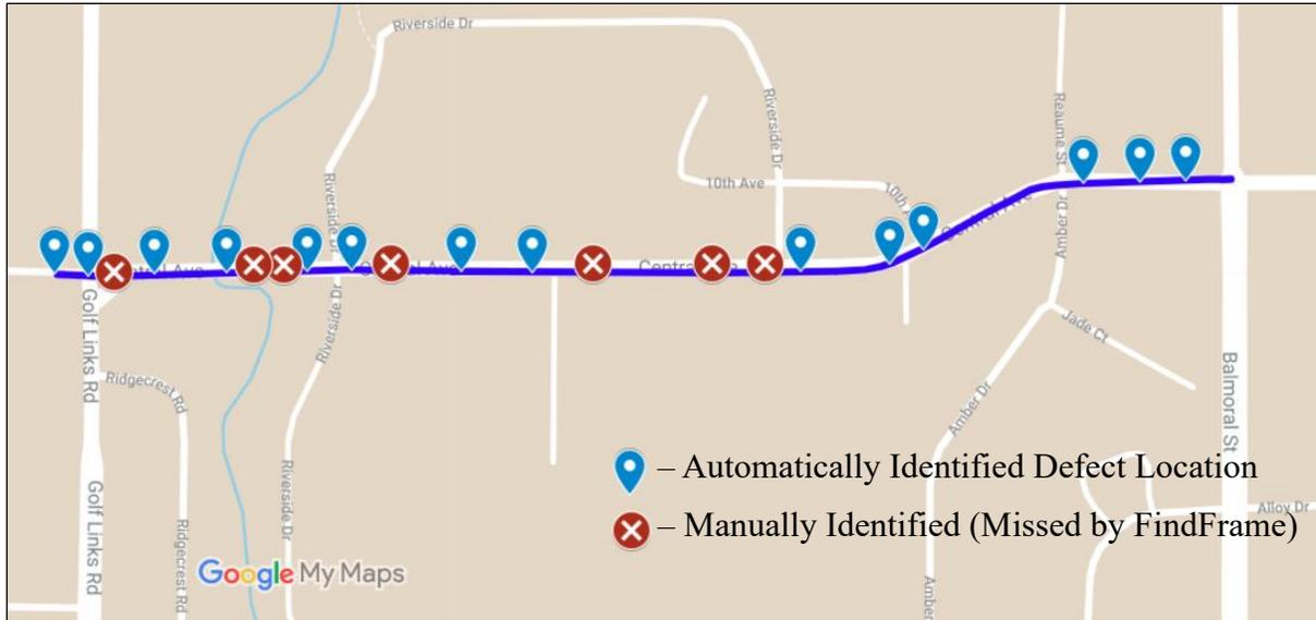
**Figure 60. Automatically and manually identified defect locations along a short route**
