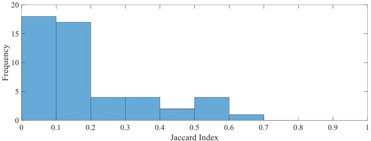
**Figure 52. Histogram of results comparing thresholded image masks to the ground truth labels**
