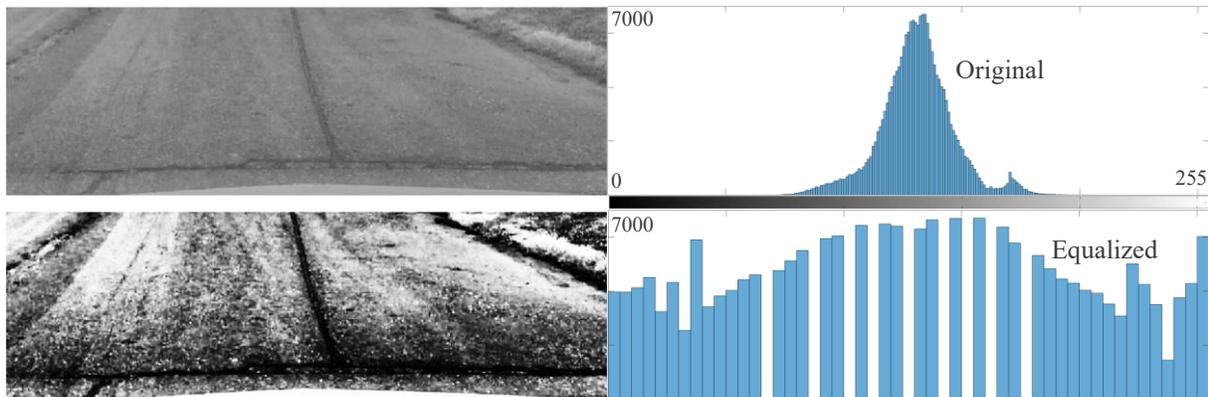
**Figure 33. The original grayscale image, an equalized version, and their histograms**
