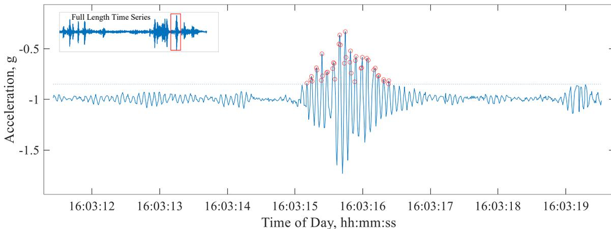
**Figure 28. Closer view of a pothole-induced spike in acceleration.**
