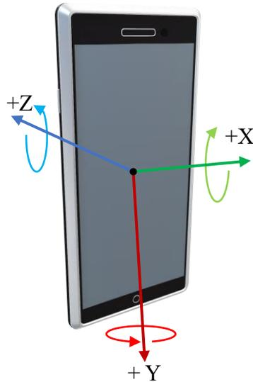
**Figure 21. The six degrees of freedom captured by the phone's motion sensors**
