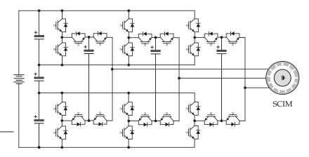
Figure 1.11. Four-level HCC fed MV drive.
