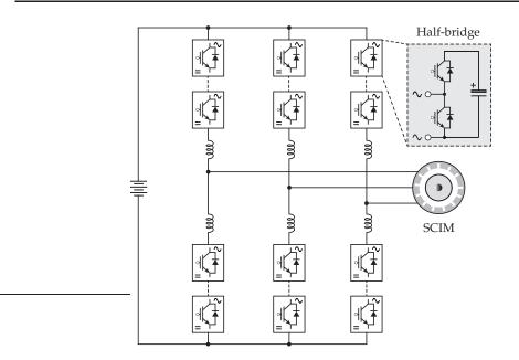
Figure 1.13. Four-level MMC fed MV drive.
