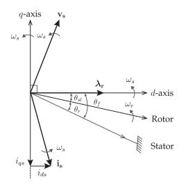
Figure 3.3. Space phasor diagram of field orientation.
