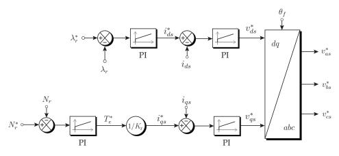
Figure 3.6. Control block diagram of IFOC.
