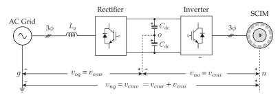
Figure 1.3. Common mode voltage in MV drive.
