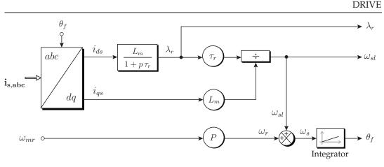
**Figure 3.5.** Estimation of rotor flux magnitude and position ( $\lambda_r$  and  $\theta_f$ ).
