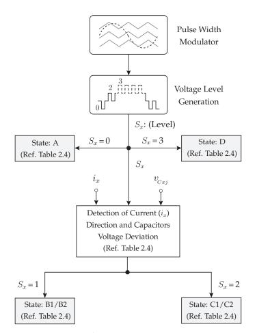
Figure 2.7. Implementation of the proposed voltage balancing approach.
