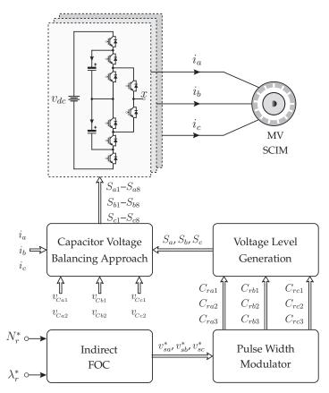
Figure 3.2. Control block diagram of the proposed 4L-MLC fed MV drive.
