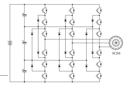
Figure 1.6. Four-level DCC fed MV drive.
