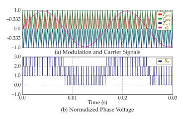
**Figure 2.13.** Representation of modulation and carrier signals in modified carrier PWM.
