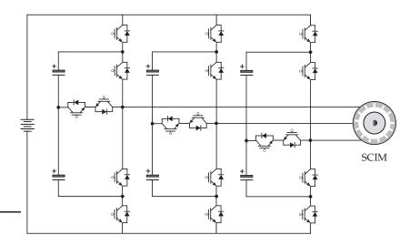
Figure 1.12. Four-level nested T-type converter fed MV drive.
