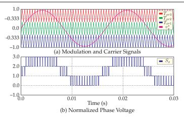
Figure 2.6. Representation of modulation and carrier signals in PD-PWM.
