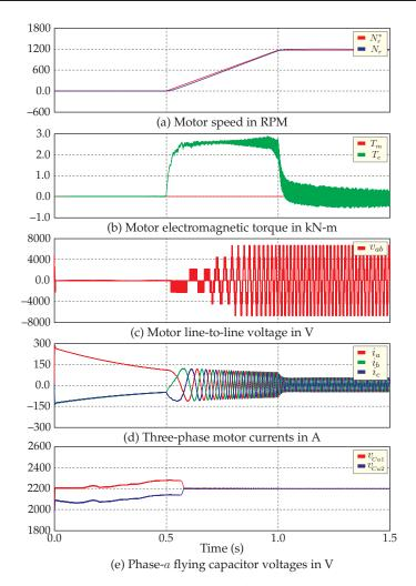
Figure 3.7. Startup performance of the proposed MV drive.
