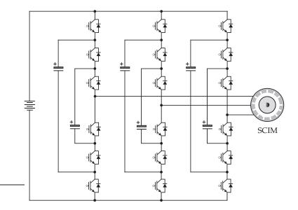
Figure 1.7. Four-level FCC fed MV drive.
