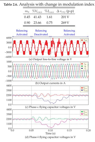
**Figure 2.9.** Step response with and without balancing approach ( $m_a = 0.75$ ,  $f_o = 60$  Hz and PF = 0.80 (lag)).
