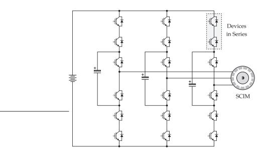
Figure 1.8. Four-level SFCC fed MV drive.
