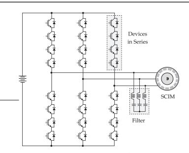
Figure 1.5. Two-level converter fed MV drive.
