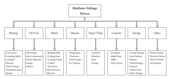
Figure 1.1. Applications of MV drives.
