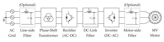
Figure 1.2. Structure of MV drive.
