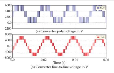
Figure 2.2. Basic operation of 4L-MLC.
