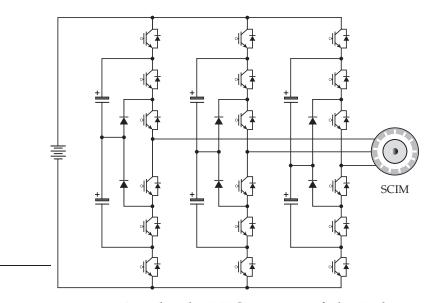
Figure 1.9. Four-level NNPC converter fed MV drive.
