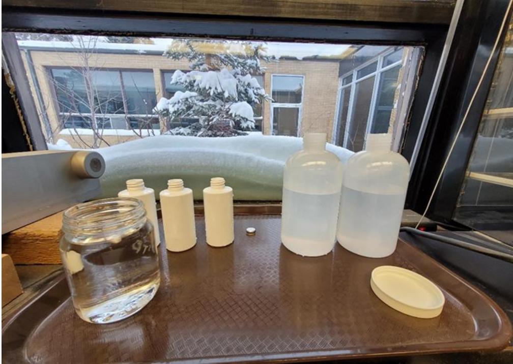
Figure 1: A picture containing Base control (Glass), White container (Bioplastic) and Translucent container (High-density Polyethylene), including replicates
