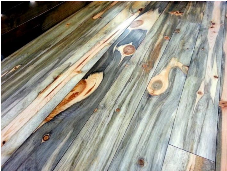
Figure 5 pine beetle damaged veneer wood. (Pinterest, 2022)
