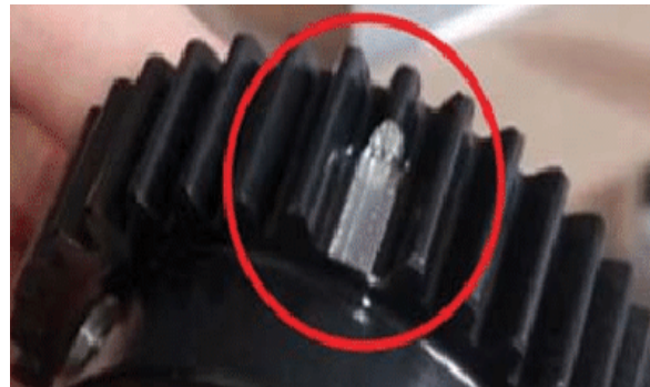
Fig. 1.5 An example of a broken gear tooth defect [23].
