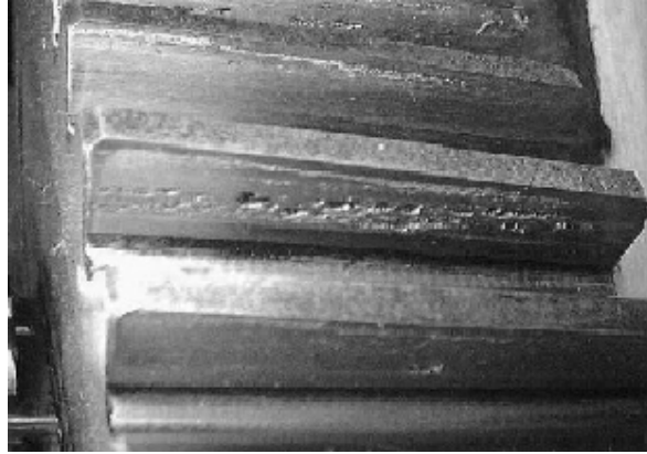
Fig. 1.4 An example of pitting defect in gears [22].
