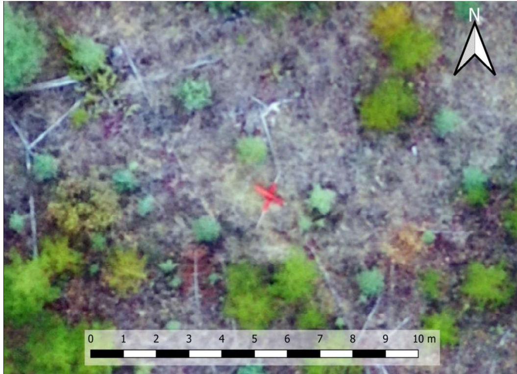
Figure 5. Plot centres marked with spray painted "X". Image captured at 100 m AGL with the Hasselbad L1D-20c camera built in to the DJI Mavic Pro 2, pointed 90° towards the ground.
