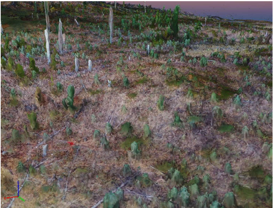
Figure 7. Example of the point cloud mesh produced for Stand A in Pix4D.
