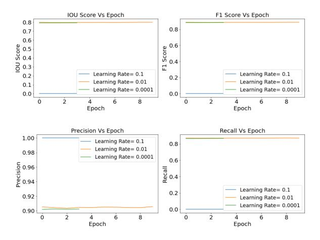
Figure 5.11: Spalling segmentation: U-Net InceptionV3- comparison of the evaluation metrics based on ADAM optimizers and learning rate 0.1, 0.01 and 0.0001
