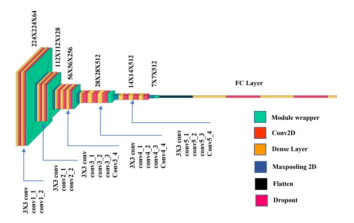
Figure 3.8: CNN base model architecture- VGG-19
