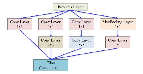
Figure 3.11: CNN base model architecture- Inception
