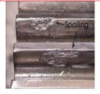
Figure 4.10 (continue): Sample images for spalling prediction using CNN
