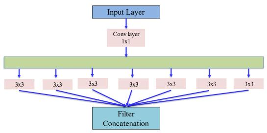
Figure 3.13: CNN base model architecture- Xception
