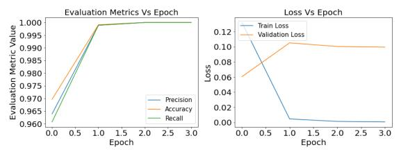
Figure 4.7: Defects classification with InceptionV3: result of the evaluation metrics and model loss for optimizer SGD and learning rate 0.001
