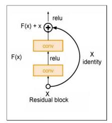
Figure 3.9: CNN base model architecture- ResNet
