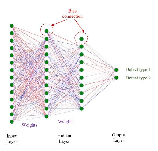
Figure 3.7: Example of a fully connected layer
