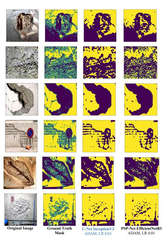
Figure 5.15: Semantic segmentation of spalling detection using best two models
