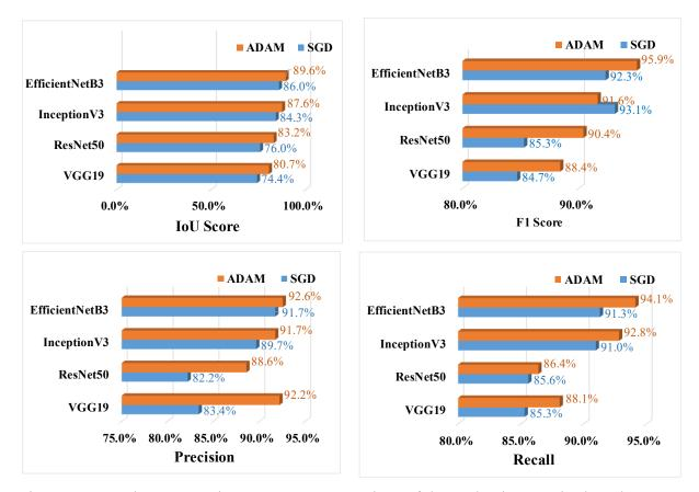
Figure 5.8: Crack segmentation: PSP-Net- comparison of the evaluation metrics based on SGD and ADAM optimizers and learning rate 0.01
