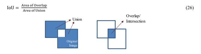
Figure 3.14: Schematic presentation of IoU
