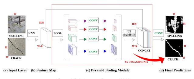
Figure 5.5: Schematic diagram of PSP-net
