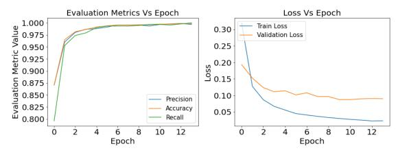
Figure 4.8: Defects classification with InceptionV3: result of the evaluation metrics and model loss for optimizer SGD and learning rate 0.1
