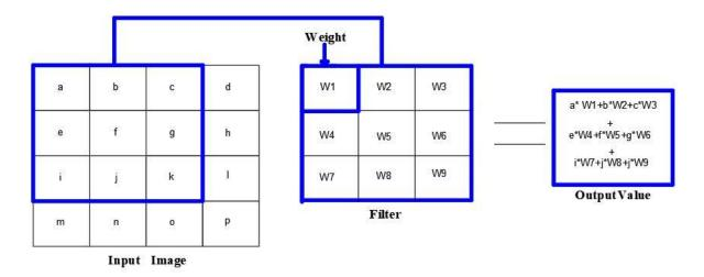
Figure 3.3: Convolutional operation method with 1-D tensor
