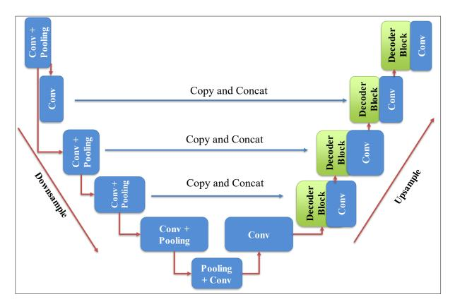
Figure 5.4: Schematic diagram of U-Net architecture
