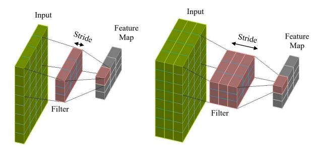
(a) 1-D channel (b) 3-D Channel Figure 3.4: Convolution example- (a) 1-D channel and (b) 3-D channel
