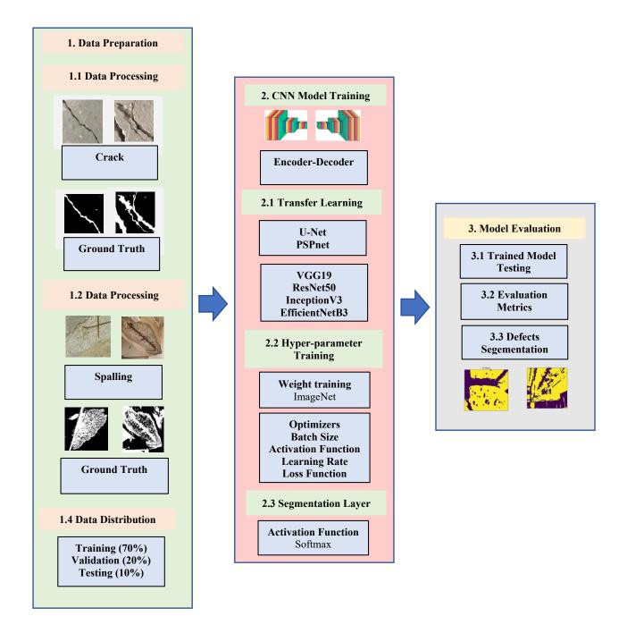
Figure 5.2: Work flow chart for defects segmentation
