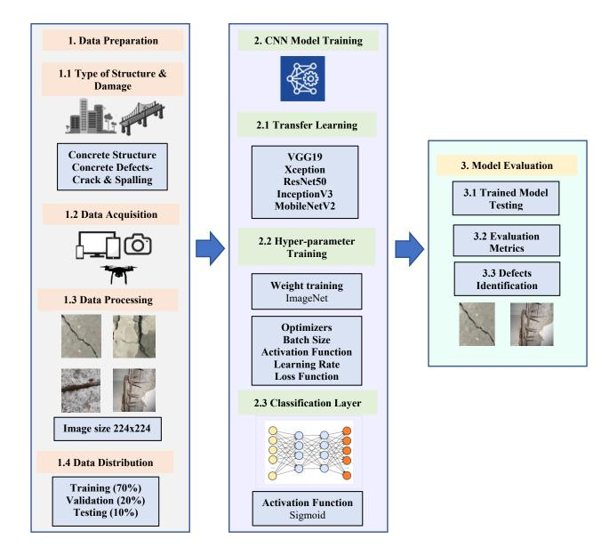
Figure 4.1: Workflow chart for defects classification
