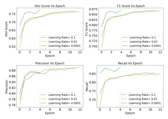
Figure 5.13: Spalling segmentation: **P**SP-Net EfficientNetB3- comparison of the evaluation metrics based on ADAM optimizers and learning rate 0.1, 0.01 and 0.0001
