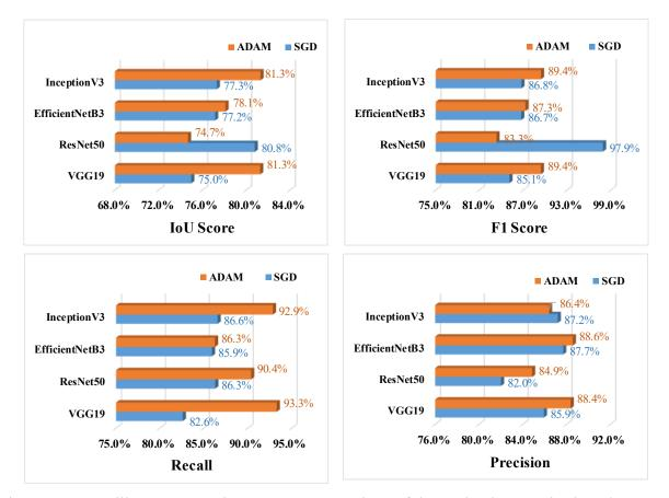
Figure 5.10: Spalling segmentation: U-Net- comparison of the evaluation metrics based on SGD and ADAM optimizers and learning rate 0.01
