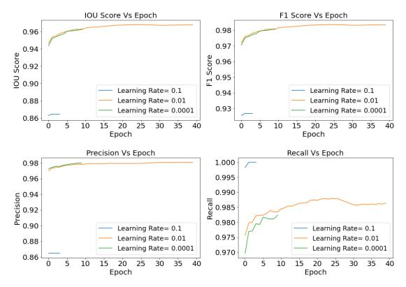
Figure 5.9: Crack segmentation: PSP-Net- comparison of the evaluation metrics based on ADAM optimizers and learning rate 0.1, 0.01 and 0.0001
