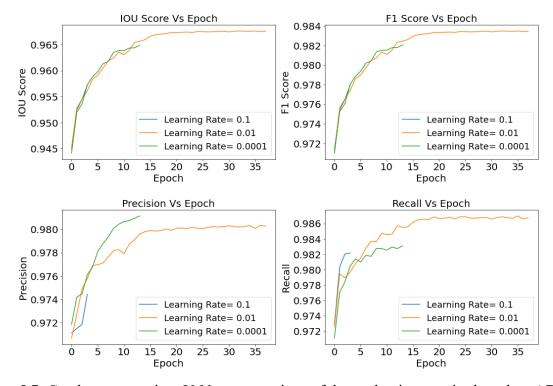
Figure 5.7: Crack segmentation: U-Net- comparison of the evaluation metrics based on ADAM optimizers and learning rate 0.1, 0.01 and 0.0001
