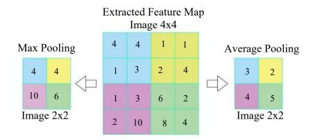
Figure 3.5: Example of max and average pooling
