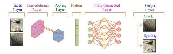
Figure 3.1: schematic diagram of basic CNN architecture
