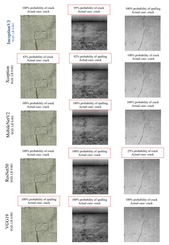
Figure 4.9 (continue): Sample images for crack prediction using CNN models
