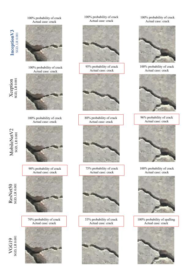
Figure 4.9: Sample images for crack prediction using CNN models
