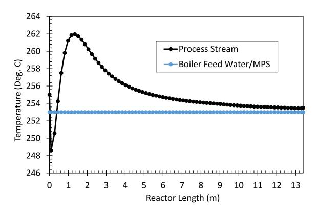
Figure 21. Temperature profiles of the process fluid (tubes) and the saturated steam (shell).
