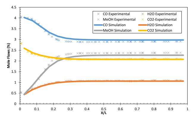
**Figure 17.** Experimental and Aspen Hysys<sup>TM</sup> simulated mole flows along MSR length using the Vanden Bussche & Froment (1996) kinetic model.
