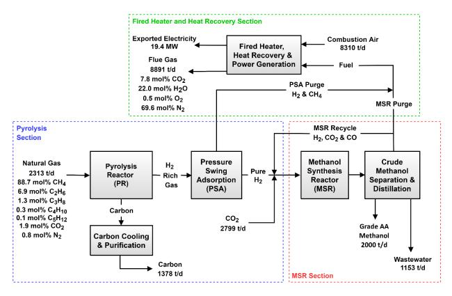
Figure 11. Process block flow diagram.
