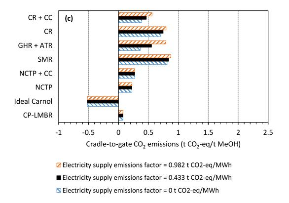
**Figure 26.** Effect of the CO<sub>2</sub> emissions factors for (a) natural gas supply, (b) CO<sub>2</sub> supply, and (c) electricity supply on the cradle-to-gate CO<sub>2</sub> emissions of several natural gas pyrolysis and reforming processes. Data for SMR and GHR + ATR assume maximum electricity imports to emphasize the effect of  $F_{elect.-supply}$  on the emissions of these processes.
