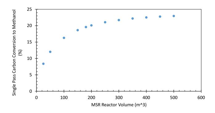
**Figure 20.** Methanol synthesis reactor volume selection under isothermal and isobaric conditions with constant reactor inlet flowrate, composition, temperature (255 °C) and pressure (8000 kPa).
