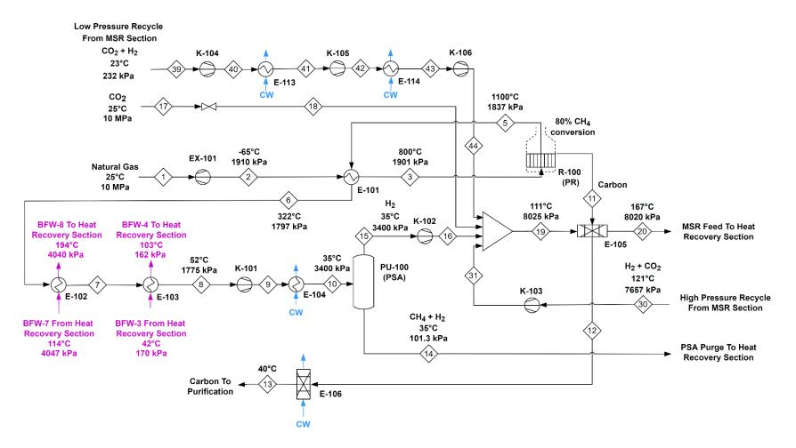
Figure 12. Process flow diagram of the pyrolysis section; E: heat exchanger EX: gas expander, K: compressor, PU: PSA unit, R: reactor.
