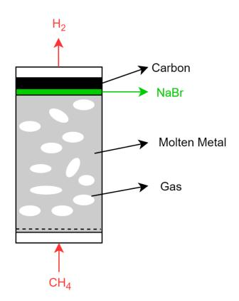
Figure 4. Simplified schematic of liquid metal bath reactor for methane pyrolysis.
