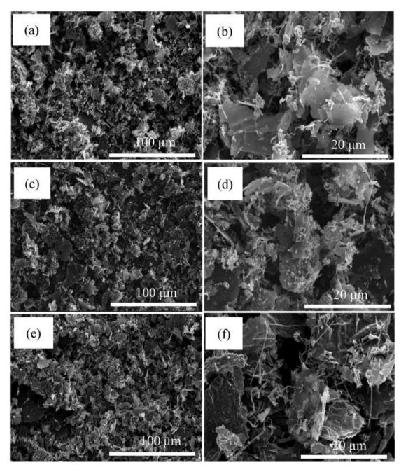
**Figure 9.** SEM micrographs of carbon samples obtained from 1000 °C (a) & (b) NiBi/KBr (110 mm/240 mm), (c) & (d) NiBi/KBr (240 mm/110 mm) & (e) & (f) NiBi/NaBr (110 mm/240 mm) two phase bubble column reactors (Rahimi et al., 2019).
