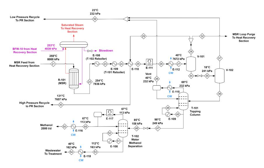
Figure 13. Process flow diagram of the MSR section; E: heat exchanger, R: reactor, T: tower, and V: vessel.
