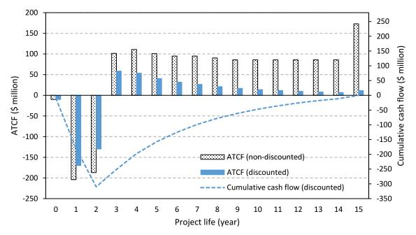
**Figure 27.** Discounted and non-discounted cash flow diagram when the cost of carbon is set to its levelized value of \$0.270/kg.
