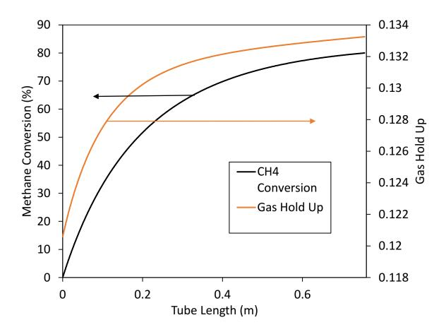
**Figure 15.** Pyrolysis reactor methane conversion and gas hold up profiles along the length of a single PR tube. Dimensions and operating conditions are those found in Table 1.
