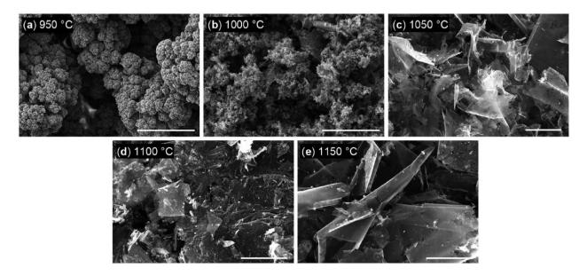
**Figure 7.** SEM micrographs of carbon obtained from 0.18 m KCl bubble column at different temperatures: (a) 950 °C, (b) 1000 °C, (c) 1050 °C, (d) 1100 °C & (e) 1150 °C. All carbons have been washed in 70 °C water for two hours with constant stirring. Scale bars in all images are 50  $\mu$ m (C. Palmer et al., 2021).
