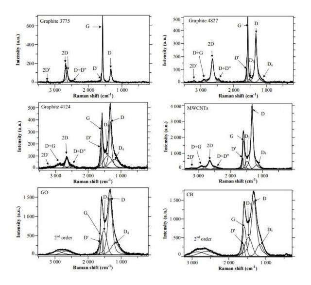
**Figure 5.** Raman spectra of carbon-based materials excited at 633 nm (Bokobza et al., 2015). Graphite grades 3775, 4827 & 4124, multiwalled carbon nanotubes (MWCNTs), graphene oxide (GO) and carbon black (CB).
