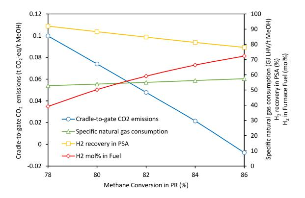
**Figure 24.** Effect of pyrolysis reactor methane conversion on cradle-to-gate emissions, natural gas consumption, PSA H<sub>2</sub> recovery and fuel H<sub>2</sub> mol%.
