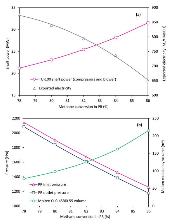
**Figure 25.** Effect of methane conversion in the PR on TU-100 shaft power, exported electricity, molten metal alloy and inlet and outlet pressures.
