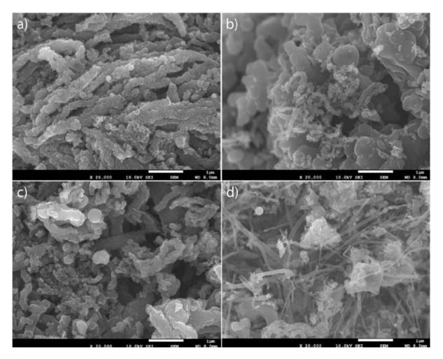
**Figure 6.** SEM micrographs of carbon obtained from 0.1 m (a) 100 wt% Sn, (b) 95 wt% Sn – 5 wt% Cu, (c) 95 wt% Sn – 5 wt% Ni & (d) 70 wt% Sn – 30 wt% Cu (Zaghloul et al., 2021).
