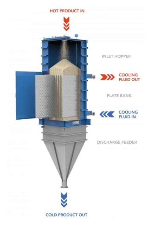
**Figure 23.** Schematic of Solex plate heat exchanger for cooling solid particles (*Cooling Heat Exchanger - Cool Bulk Solids Without Air | Solex - Solex*, n.d.).
