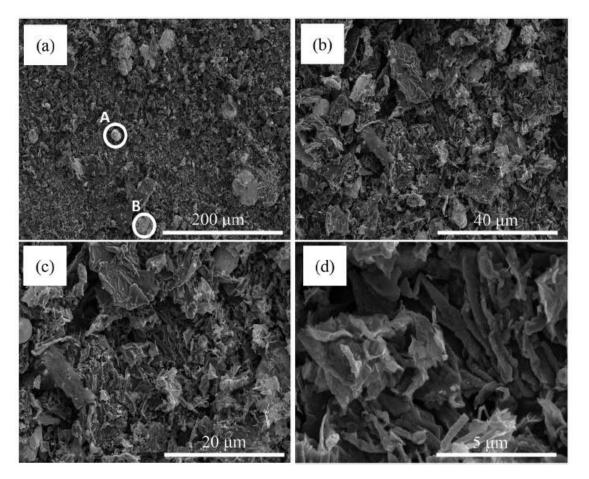
**Figure 8.** SEM micrographs of carbon samples obtained in 1000 °C NiBi (350 mm) single phase bubble column reactor at different magnifications. A & B indicate the presence of metal particles (Rahimi et al., 2019).
