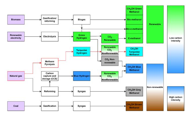
Figure 1. Methanol production Routes
