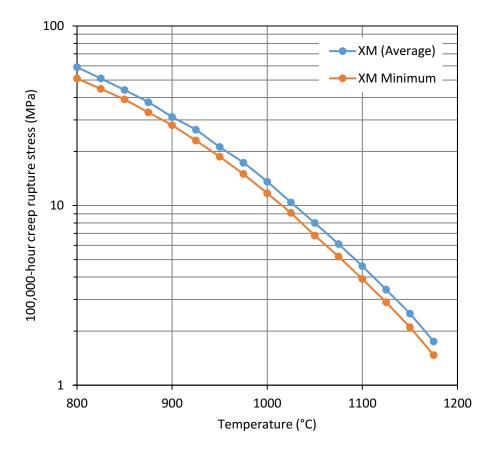
Figure 16. 100,000-h creep rupture stress versus temperature for Manaurite XM.
