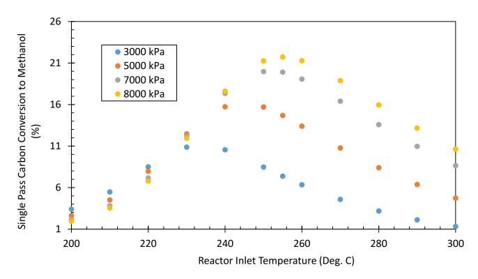
**Figure 19.** Methanol synthesis reactor inlet temperature and pressure selection with constant reactor volume (300 m<sup>3</sup>), inlet flow rate and feed composition under isothermal and isobaric conditions.
