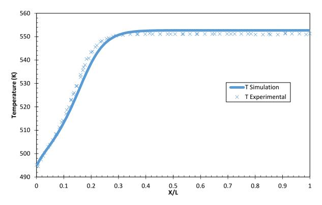
**Figure 18.** MSR reactor temperature profile simulated in Aspen Hysys<sup>™</sup> using the Vanden Bussche and Froment (1996) kinetic model.
