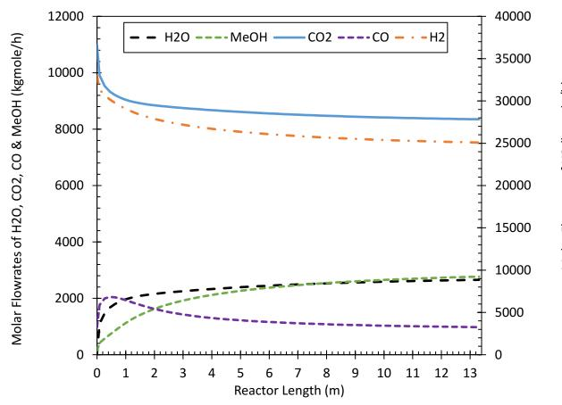
Figure 22. Molar flow profiles along the tubes of the MSR.
