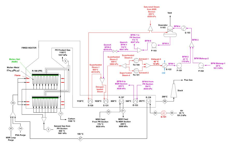
**Figure 14.** Process flow diagram of the fired heater and heat recovery section; B: blower, E: heat exchanger, P: pump, R: reactor, TU: steam turbine.
