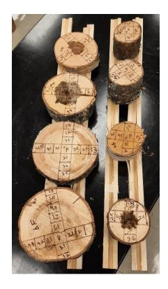
Figure 4 - Wood samples labeled 1" from pith to bark.
