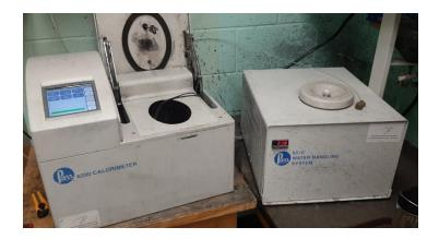
Figure 3 - Bomb calorimeter
