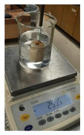
Figure 6 - Water displacement method
