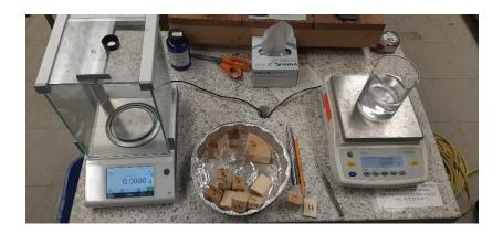
Figure 2 - Wood density instruments
