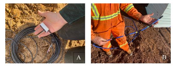
Figure 4. (A) TEROS 10 soil moisture sensor, and (B) five 44007RC Precision Epoxy NTC thermistors arranged in a single cable (or thermistor stack)..
