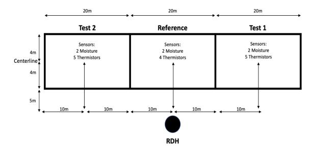
Figure 2. Plan view of the Mawn Road test site.
