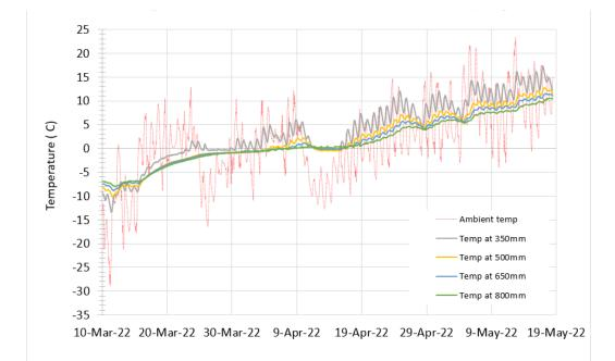
Figure 1. Roadbed thawing in insulated SK resource road during spring 2022.
