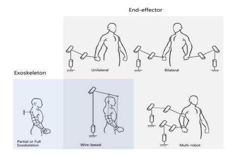
*Note:* Two main categories of upper-limb rehabilitation robots (Sheng et al., 2016).
