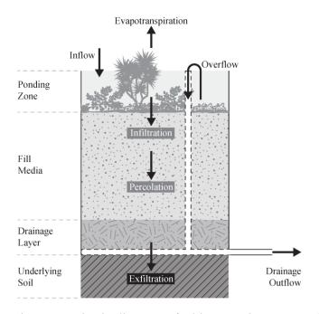
Figure 9. A basic diagram of a bio-retention system (De-Ville et al., 2021).
