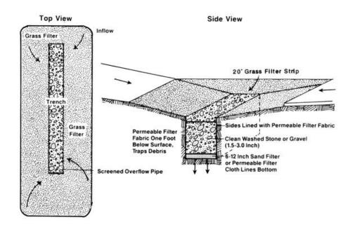
Figure 10. A basic diagram of an infiltration trench (Schueler, 1987).
