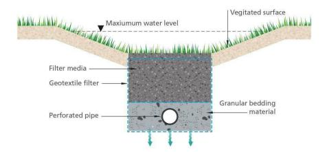
Figure 12. Diagram of an enhanced swale system (PolyPipe, 2023).
