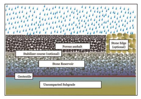
Figure 11. Diagram of a porous asphalt system (Dylla & Hansen, 2015).
