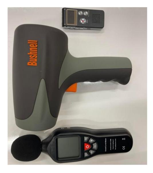
Figure A6: Some of the electronic equipment tried for data collection. The voice recorder is at the top of the page, the speed radar gun is in the middle, and the decibel meter is at the bottom
