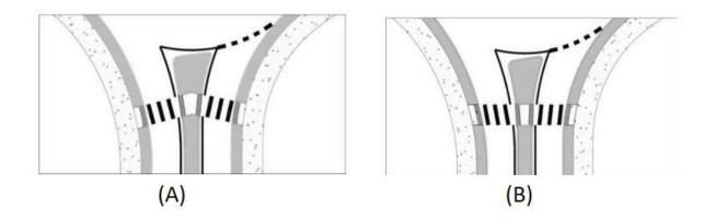
Figure 7: Type (A) is perpendicular crosswalk alignment. Type (B) is flat crosswalk alignment [11]
