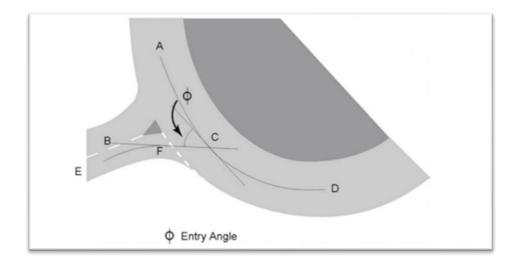
Figure 6: Showing Vehicle Entry Angle Phi (φ) [11]
