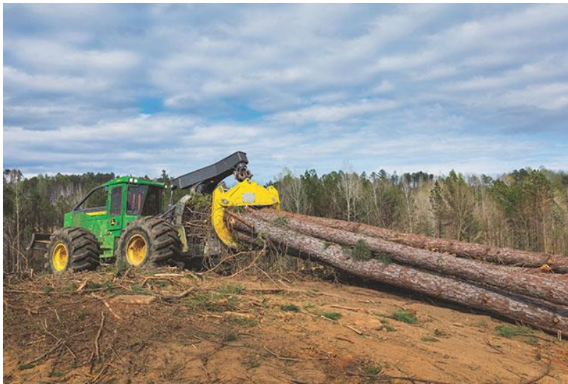
Figure 5. A grapple skidder moving wood (Canadian Forest Industries 2020).
