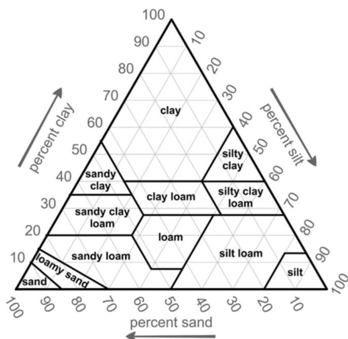
Figure 3. The soil textural triangle of that describes textures by class for mineral soils (Plant and Soil Sciences eLibrary).
