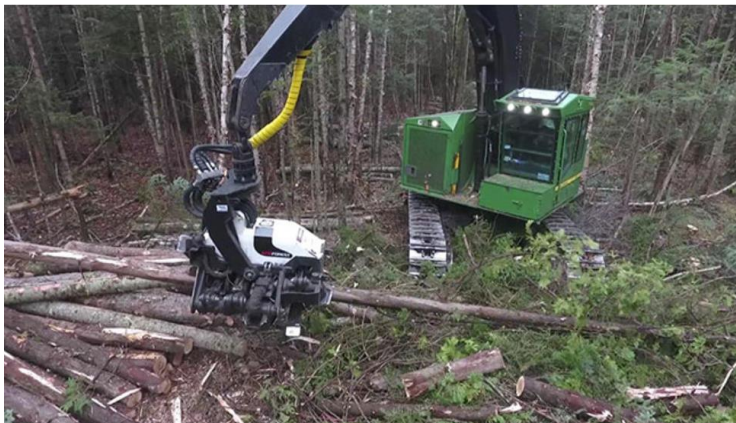
Figure 2. Single grip harvester in action (Canadian Forest Industries 2017).
