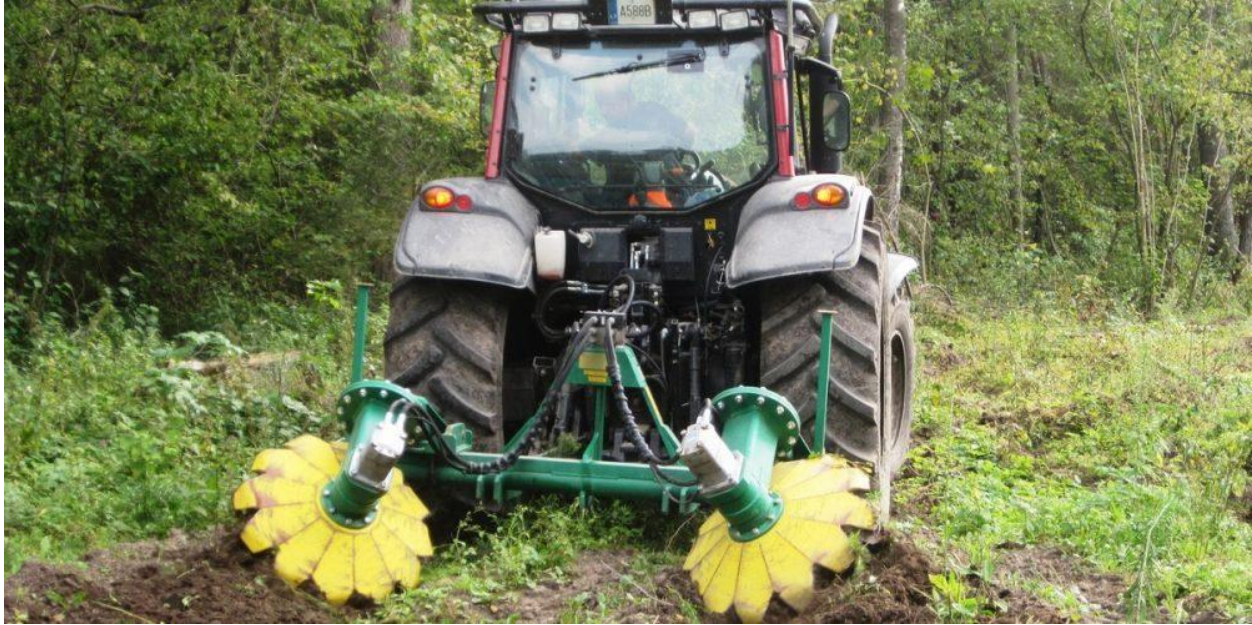
Figure 7. A disc trencher disturbing soil, exposing valuable minerals at a cost of quicker consumption (Mendel University 2020).
