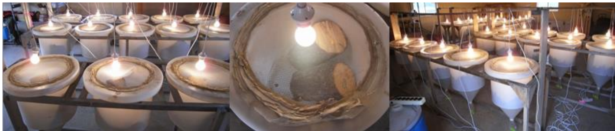
Figure 3. Berlese funnels used for the saproxylic beetle collection at the Mercer Peace River warehouse in Peace River, Alberta. Beetle collection from the early and advanced decay class is seen in the left two images and the right image, respectively.
