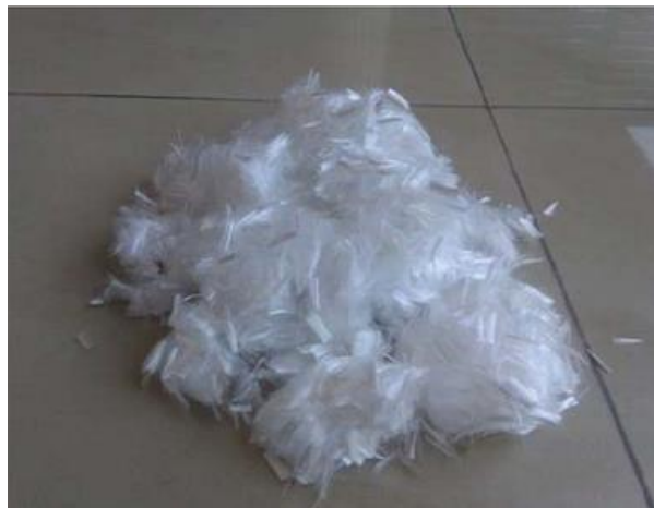
Figure 3.1. Polypropylene fiber (PP) with 13mm length.
