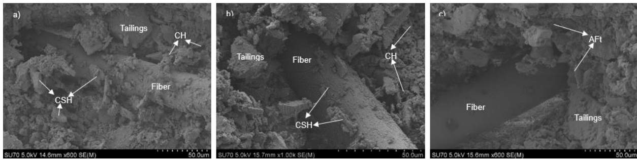
Figure 4.12. SEM images of FR-CPB at three curing times: (a) 7 days, (b) 28 days, and (c) 90 days.
