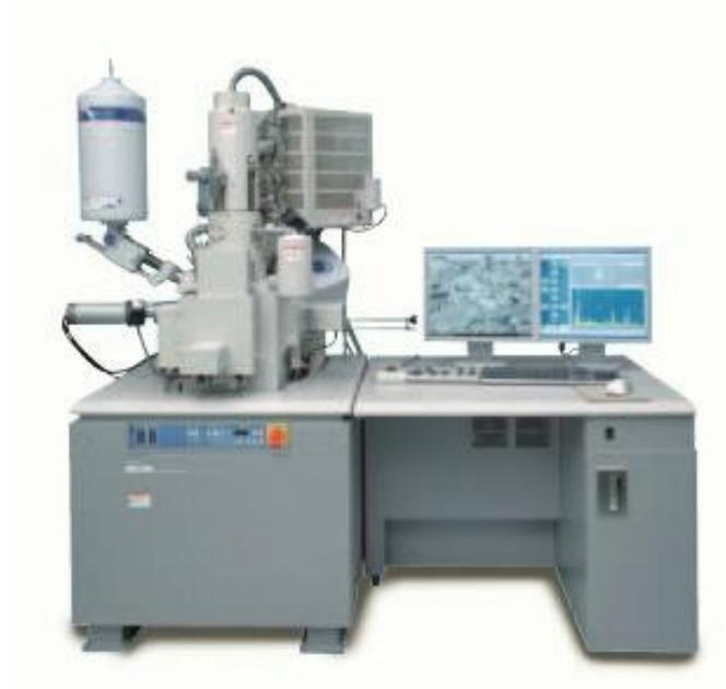
Figure 3.2 The Hitachi SU-70 SEM as shown in the Hitachi commercial brochure.
