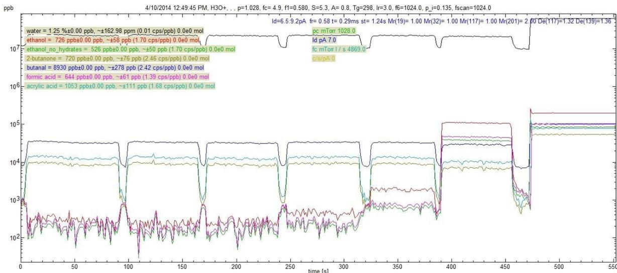
**Figure 6.** Example of MIM mode for detection of ethanol using  $H_3O^+$  precursor ion. The plateaus represent calculated average concentrations (in ppb) of various (colour coded in the software) product ions.
