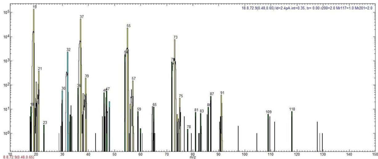
**Figure 5.** Example of water full scans of mass/charge ratio ( $m/z$ ) against frequency of counts produced by SIFT-MS software.
