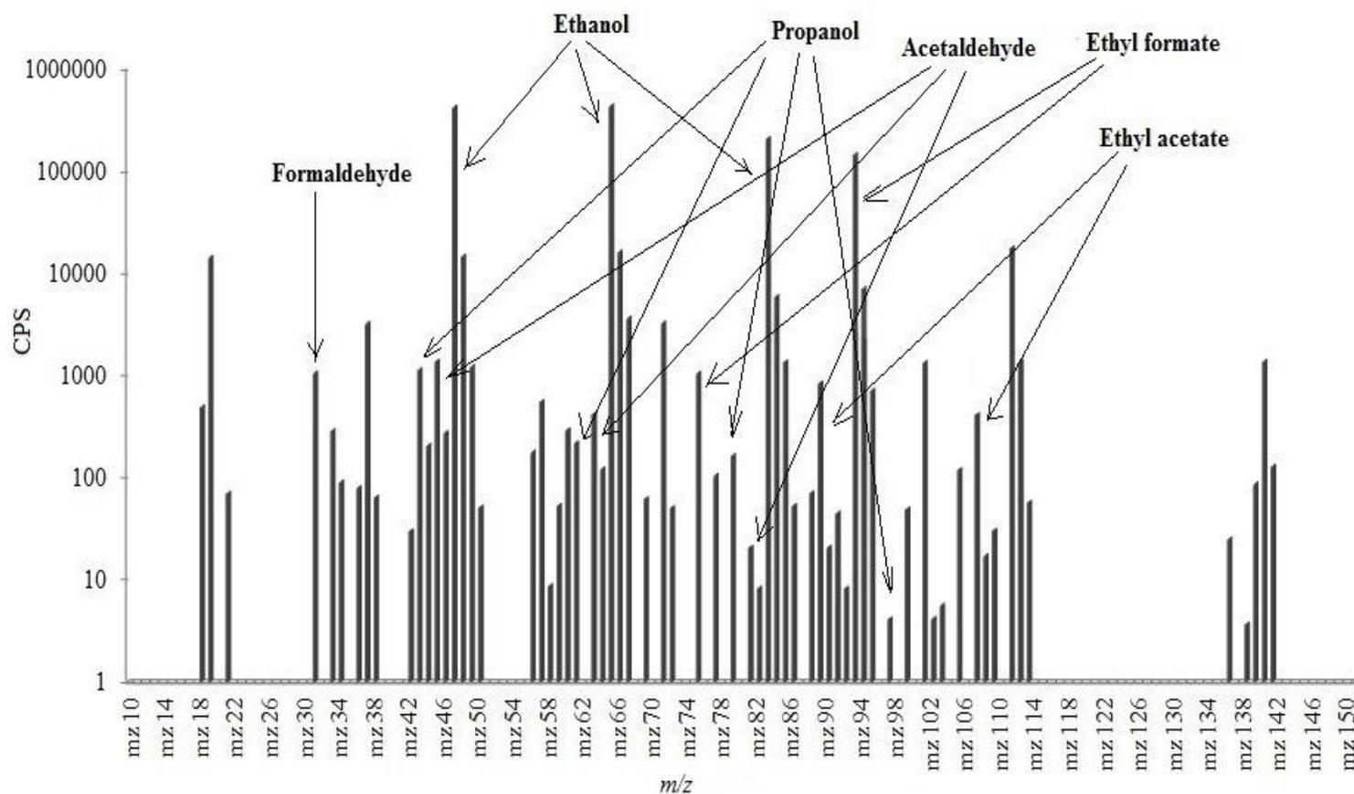
**Figure 13.** Analysis of gas headspace for beer by SIFT-MS. The spectra were generated using  $\text{H}_3\text{O}^+$  precursor ions showing the mean of 3 measurements. Ions produced from blank (water) sample were subtracted from this data. Product  $m/z$  values for common compounds in beer ethanol, propanol, ethyl acetate are indicated.
