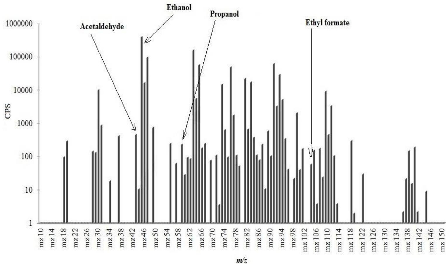
**Figure 14.** Headspace gas SIFT-MS spectra analysis of beer using  $\text{NO}^+$  precursor ions. The mean measurements of 3 samples is shown. Ions produced from blank (water) sample were subtracted from this data. Product  $m/z$  values for common compounds in beer as conformation of the compounds ethanol, propanol and ethyl acetate are indicated.
