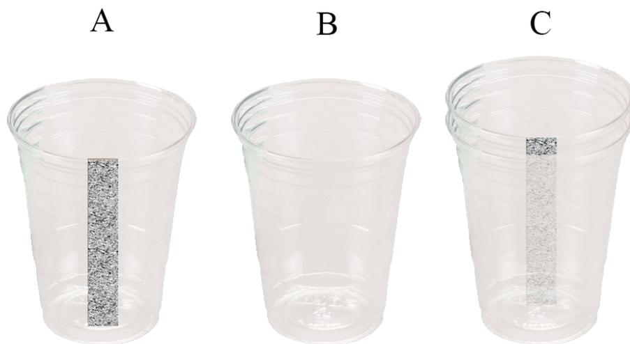
Figure 3. Modified test vessel for chronic exposure testing with invertebrates. A) The inner cup with a 1 cm by 5 cm strip of 200 micron mesh affixed by aquarium silica B) The outer cup holds both the inner cup and test solution C) Both components of the test vessel as used during the chronic experiments.
